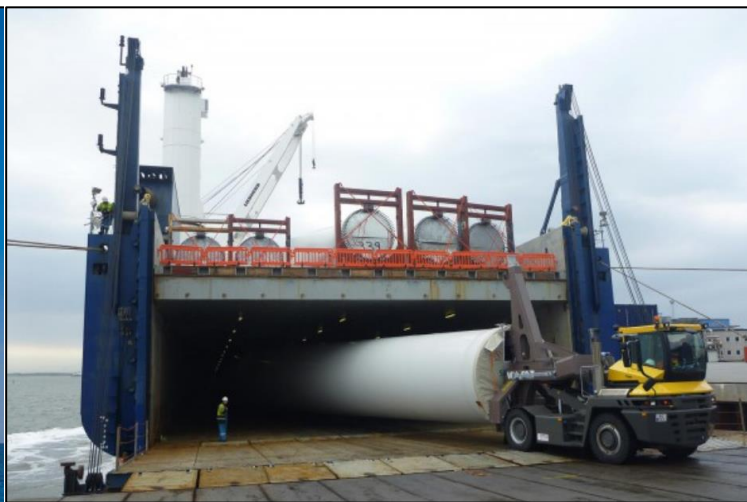
Figure 3.4-5. Ro/Ro capable vessel Source: Roll Group ( www.roll-group.com/projects/windmill-equipment.html ) as cited in BOEM (2016)
