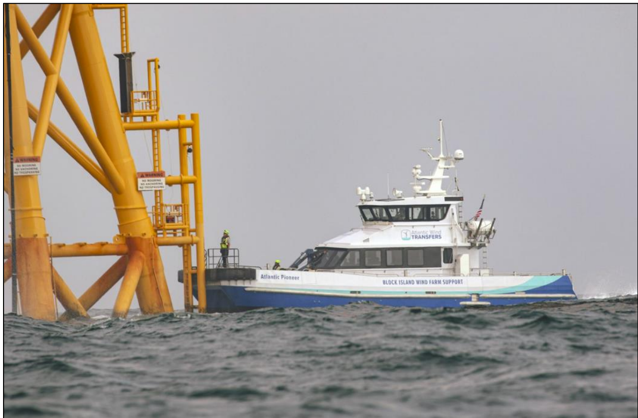
Figure 3.2-1. Crew transfer vessel
