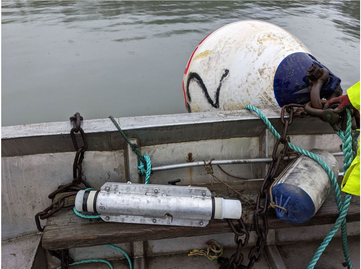
Figure 13: Welded bracket housing F-POD attached to commercial fishing mooring buoy.
