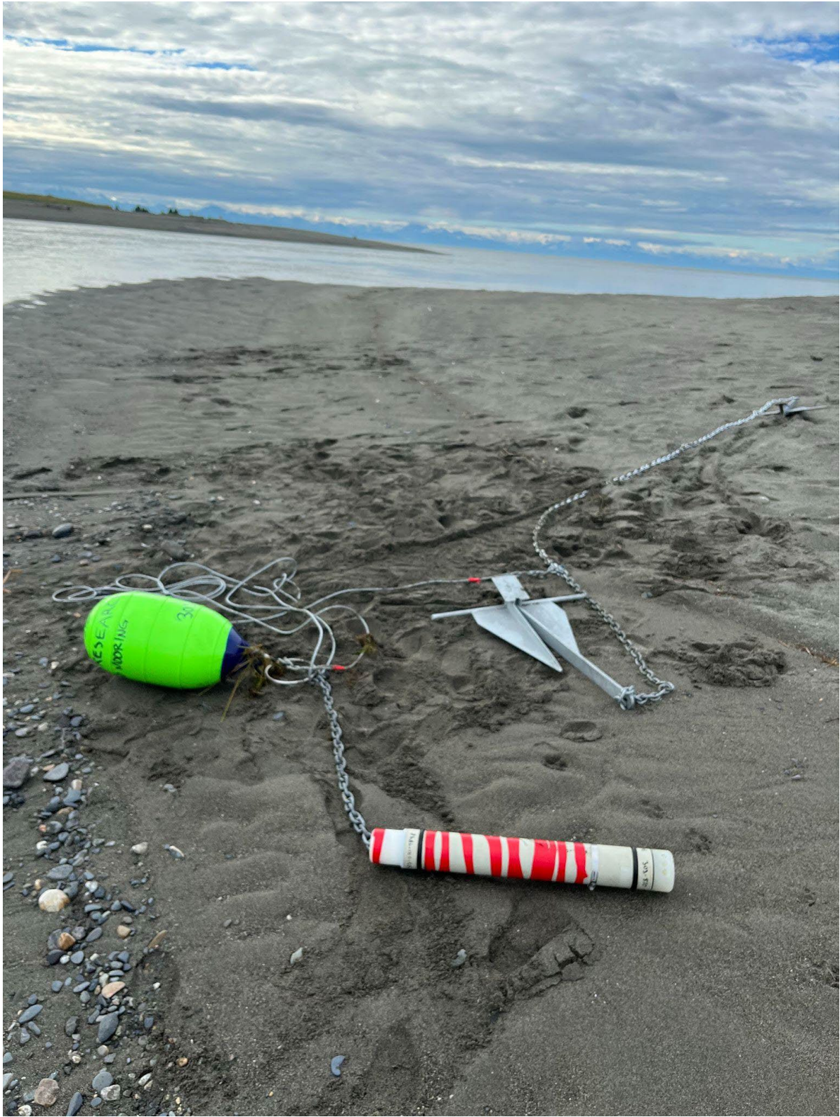
Figure 14: Kasilof River standard deployment configuration.
