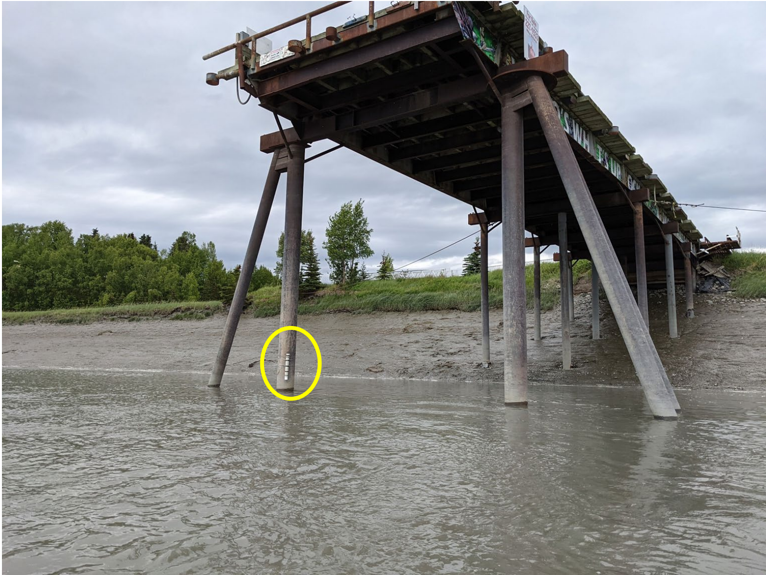
Figure 20: Hose clamp F-POD deployment on the Vasko Dock in the Kasilof River, June 2021
