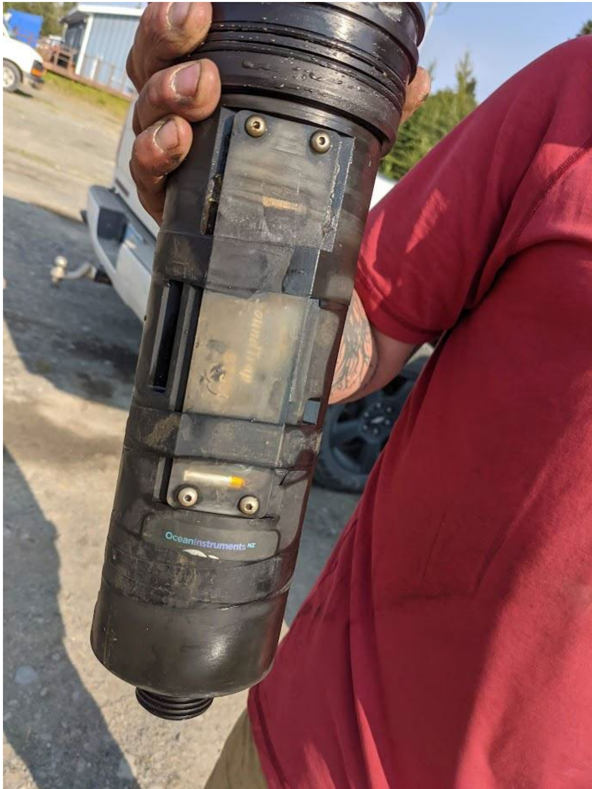
Figure 18: Damaged ST500 from the Kenai River floating dock deployment, August 2021.
