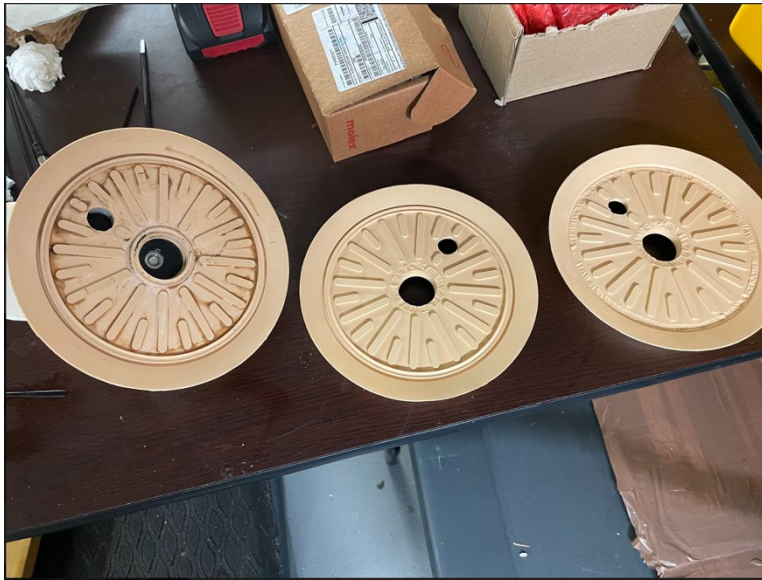
Figure 17. Vacuum cup varieties: (L to R) intact, inner ring removed, inner and outer ring removed.
