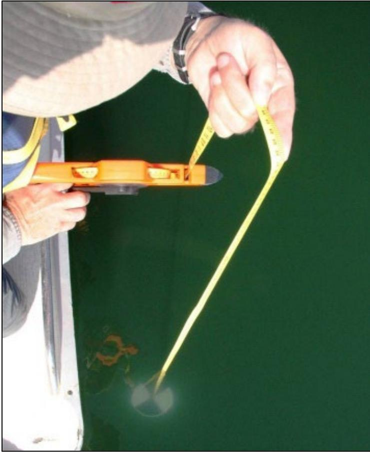
**Figure 12. Measuring water clarity with Secchi disk.**
