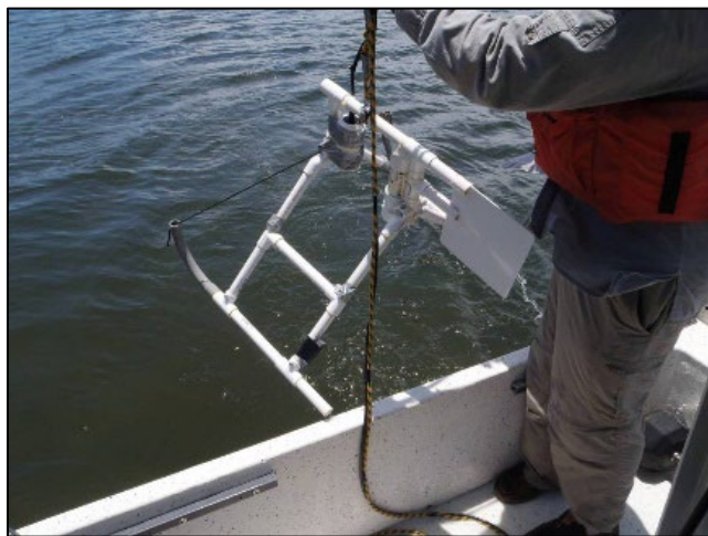
Figure 10. Sled with camera and depth logger, compensated for height above substrate.
