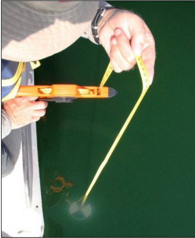
Figure 12. Measuring water clarity with Secchi disk.
