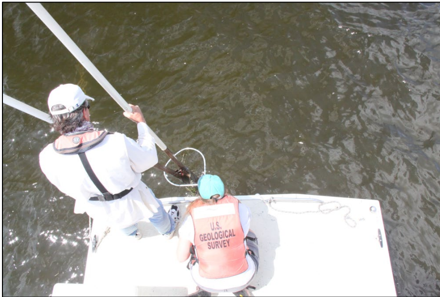
Figure 13. Directed sampling of benthic vegetation with post-hole diggers.
