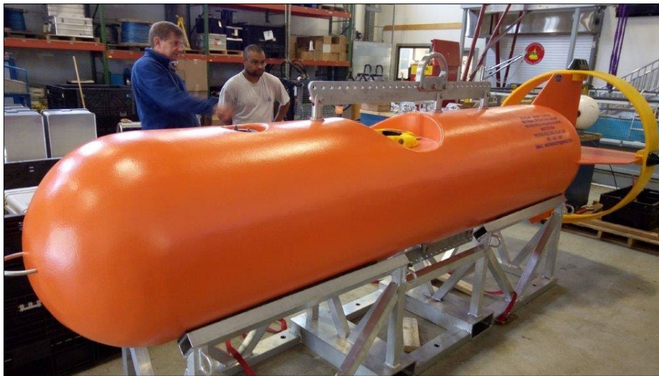
Photo C-12. StableMoor® buoy for the Canyon SHRU VLA.
