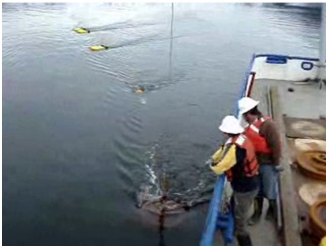
Figure A-14. Typical Subsurface-Mooring System Deployment
