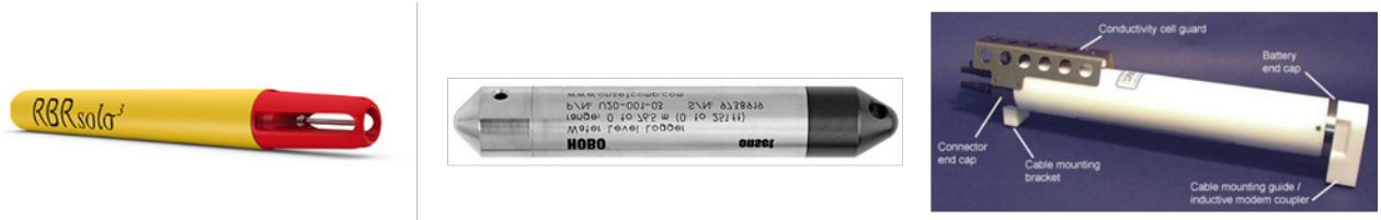
Figure A-11. Thermistor (RBR Solo) Pressure Sensor (Onset Titanium HOB0), and CTD (SBE16plus v2)
