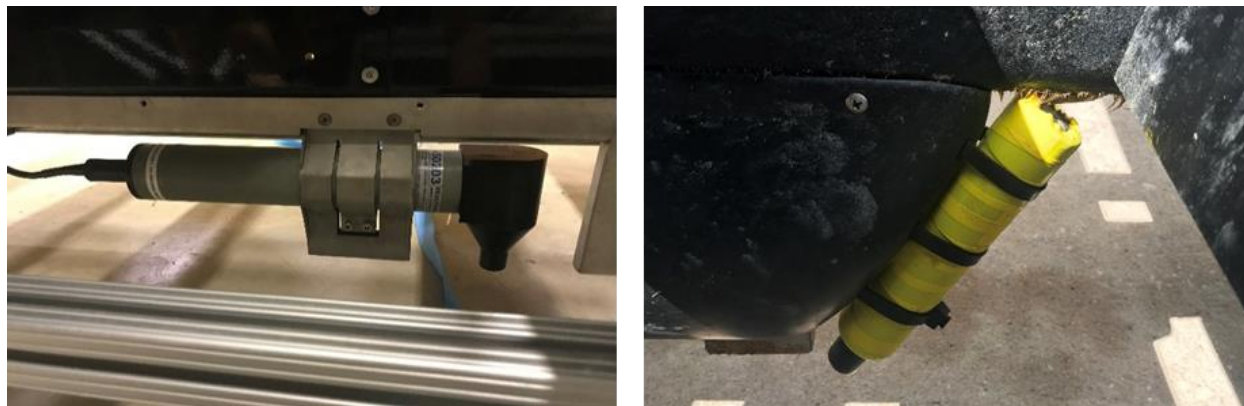
Figure 8. Acoustic receivers mounted to the Wave Glider
