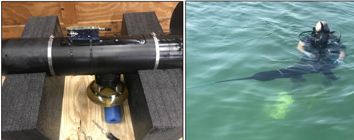
Figure 24. Wave Glider passive acoustic recorders
