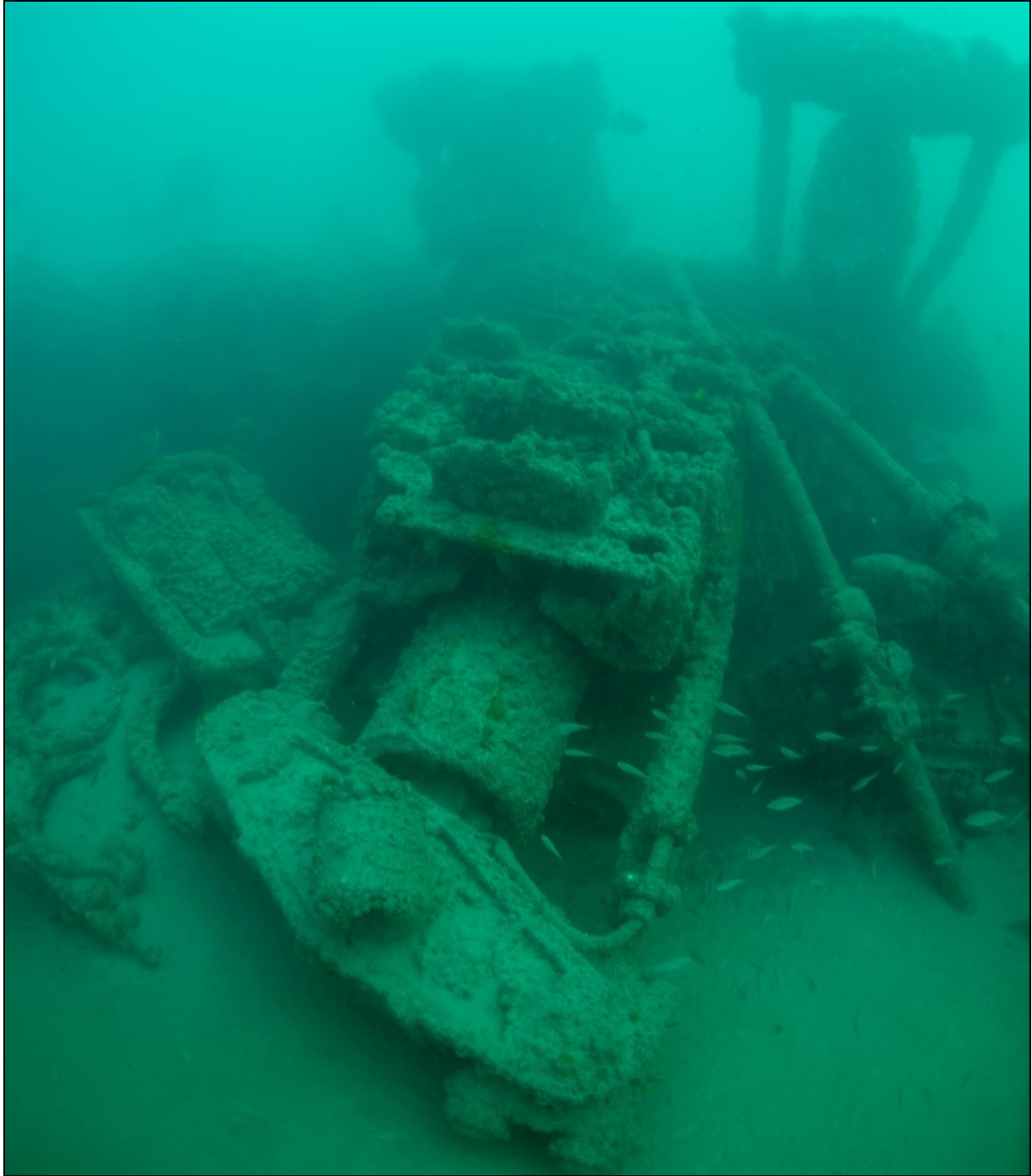
Figure 7-39 Cylinder Diesel Engine piston and connecting rods located at the stern of Australia . Source: NOAA
