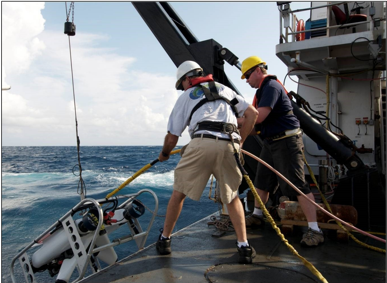
Figure 4-5 University of North Carolina at Wilmington (UNCW) and NOAA personnel deploy an ROV from the deck of R/V Nancy Foster .
