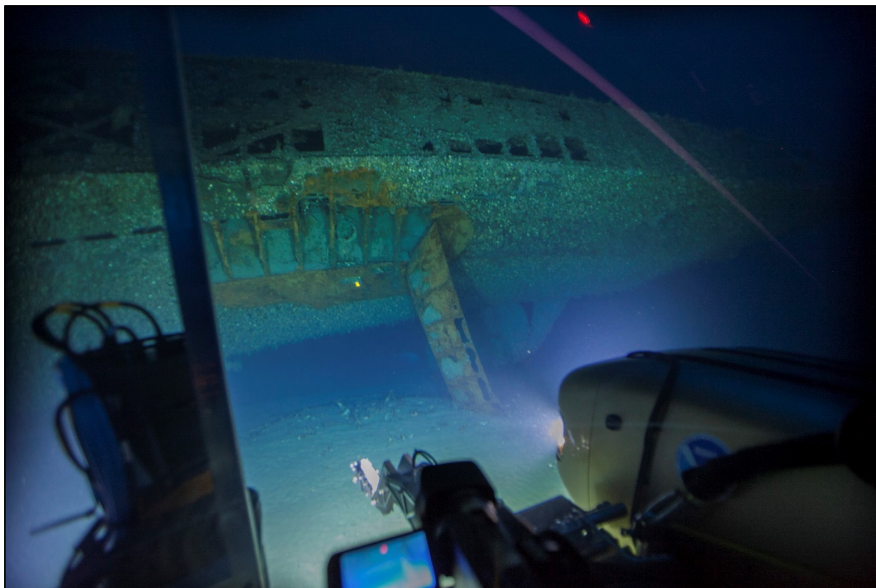
Figure 9-57 Area of damage to the outer hull fairing on the starboard side bow area.
