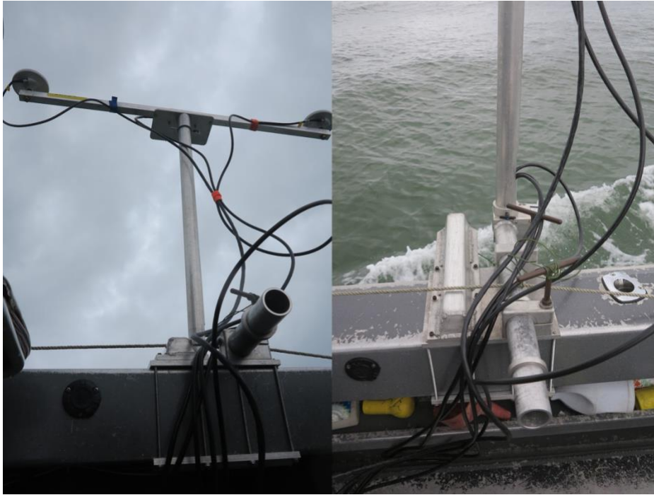
Figure 34 Left: GNSS antennae and IMU mounted on a pole on the starboard gunwale of the F/V Quest. Right.: gunwale adapter.
