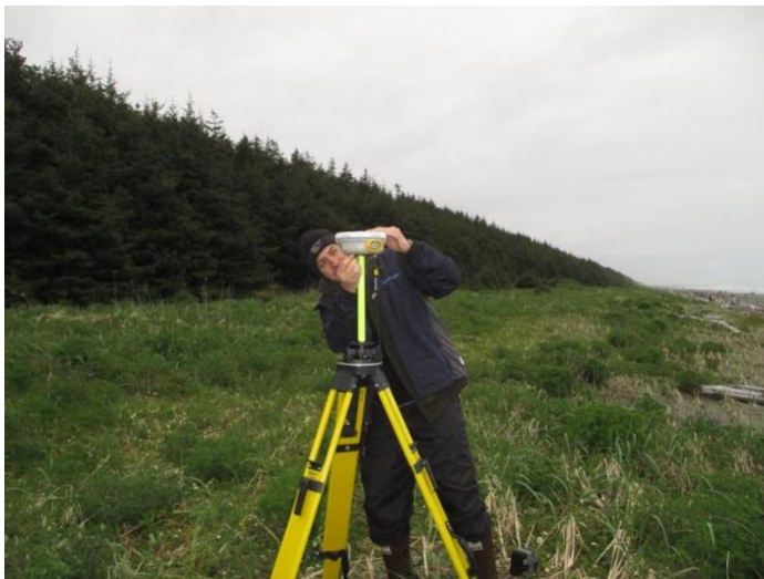
Figure 37. Setting up the Trimble R8 base station broadcasting real time kinematic corrections to the F/V Quest for the multibeam survey.
