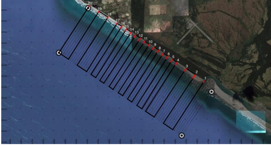
Figure 42. Beach elevation transects occupied in 2018 and 2014 in red using GNSS surveying techniques.
