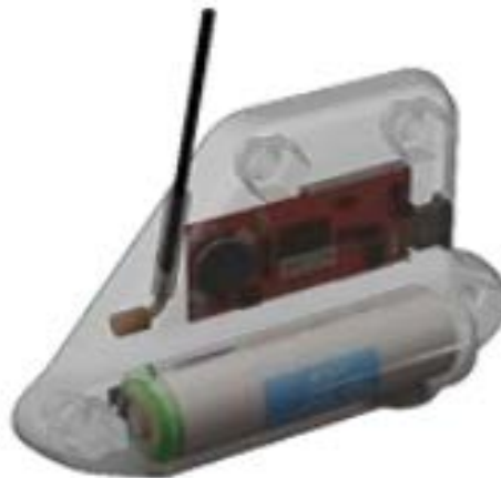
Figure 5. Wildlife Computers fin-mounted satellite SPOT/SPLASH tag.
