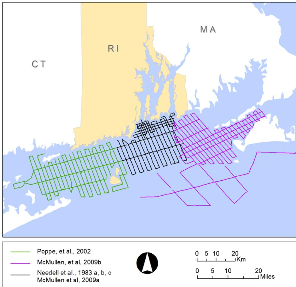
**Figure 4-2. USGS seismic reflection profile tracklines surveyed between 1975 and 1981.**
