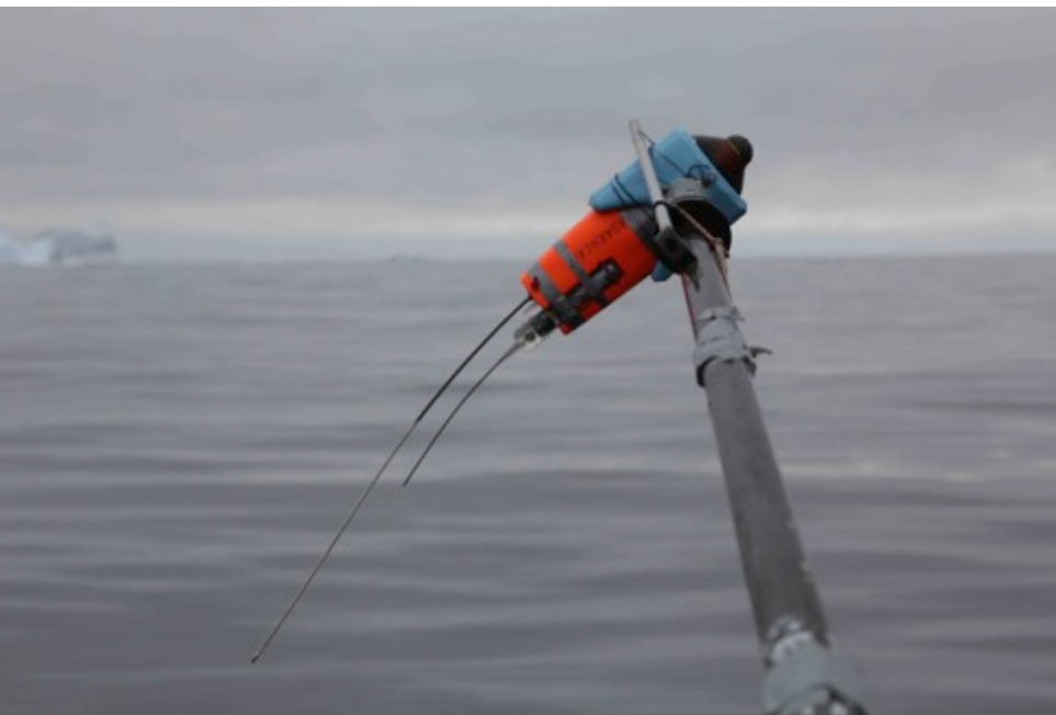
Figure 11. Low-quality picture of the Acousonde secured with yarn around the blue grip.
