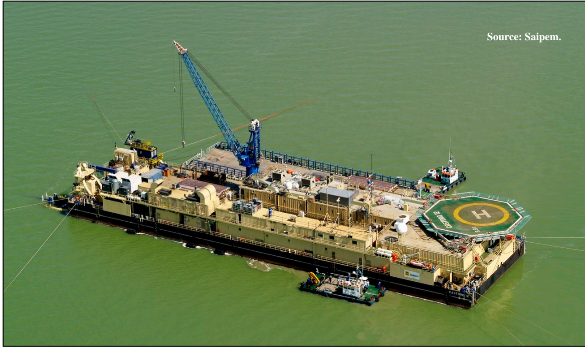
Figure F.7. Castoro 12 , a shallow water low-spec lay barge.
