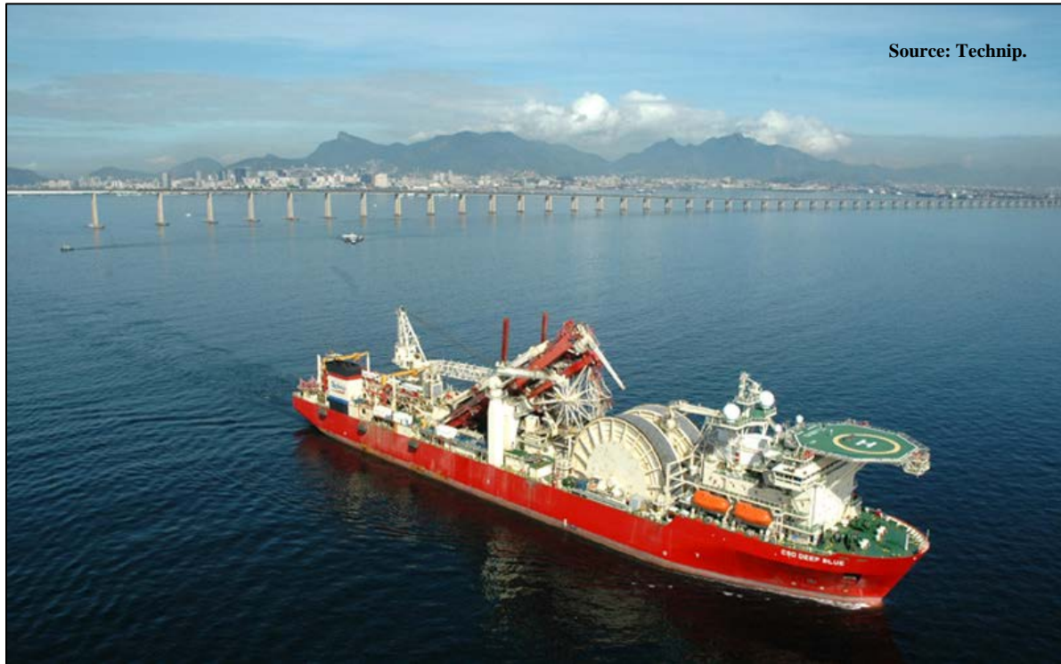
Figure F.11. Technip's Deep Blue high-spec pipelay vessel.
