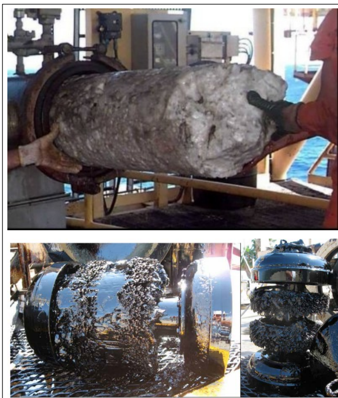
Figure B.6. Hydrates (top) and wax (bottom) removal in pipeline.
