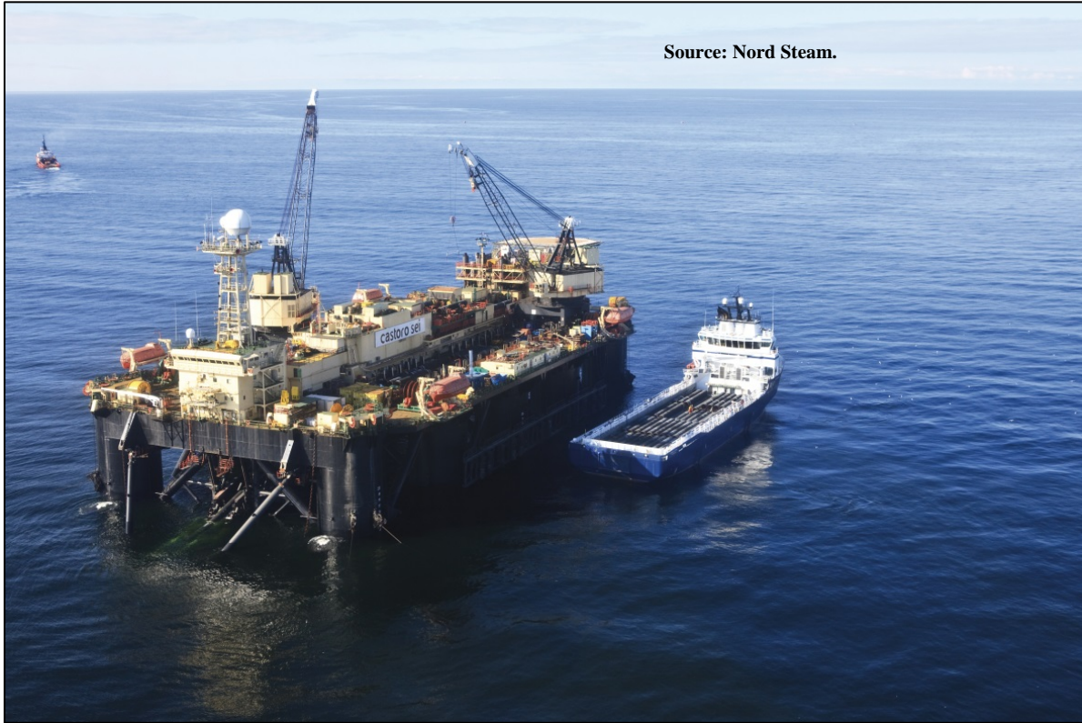
Figure F.9. Castoro Sei , a semi-submersible heavy-lift vessel.
