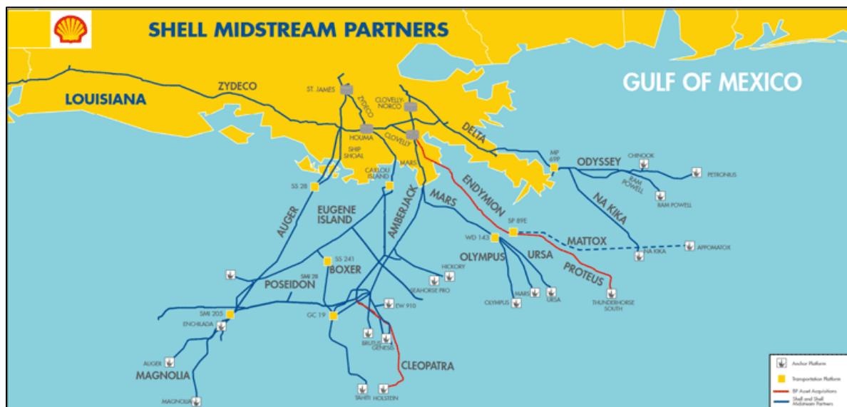
Figure N.19. Shell's oil pipeline network and transportation platforms in yellow.
