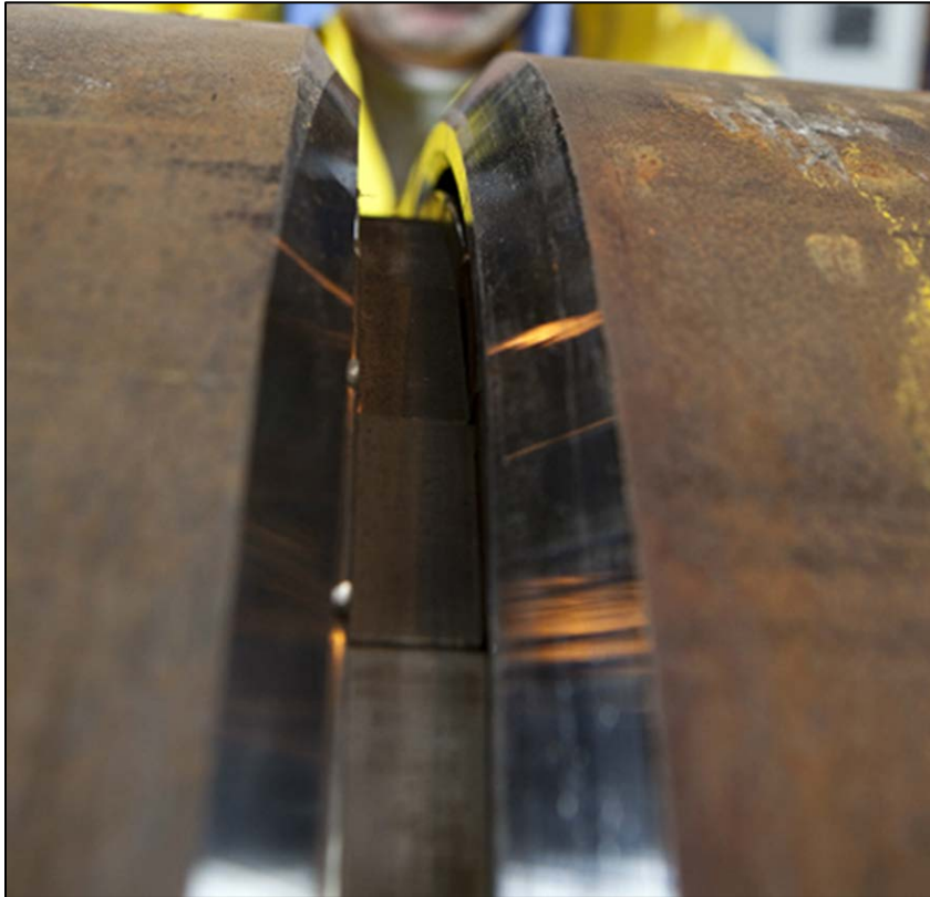
Figure E.1. A typical bevel on an offshore pipeline.
