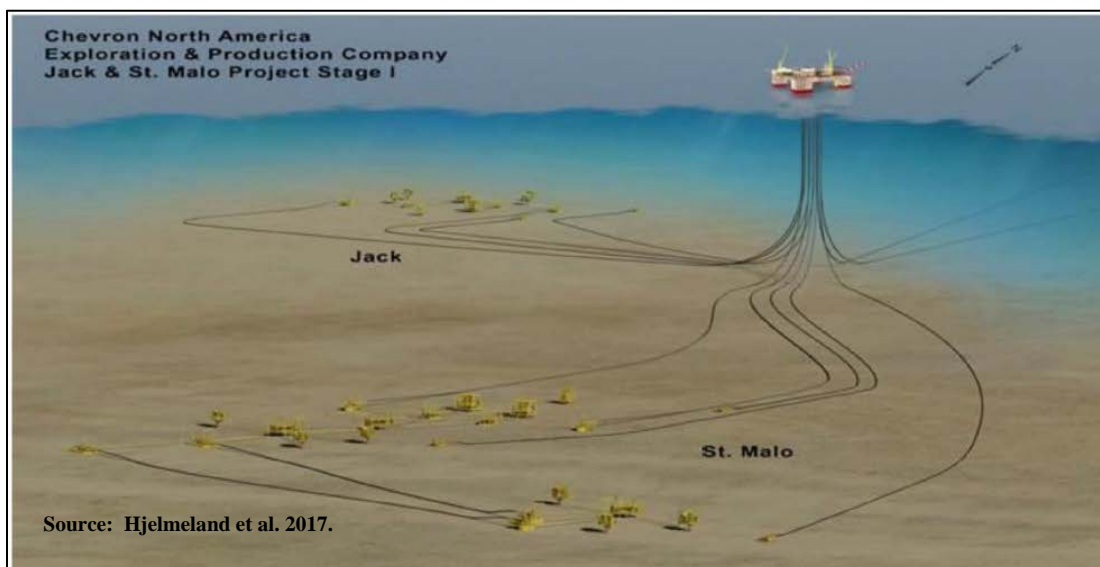
Figure C.18. Jack and St-Malo stage one field layout.
