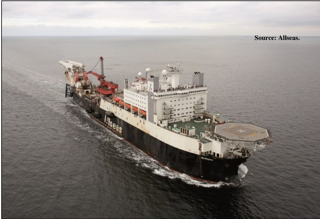
Figure F.13. Allseas' Solitaire ultra high-spec pipelay vessel.
