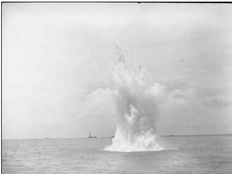
Figure 106. “Detonation of a charge of Nitramon explosive used in seismographic operations” off Louisiana coast, August 1947.
