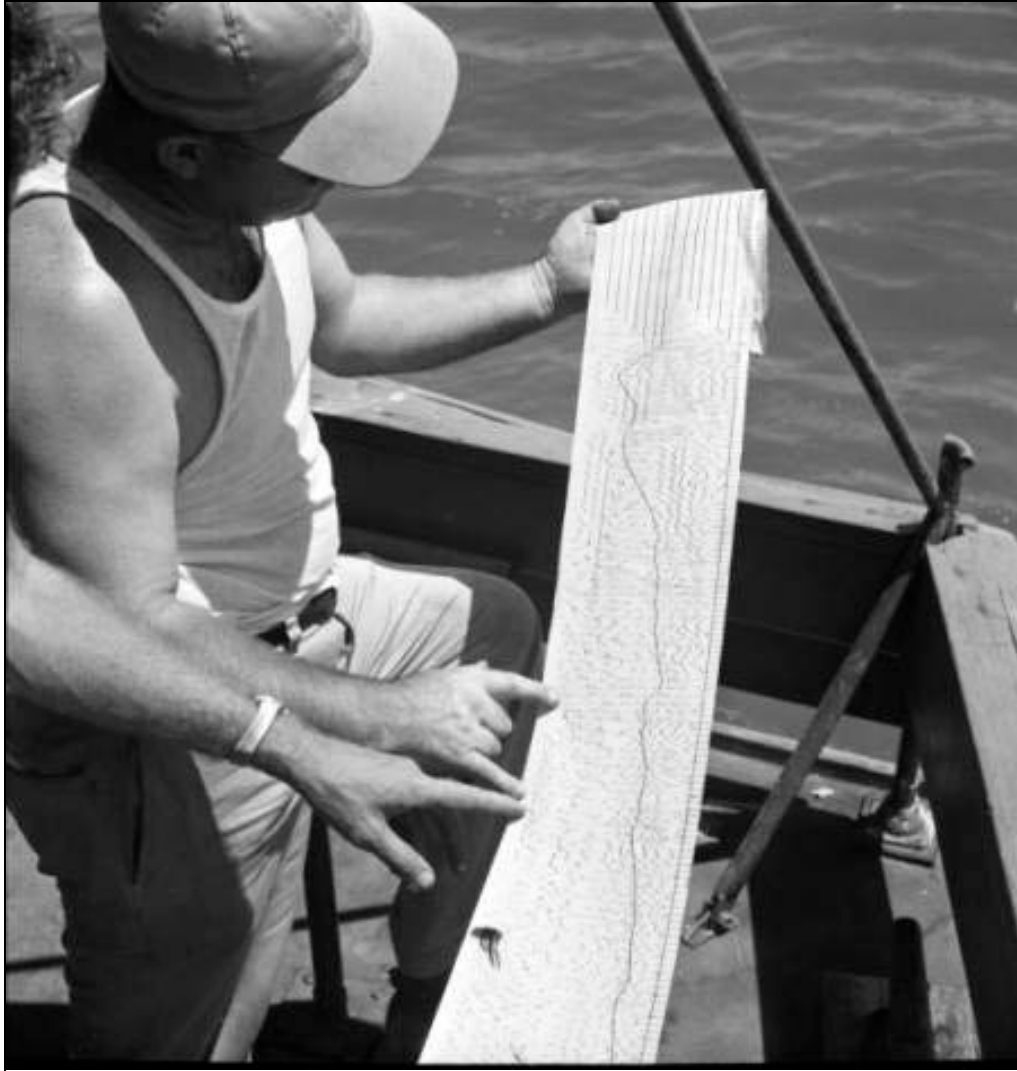
Figure 110. Shot record aboard the instrument ship Seafarer .
