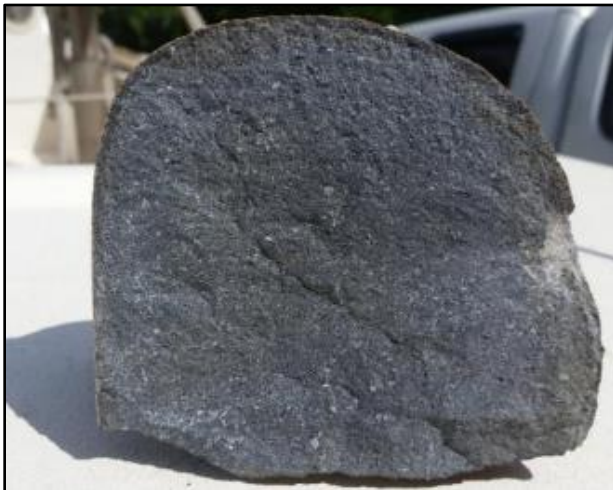
Figure 215. Break face illustrating plutonic granodiorite composition of subject ballast stone.
