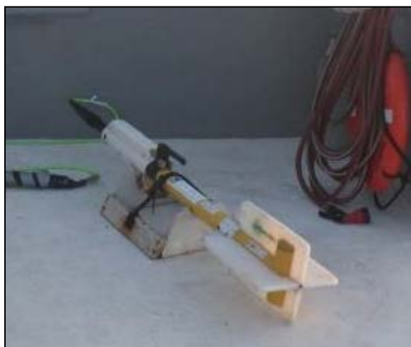
Figure 18. Geometrics G-882 Digital Cesium Marine Magnetometer used to identify magnetic anomalies within the survey areas.
