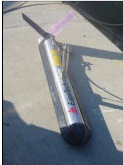
Figure 20. EdgeTech 4200 dual frequency sidescan sonar system.
