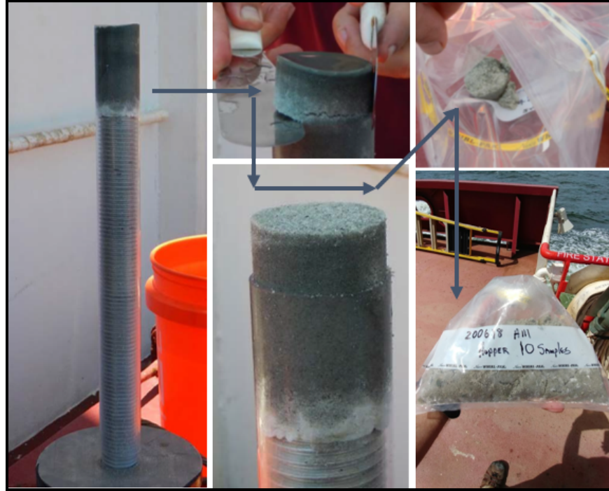
Figure 15. The extrusion and subsampling procedure for hopper bed cores
