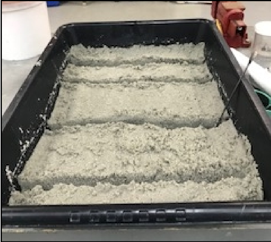
Figure 17. Pan of moist sample with specimens removed for analysis.
