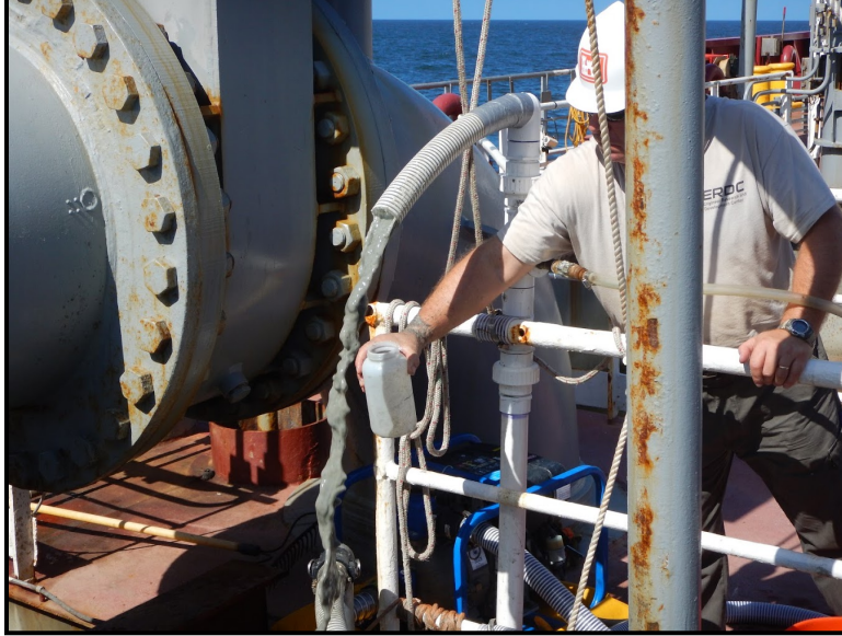
Figure 10. Bottle sampling method used to collect hopper inflow sediments.
