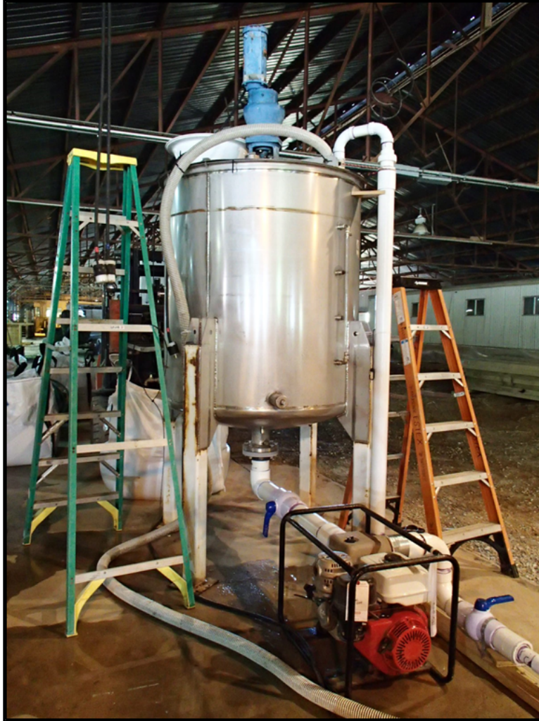
Figure B-3. Sediment mixing tank.
