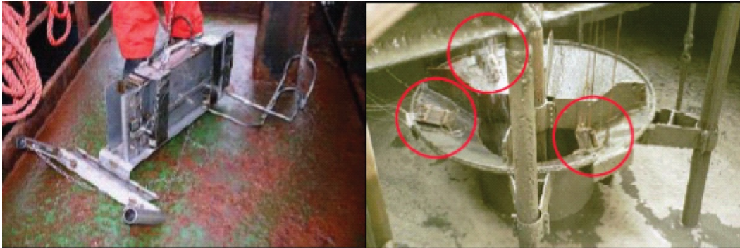
Figure A-6. Photo of the custom flow-through sampler used by Kerssemakers (2004).
