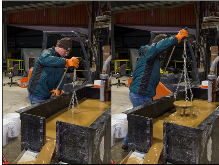
Figure B-11. Laboratory testing of the plate sampler.
