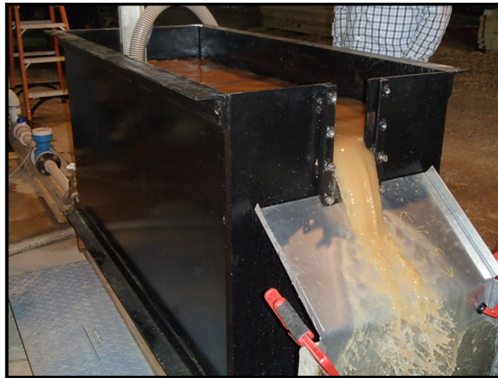
Figure B-6. Model weir tank in overflow.
