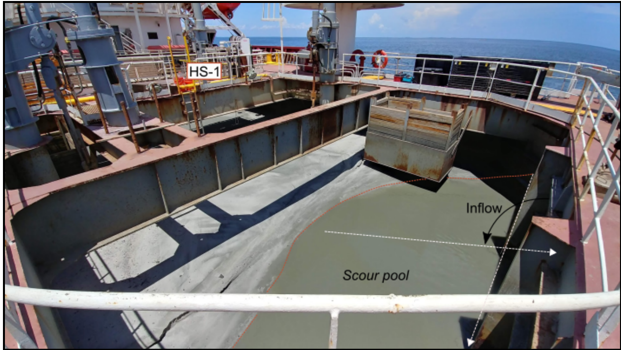
Figure 16. The scour pool at the conclusion of a dredge load.
