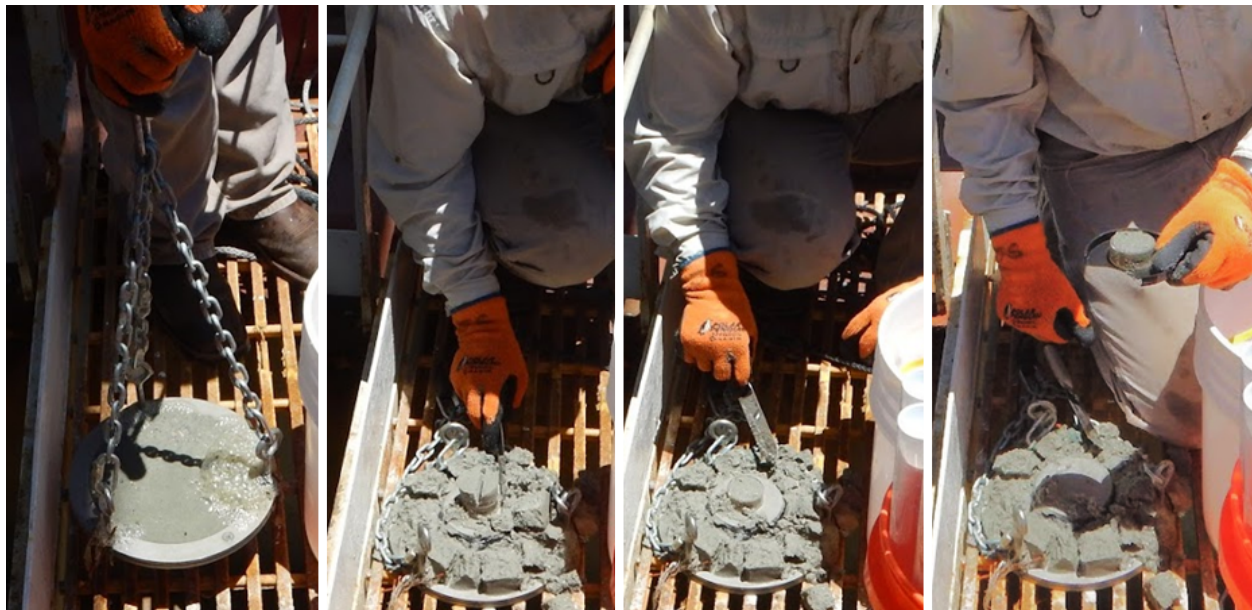
Figure 13. Plate sampling procedure.
