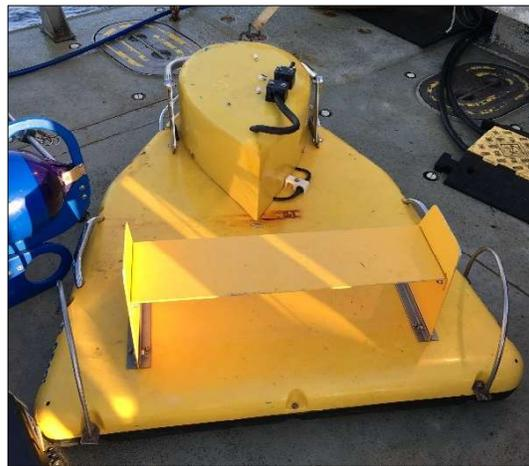
**Photo B-5. Edgetech 512i side-scan sonar.**
