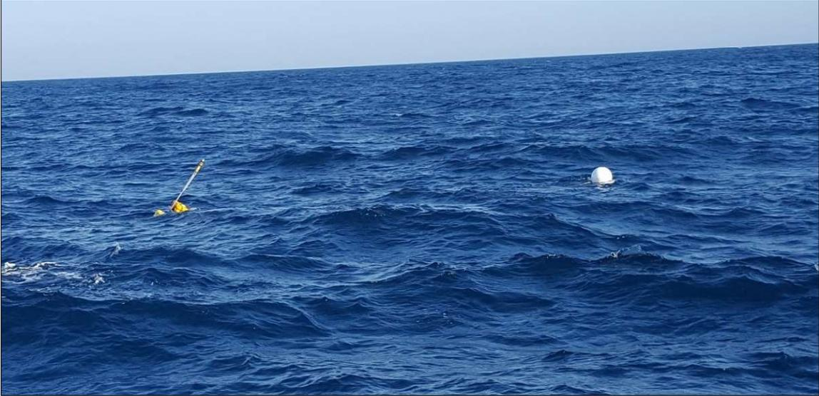
**Photo B-49. Strong currents were encountered at Site 5.** Currents caused the acoustic buoys to pull taut at the end of the bridle and mooring line, which resulted in the control box submerging. In addition, the current caused the hydrophone array cable to drift away from the intended vertical position. Photo courtesy of CSA Ocean Sciences Inc.
