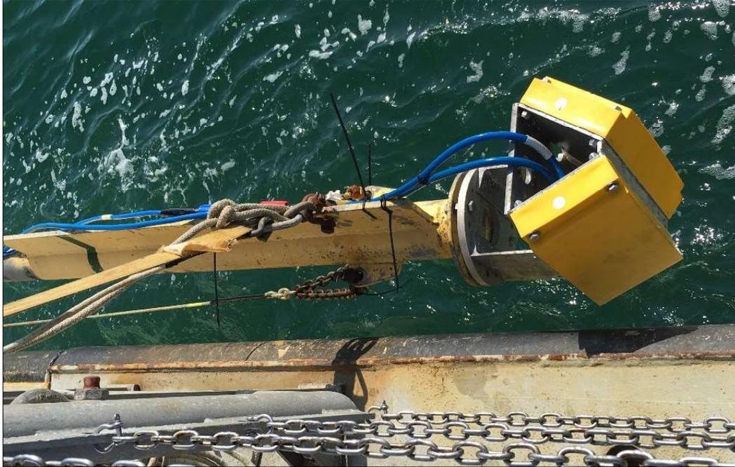
**Photo B-12. SEA SWATHPlus Interferometric Sonar.**
