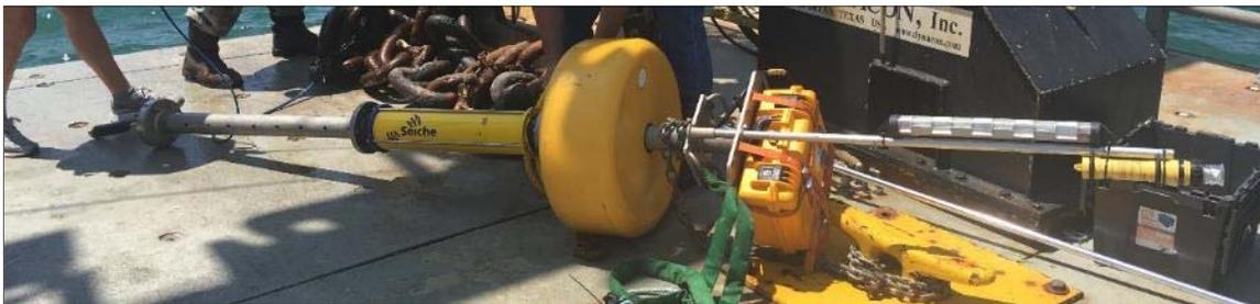
**Figure 2.5-1. Photo of an acoustic data acquisition buoy.**
