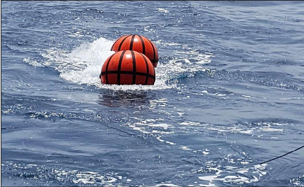
**Photo B-35. Photos of the Mini GI airguns and associated red floats.** Top left, the floats and airgun system ready for deployment. Top right, the active Mini GI airguns in the water. Bottom, the surface bubbles around the floats resulting from airgun pulses. Photos courtesy of CSA Ocean Sciences Inc.
