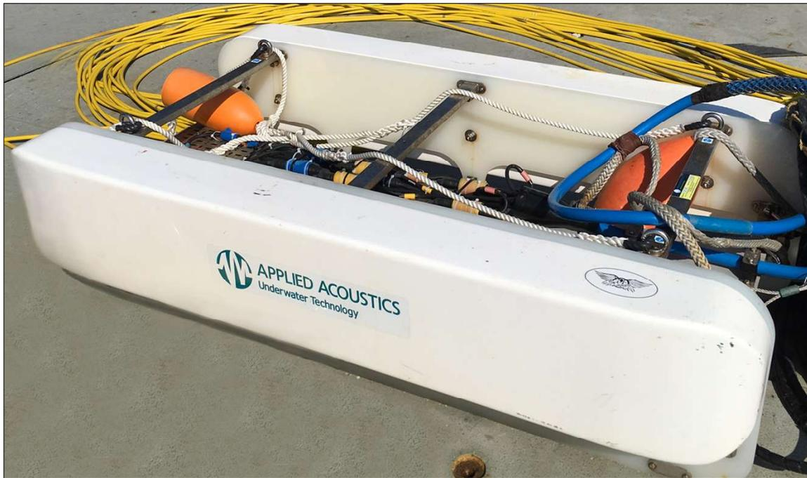
**Photo B-11. Applied Acoustics 251 Boomer (single plate).**
