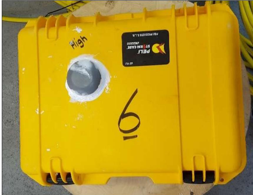
**Photo B-23.** A control box for the acoustic acquisition buoy. The control box was mounted on top of the flotation disc and housed the battery, memory, and data connections to the acoustic data acquisition cylinder. The global positioning system (GPS) antenna is the grey puck on the outside of the box. Photo courtesy of CSA Ocean Sciences Inc.
