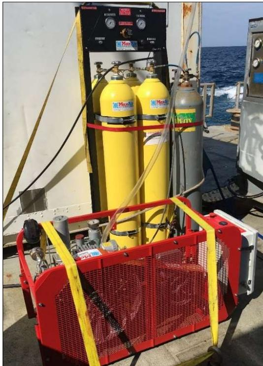
**Photo B-34. The compressor provided compressed air for the airguns.**
