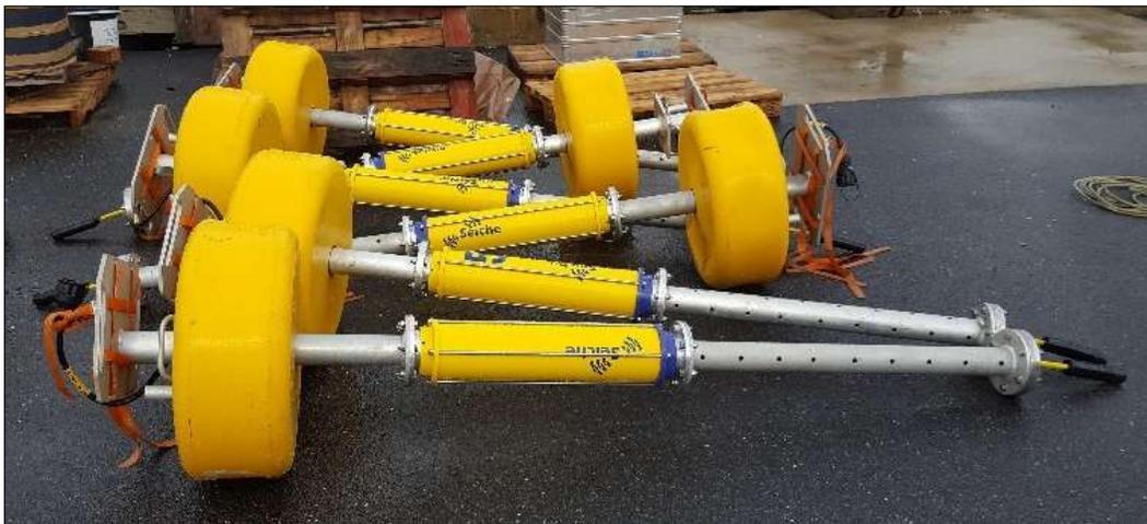
**Photo B-20. Acoustic acquisition buoys.**
