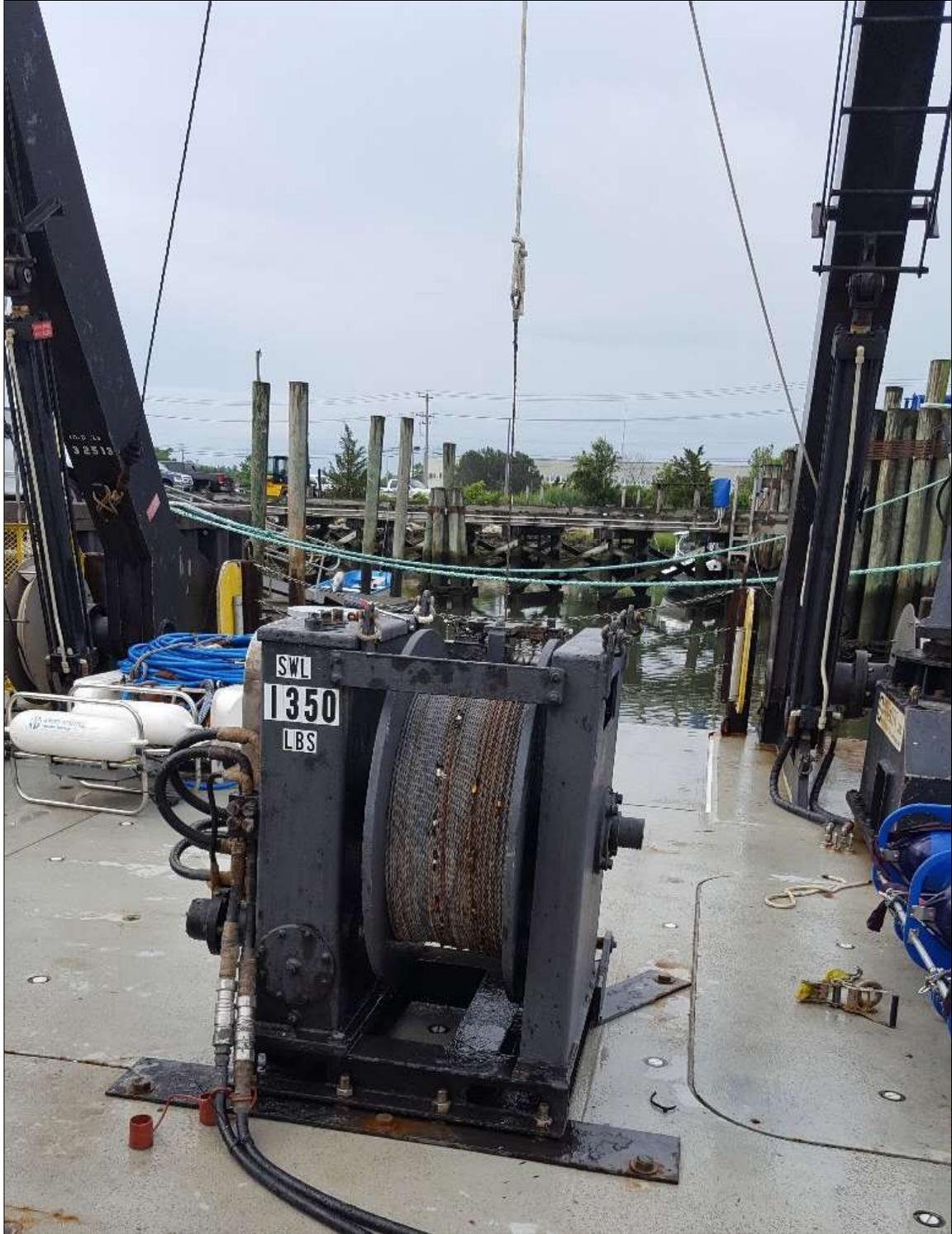
**Photo B-3.** View of the R/V *Hugh R. Sharp* back deck. The winch (foreground) was used to deploy and retrieve field survey equipment. Photo courtesy of CSA Ocean Sciences Inc.
