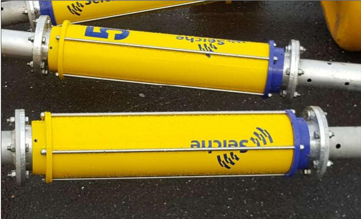
**Photo B-21. Close-up of the acoustic data acquisition cylinder.**
