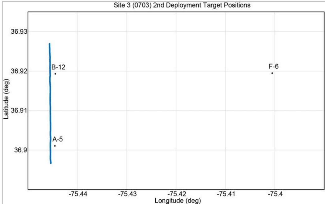
**Figure 3.3-3. Site3 (S3), deployment 2, geographic buoy positions.** Positions A (Buoy5), B (Buoy12), and F (Buoy6) as well as the source track (blue). North is vertical (upward). Note the source went back and forth along the source track. Latitude and longitude are not to scale, so bearings and angles are not properly displayed and are for general orientation only.
