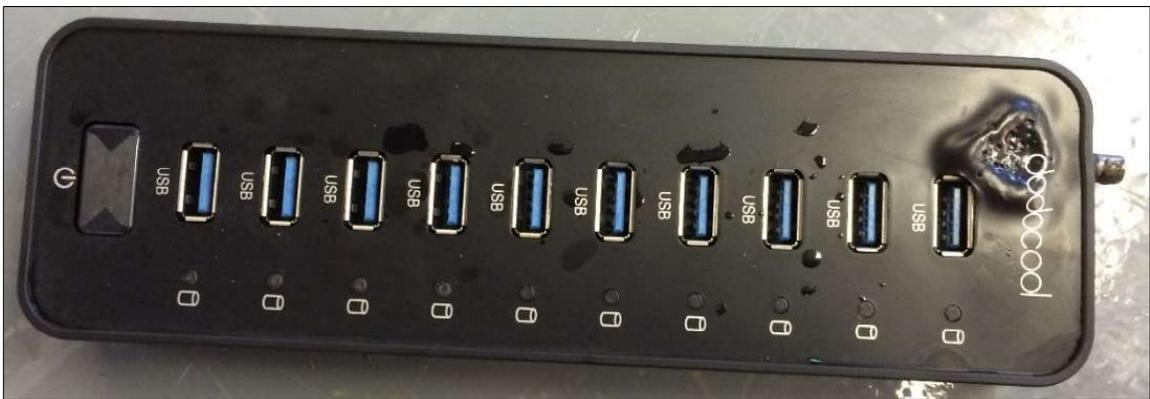
**Photo B-40. Close-up of internal components of a control box.** Top shows water intrusion on the USB hub, which resulted in failure to record data. Bottom image shows the USB hub melted from saltwater intrusion. Photos courtesy of CSA Ocean Sciences Inc.
