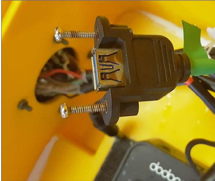
**Photo B-41. Internal component corrosion.** Close-up of internal component of a control box showing corrosion (rust) on a female connector resulting from saltwater intrusion. Once corroded, the connector would no longer make a connection. Photo courtesy of CSA Ocean Sciences Inc.
