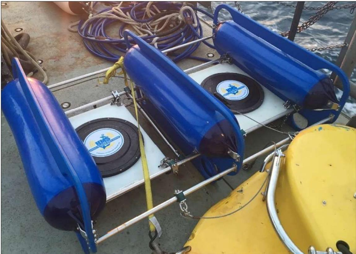
**Photo B-15. FSI Bubble Gun (dual plate).**
