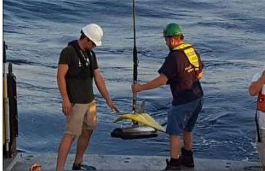
**Photo B-33. Retrieval of the Edgetech 4200 (between two personnel).**
