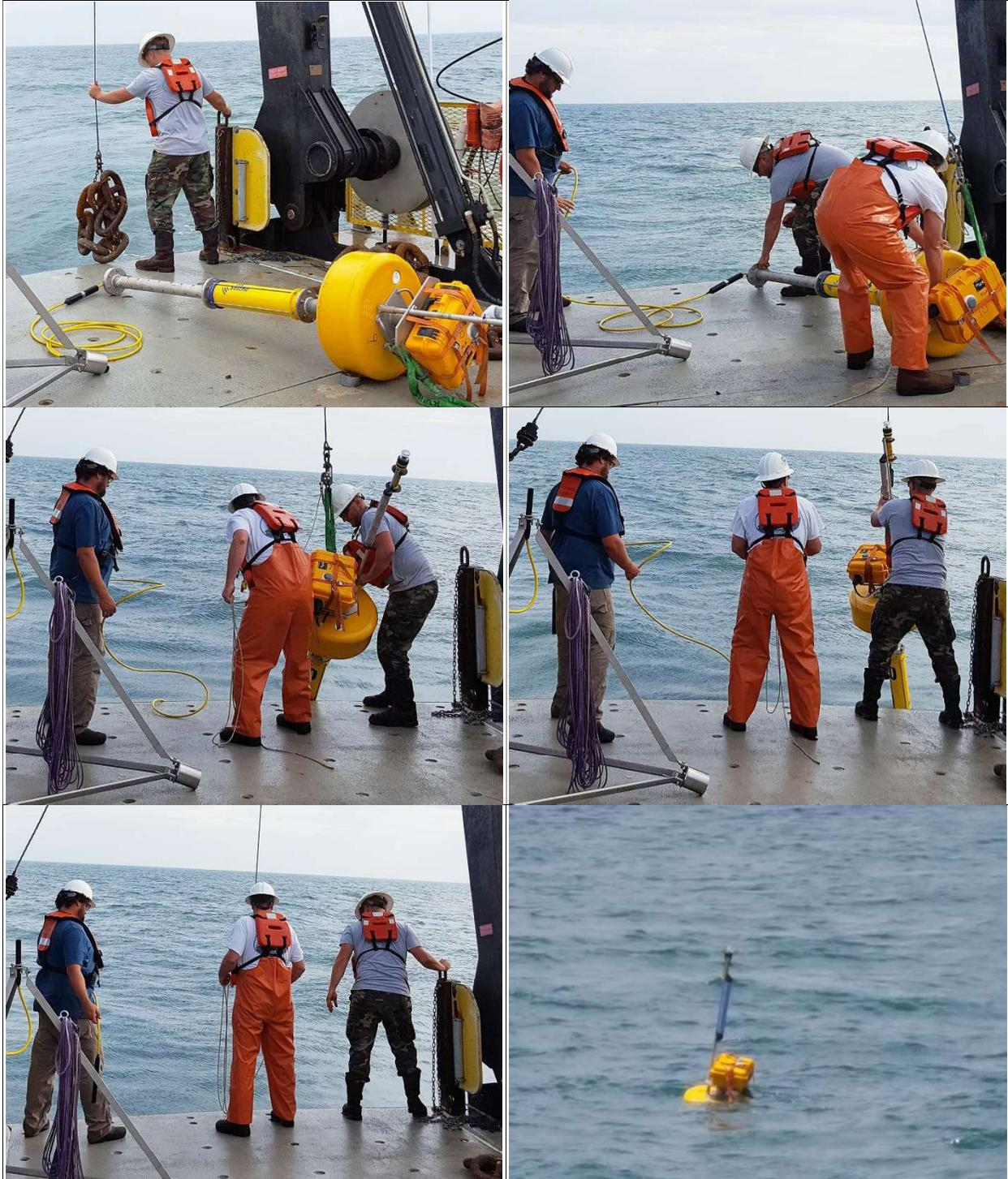
**Photo B-30. Process of acoustic acquisition buoy deployment.** Anchor chain being deployed by CSA Ocean Sciences Inc. personnel, followed by lift and release of the acoustic acquisition buoy by CSA personnel with the assistance of R/V *Hugh R. Sharp* deck crew. The tripod platform being placed at position D is visible in the lower left corner of the images. The yellow hydrophone cable can be seen in the hand of the crew member on the far left. Photos courtesy of CSA Ocean Sciences Inc.
