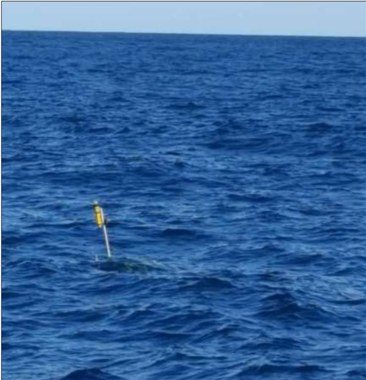
**Photo B-50. Acoustic acquisition buoy in strong currents.** Currents caused the control box and buoy to completely submerge. However, the control boxes were waterproofed as part of the redesign, and there was minimal (if any) water intrusion. Photo courtesy of CSA Ocean Sciences Inc.
