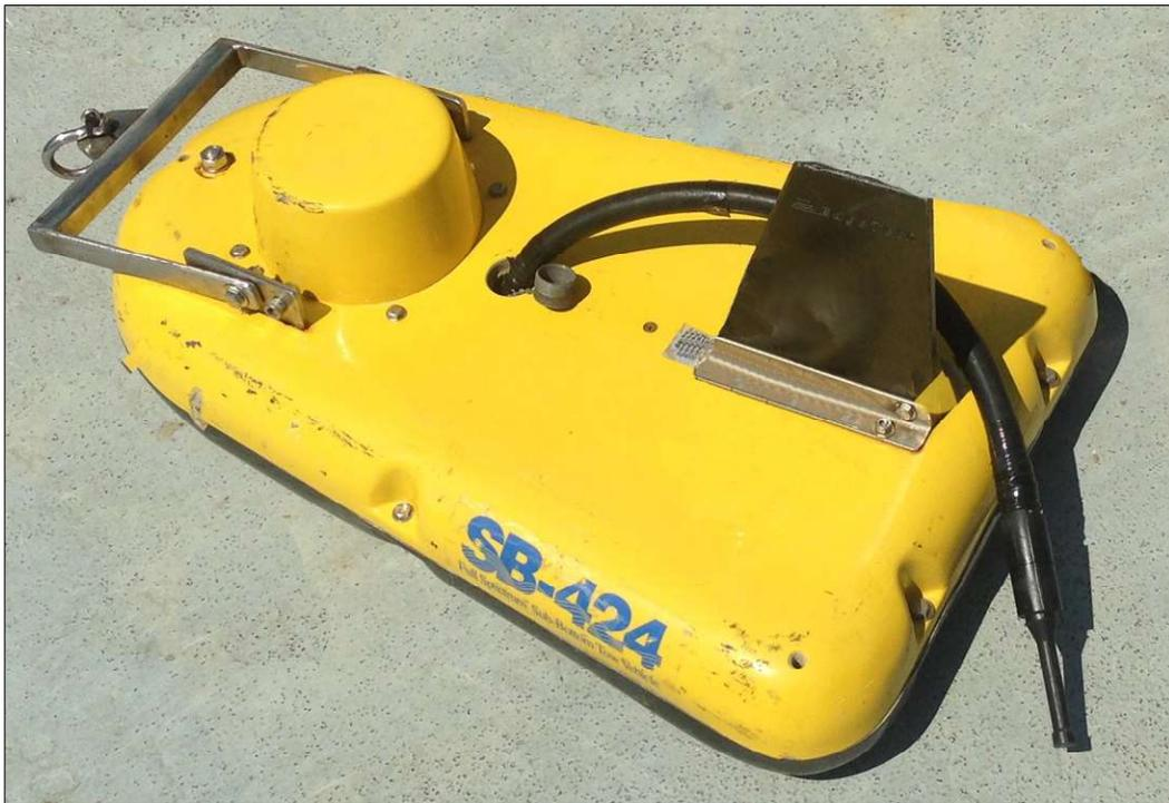
**Photo B-13. Edgetech SBP 424 tow vehicle for 3100p and 3200XS CHIRP side-scan sonar.**
