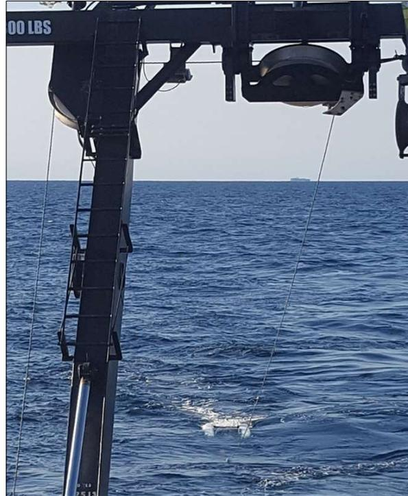
**Photo B-36.** Photo of the Applied Acoustics 251 Boomer (white pontoon) just under water surface.
