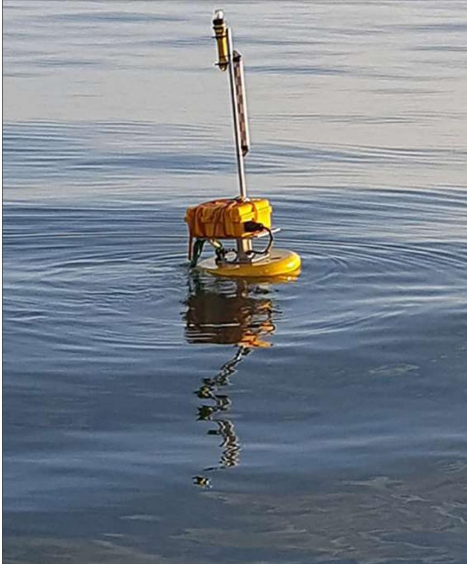
**Photo B-39. Photo of an acoustic buoy in calm waters.** The yellow float (disc) should be resting higher above the water line; this image shows lack of positive buoyancy with too much of the float below the water line. Photo courtesy of CSA Ocean Sciences Inc.
