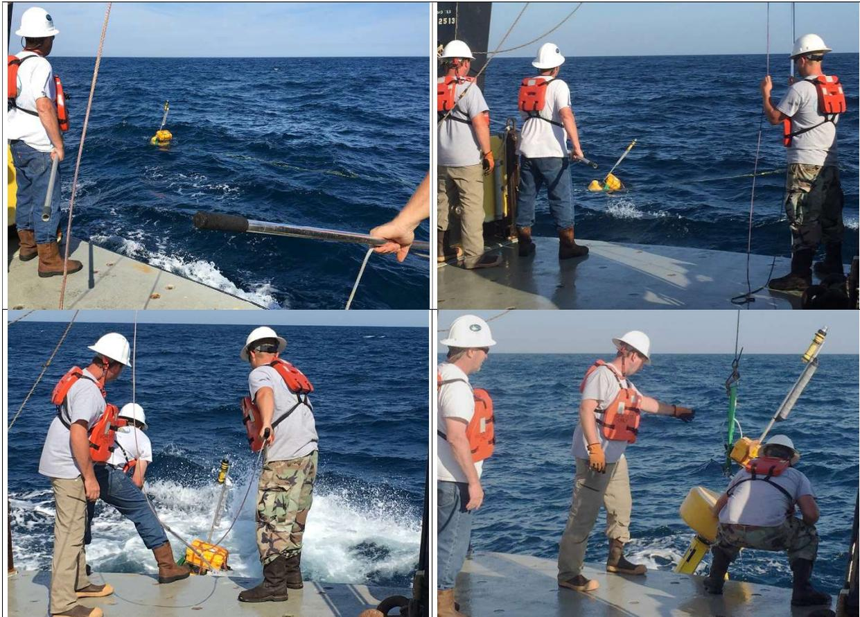
**Photo B-31. Retrieval process of an acoustic acquisition buoy.** The R/V *Hugh R. Sharp* backs down on the buoy, and then the buoy is hooked with a long reach (pole) and secured to the winch cable via the green strap. Retrieval was performed by CSA Ocean Sciences Inc. personnel with the assistance of R/V *Hugh R. Sharp* deck crew. Photos courtesy of CSA Ocean Sciences Inc.
