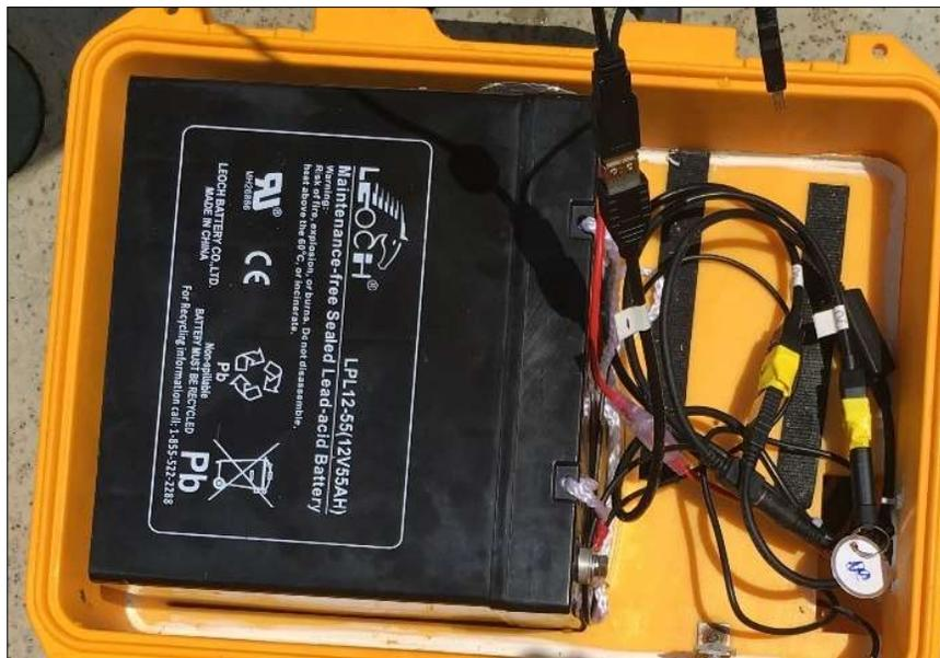
**Photo B-24.** Interior of a control box for the acoustic acquisition buoy. The black box is the battery, and the USB data storage device (thumb drive) is on the right. Photo courtesy of CSA Ocean Sciences Inc.
