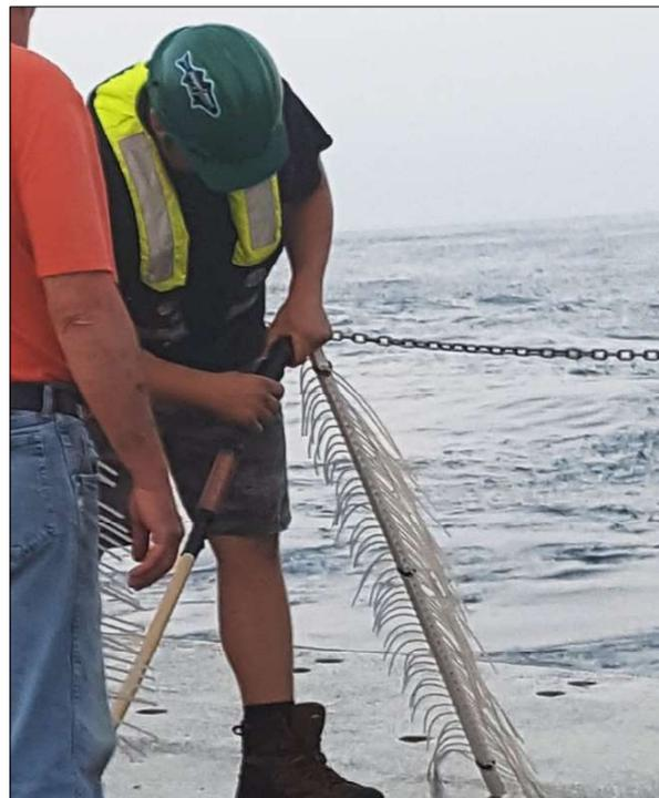
**Photo B-37.** Photo of the SIG 2 Mini-Sparker (white pole with fringe, which are the electrodes) in preparation for deployment.
