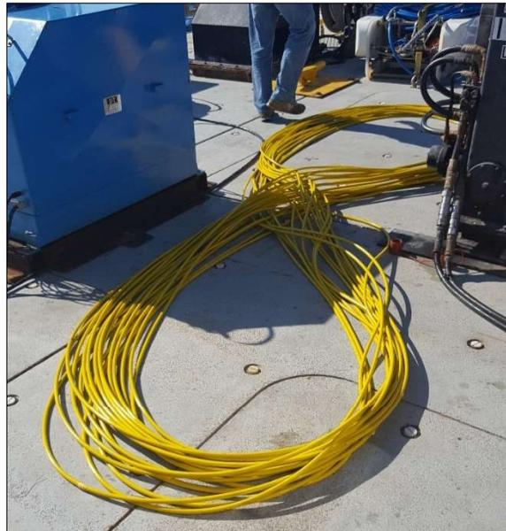
**Photo B-28. Yellow hydrophone cable coiled on deck and ready for deployment.** The 200-m cable was attached to position D (located directly under the vessel track) on a tripod platform. Photo courtesy of CSA Ocean Sciences Inc.
