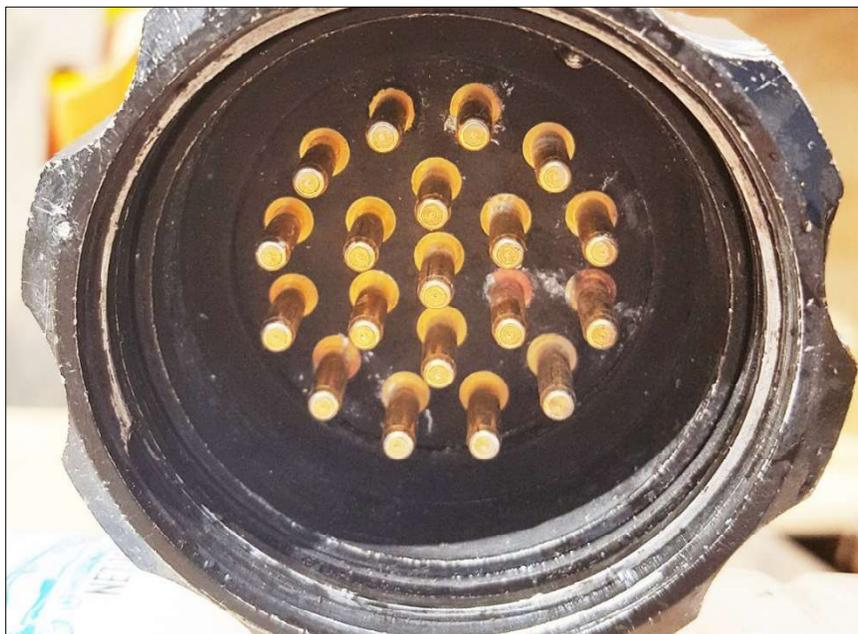
**Photo B-42. External connector corrosion.** Close-up of the external connector to the control box showing early corrosion (rust and white precipitate) on the connector, resulting from saltwater intrusion due to the lack of an O-ring. Photo courtesy of CSA Ocean Sciences Inc.
