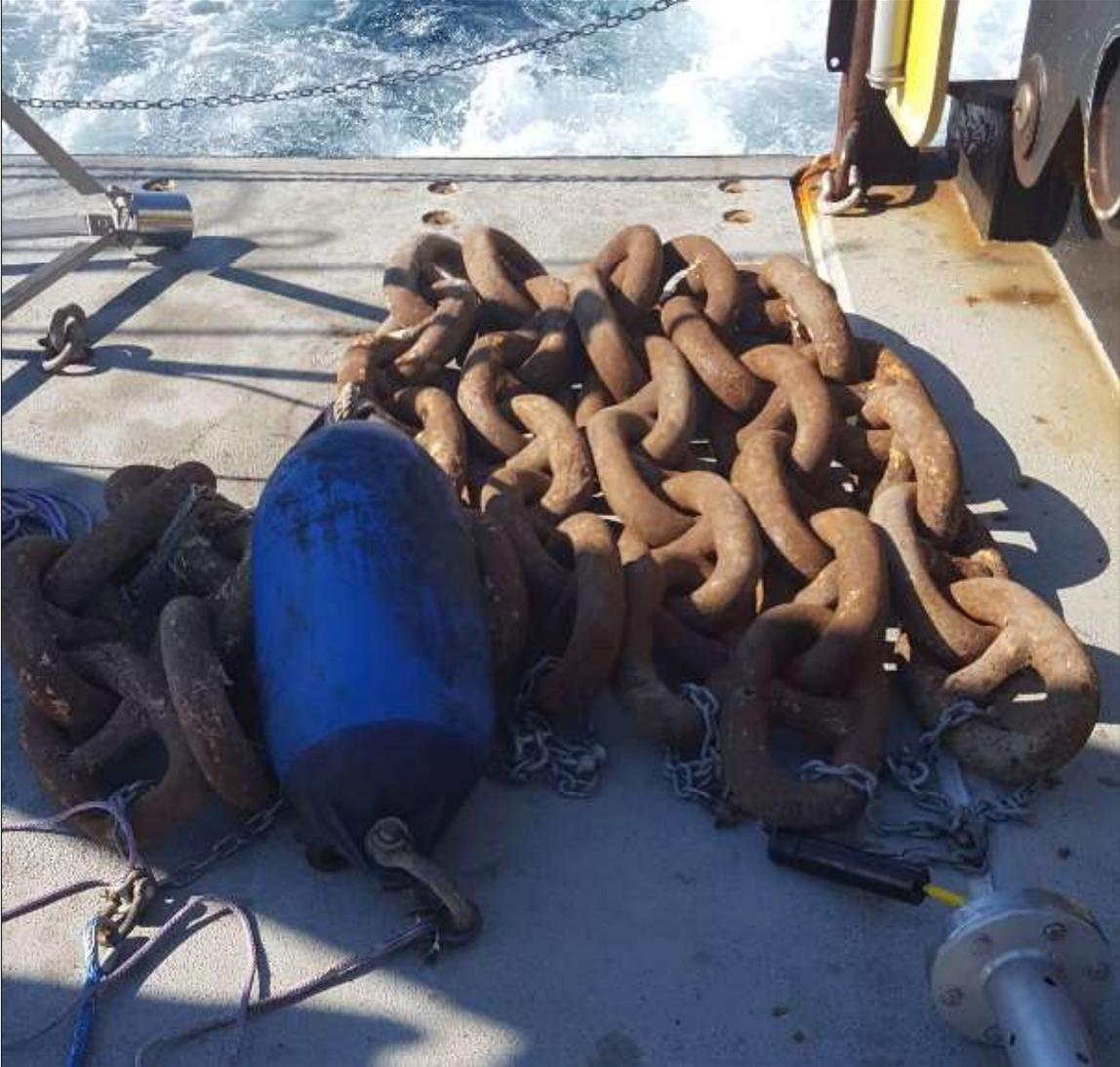
**Photo B-29.** Anchor chain section served as bottom mooring for the buoys.
