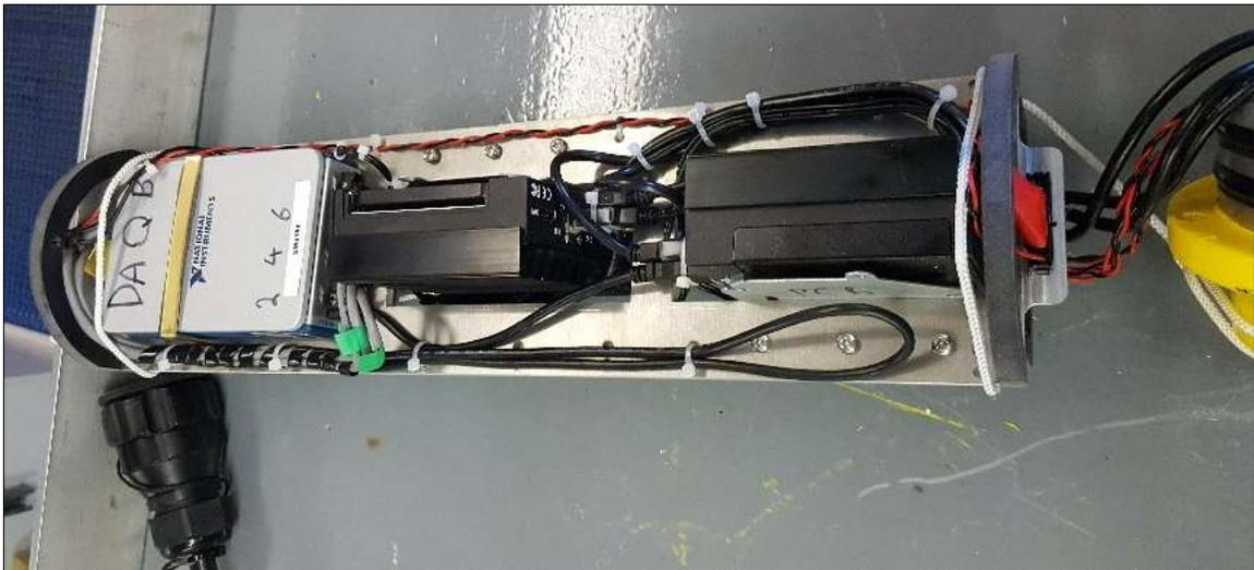
**Photo B-22. Internal view of the data acquisition cylinder, showing the twin acquisition systems.**
