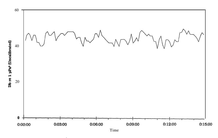
FIGURE 13. Variability of the **icebreaking** sounds, 20-1000 Hz band level, during the first 15 min of the playback tape. Levels are in **dB** relative to the minimum one-third octave **level** observed during the 15 min period.
