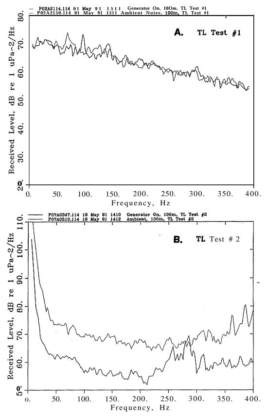
FIGURE 21. Noise spectra observed 100 m from the ice camp with the generator on and off. Data were obtained during the four transmission loss tests in 1991. The sound projectors were silent during these measurements.
