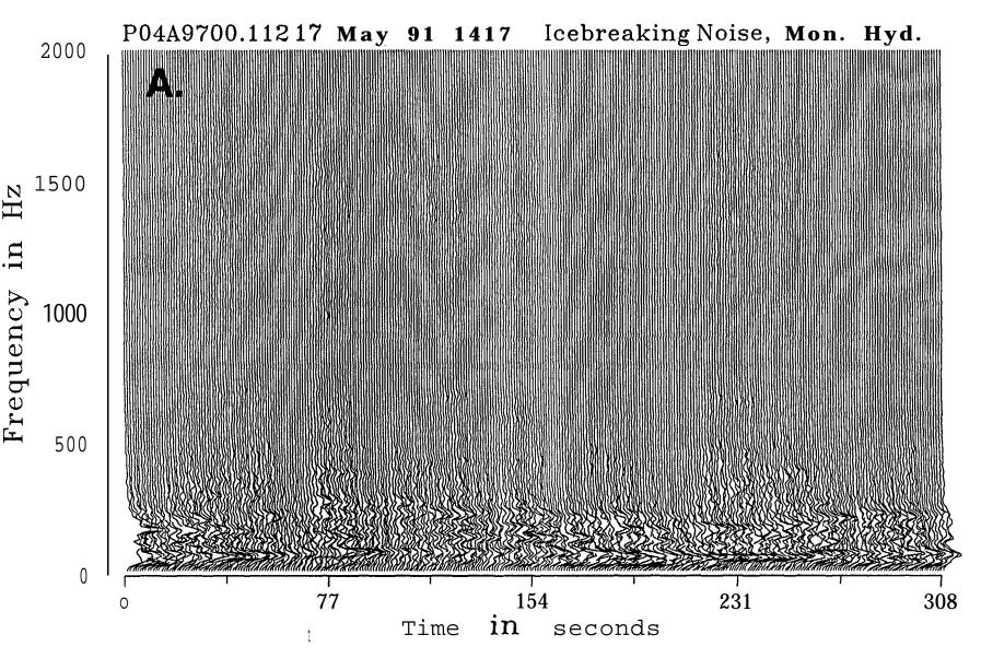
FIGURE 15. Waterfall spectrogram of the icebreaker playback sounds extending over 5 min starting at 14:17 on 17 May 1991. The data span the frequency range 20-2000 Hz. (A) is for the signal at the monitor hydrophore near the projectors. (B) is for the signal received at a **sonobuoy** 0.73 km from the projectors.
