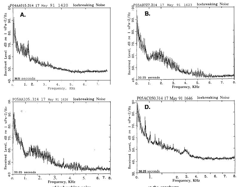
FIGURE 17. Four examples of icebreaking noise spectra for sounds received at the sonobuoy during a playback experiment, 17 May  $\Re$  1991, range 0.73 km.
