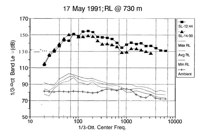
FIGURE 34. Third-octave levels of sounds 1 m from the projector (squares, triangles) and at a **sonobuo** y 730 m from the projector (max., mean and min. of 10 examples) during icebreaker noise playback on 17 May 1991. Plus signs show ambient noise levels after the playback. All data are in **dB** re 1 **\muPa**.
