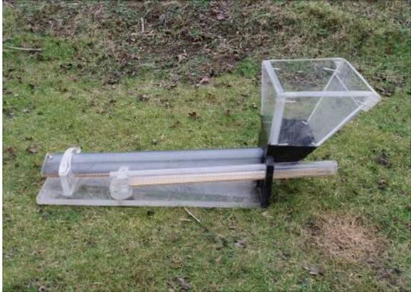
**Figure 2.** An example of an eel trough (a) and an eel tube (b) suitable for measuring eels. An eel trough could be used to measure and tag eels and an eel tube could be modified to provide access to the dorsal for tag attachment. Both can be used with flowing seawater. Images from The Eel Manual, page 21-22; uploaded as supporting information.
