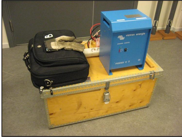
Figure 7. The wooden box that contains the electronics unit and recording instruments. Missing in the picture is the cable, which connects the “dry electronic” and the sub-surface sledge shown in Fig. 5.
