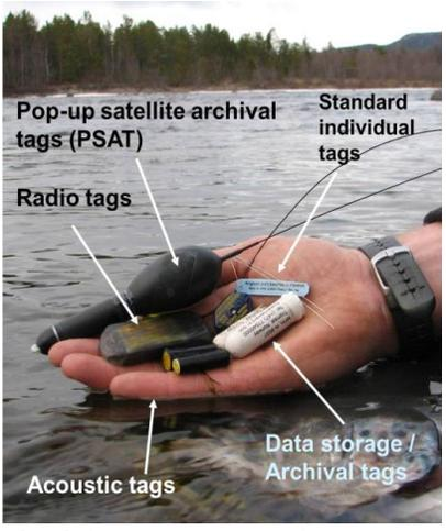
**Figure 1.** Different types of tags for fish movement studies. Note the difference in size of the pop-up satellite tag compared to the acoustic tag. Image from Thorstad et al., 2013.
