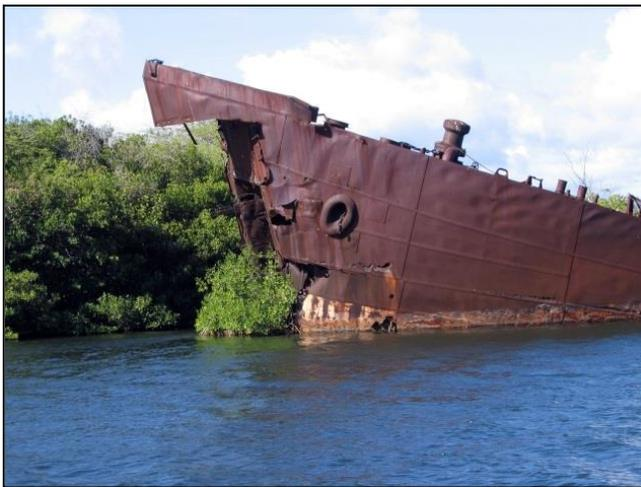
Figure 64: Bow of *LST-480* (RN771), ramp and doors missing, remains at West Loch, Pearl Harbor. (NOAA ONMS)
