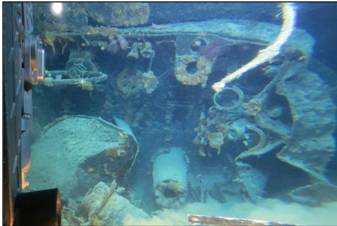
Figure 70: Bridge atop the conning tower (on STBD side) of the *I-400* Japanese submarine. (NOAA ONMS)
