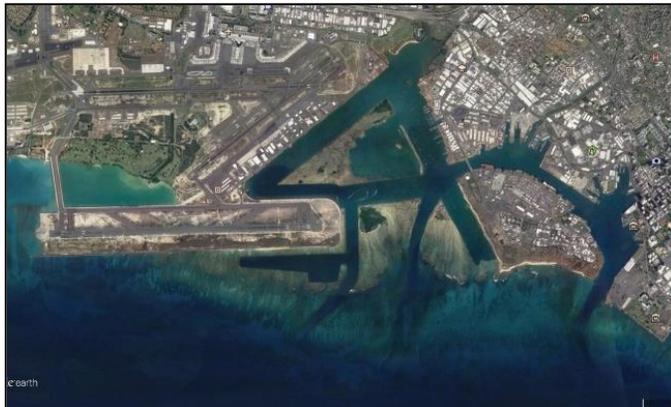
Figure 57: Triangular Ke`ehi Lagoon 1930s seaplane runways are clearly visible near the modern-day HNL reef runway. (Google Earth © 2016 Google Data USGS)
