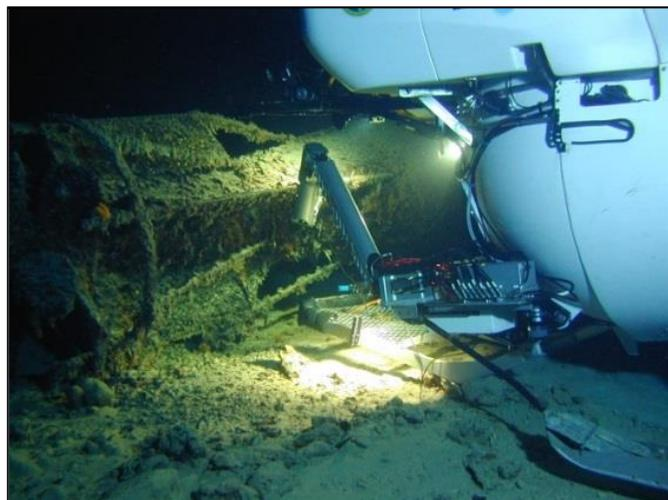
Figure 14: HURL Pisces IV measuring conductivity through the corrosion surface of the Japanese midget sub (RN740). (HURL/NOAA ONMS 2005)
