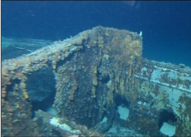
Figure 17: Rusticle formation, view from the Pisces V into the cab of a WWII AMTRACK (RN578); O`ahu. (NOAA ONMS)
