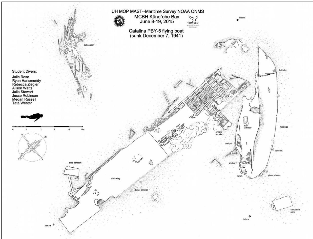
Figure 62: Baseline trilateration plan of the PBY-5 Catalina (RN834) produced by MAST 2015 students in the murky waters of Kāne`ohe Bay. (NOAA ONMS)
