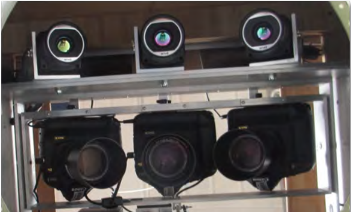
Figure 13. NOAA Twin Otter belly-port camera setup: three FLIR SC645 thermal imagers (top), paired with three Canon 1Ds Mark III digital SLR cameras (bottom).
