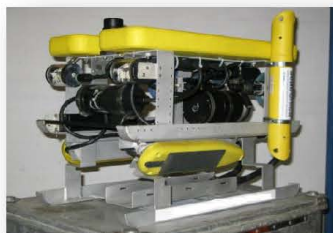
Bathyswath on a micro-ROV
