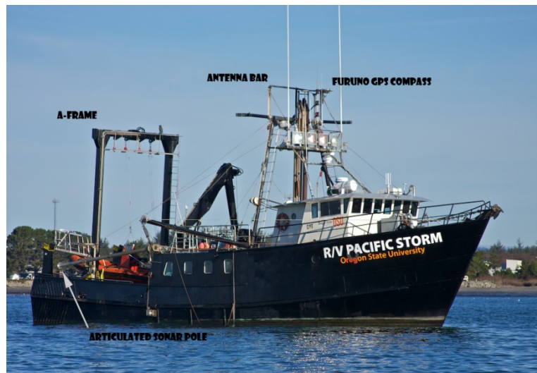
Figure 8. The R/V Pacific Storm , owned and operated by the Marine Mammal Institute at Oregon State University, was utilized as the multibeam mapping platform for this study
