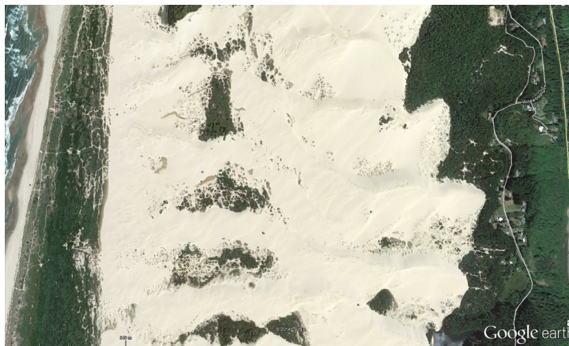
Figure 32. Dune field south of Winchester, OR. These dunes are roughly the same scale as the interpreted paleo dunes on the SETS and BOEM study areas, having wavelengths of ~ 300-400 m (other nearby dune fields have much shorter wavelengths). The wind direction indicated by these dunes is northerly, while the offshore possible paleo dunes suggest a northeasterly prevailing wind.
