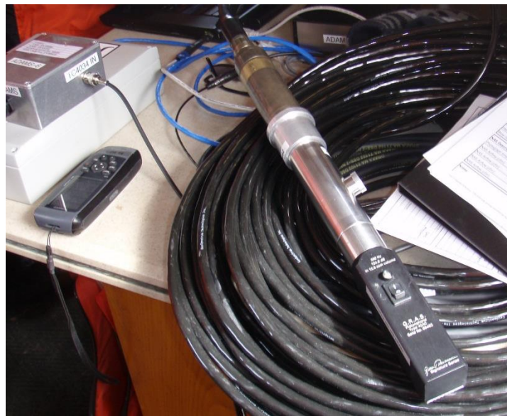
Figure B-1. Example of a GRAS pistonphone calibrator on a hydrophone. Each hydrophone type has a customized adapter whose volume was measured with a NIST verified Larson-Davis Sound Level Meter.
