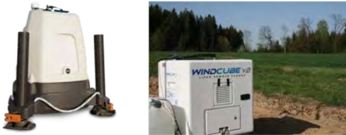
Figure 3-9: Left- Natural Power LIDAR System; Right- Leosphere WINDCUBE LIDAR System.
