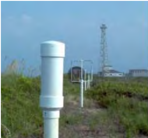
Figure 4-10: Compact loop and standard wide-band copper pipe loops are shown for size comparison.
