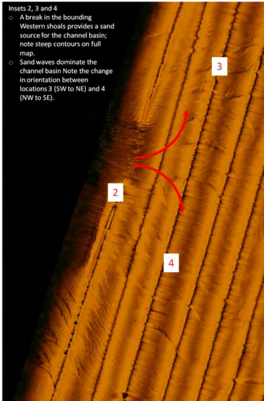
Figure 7-13: Detail from Figure 7-11 showing break in western shoal which supplies sand to the channel basin.
