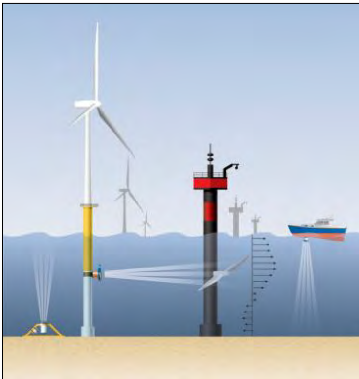
Figure 6-1: Illustration of vertically and horizontally oriented ADCPs.
