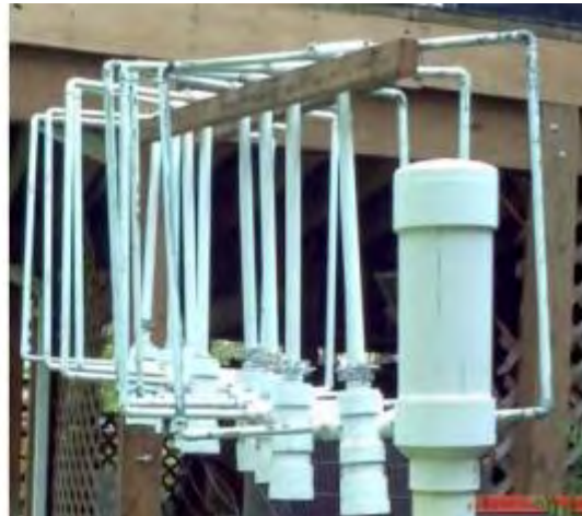
Figure 4-10: Compact loop and standard wide-band copper pipe loops are shown for size comparison.
