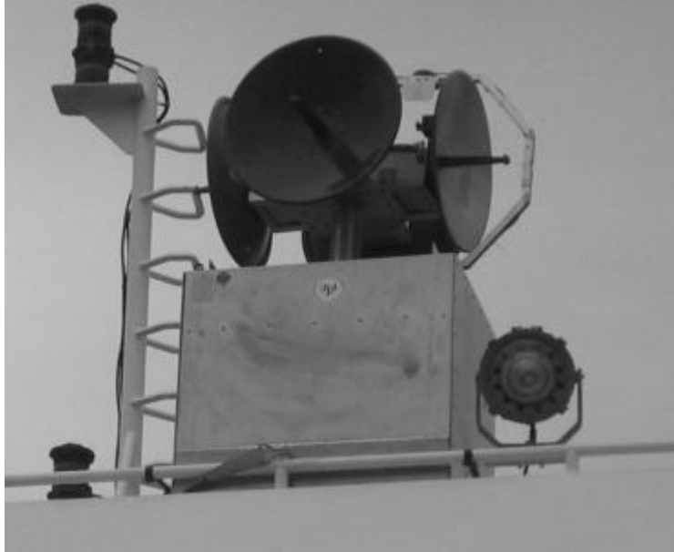
Figure 5-1: The APL/UW coherent real-aperture radar CORAR mounted on the R/V Thompson. All four parabolic antennas are vertically polarized.
