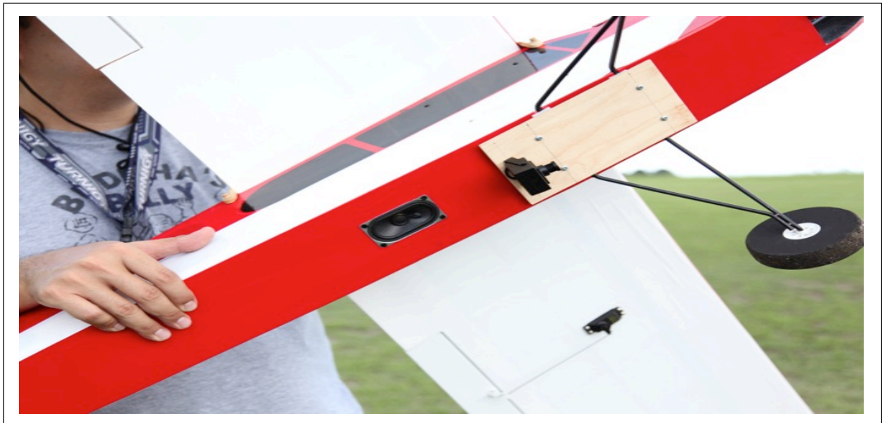
Figure 18. Radio-controlled aircraft with speaker mounted to underside of airframe.
