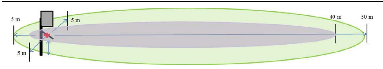
Figure 59. Minimum (gray) and maximum (green) range of detection of the ultrasonic microphone within the ReBAT ® housing.
