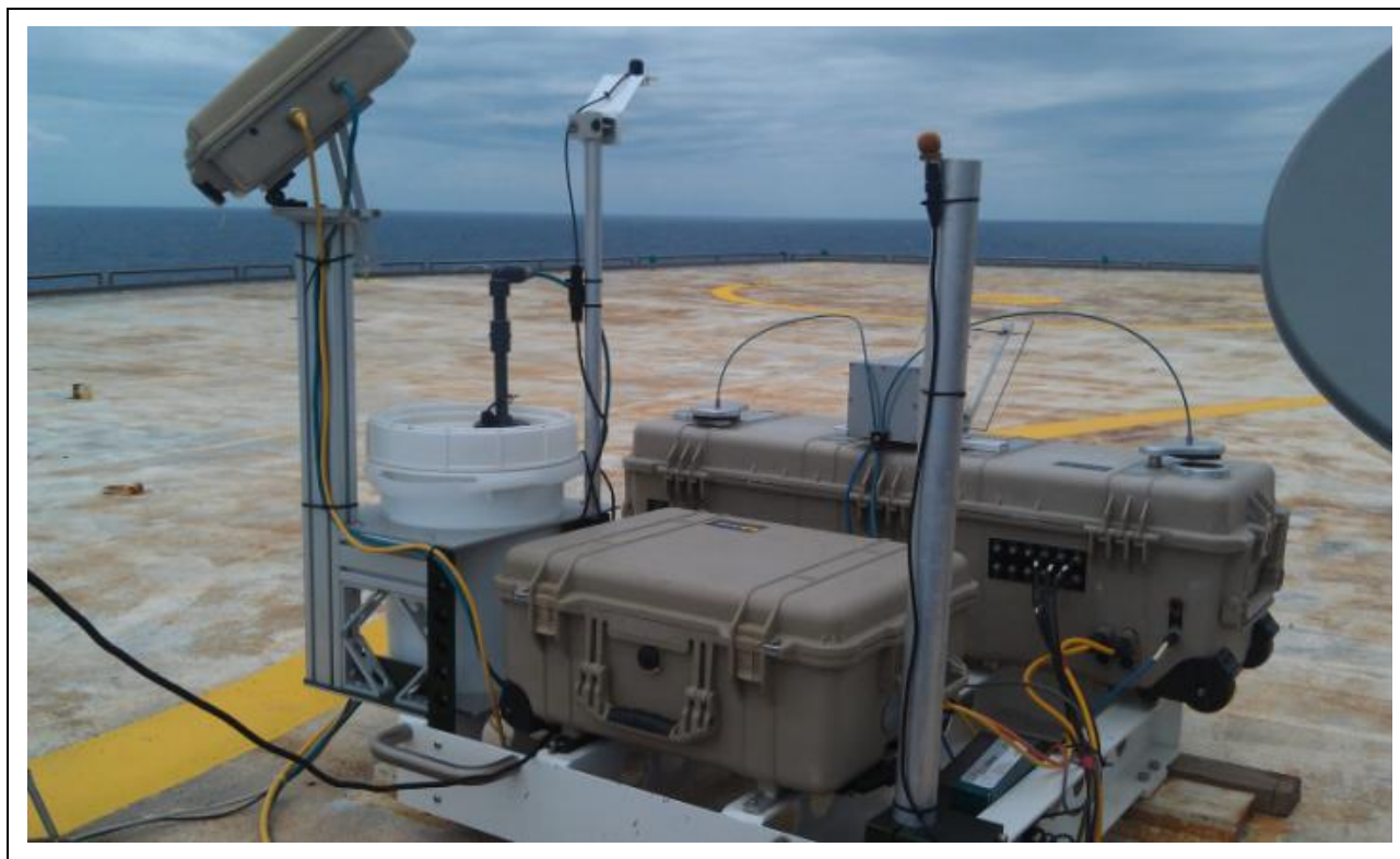
Figure 46. The mounting frame designed to streamline deployment and decommissioning.
