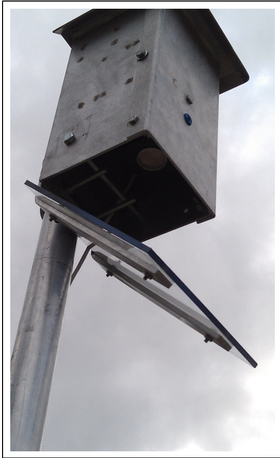
Figure 52. View of underside of the ReBAT ® housing with the AR-125 microphone visible inside pointing down at the reflector plate.
