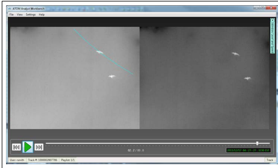
Figure 26. Screenshot of analyst client software showing target flight path feature on a set of bird tracks from Frying Pan Shoals Dec 2011 thermographic data.
