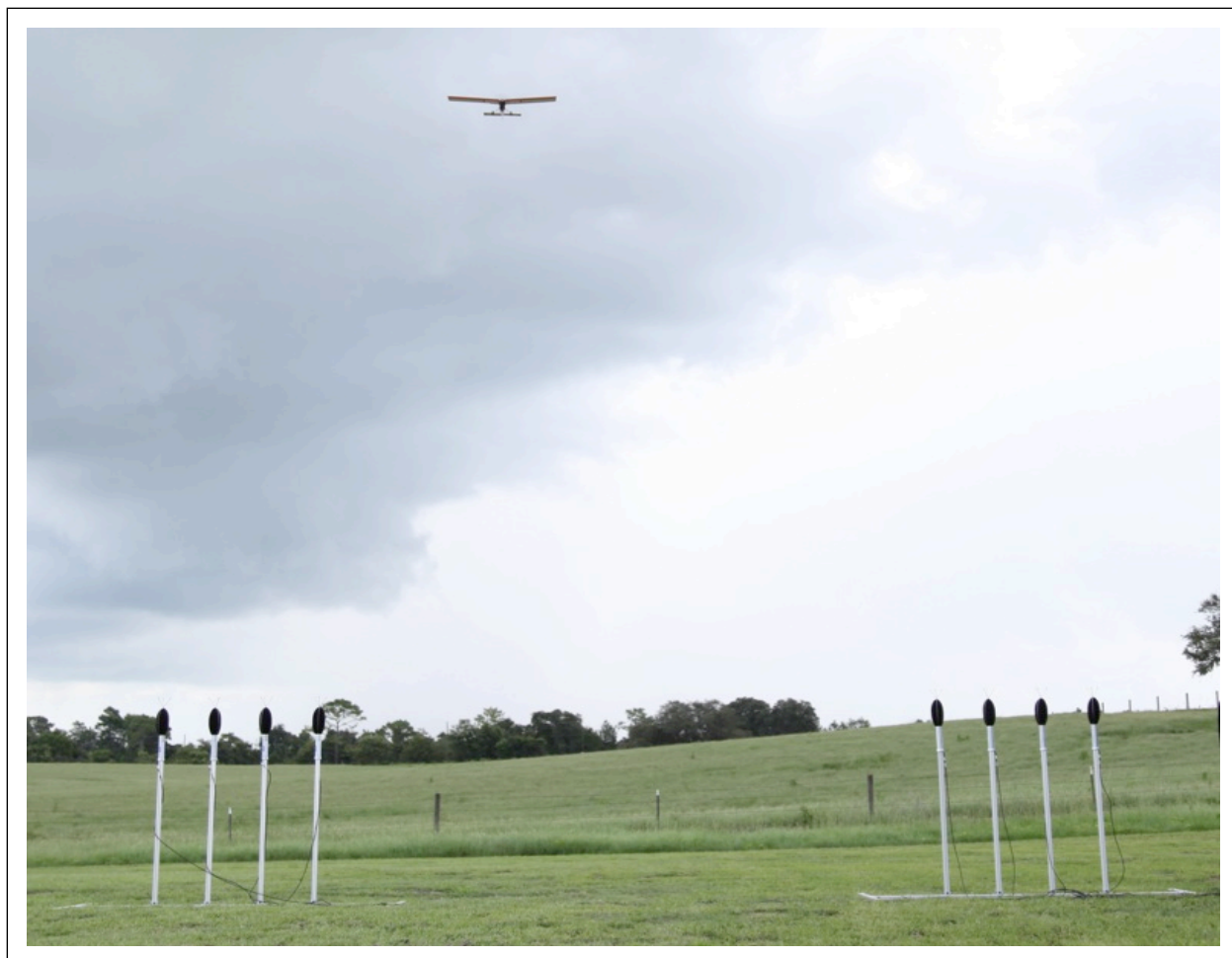
Figure 19. Radio-controlled aircraft test of the ATOM audible acoustic subsystem showing the two microphone nodes.
