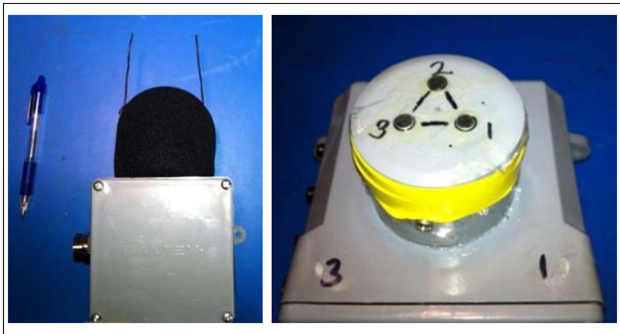
Figure 44. Images of the revised microphone array for the FPSLT deployment.
