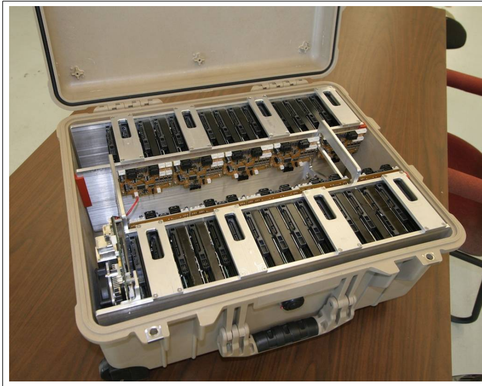
Figure 5. ATOM data storage subsystem.
