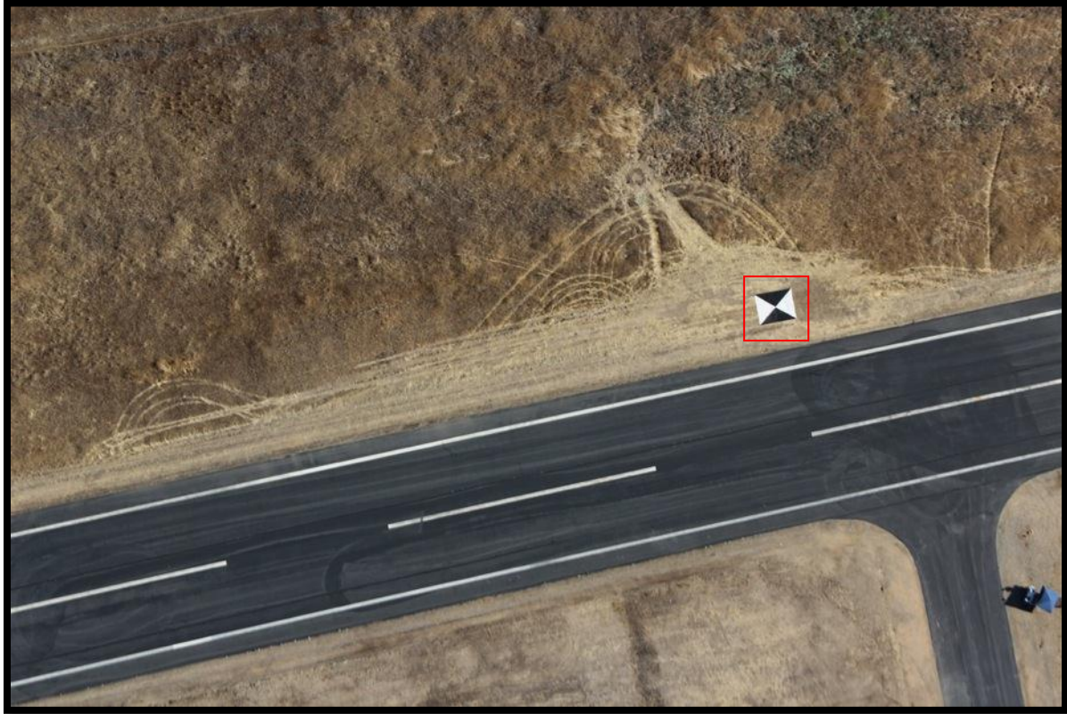
Figure 3–26. Image taken during UAS-based imaging flight tests conducted during the week of 3 October 2011 at Camp Roberts CA, from a flight altitude of 272 m agl. A red box is drawn around a black and white image calibration object, located on the ground just above the runway in the image. An enlargement of this object is shown in Figure 3–27.
