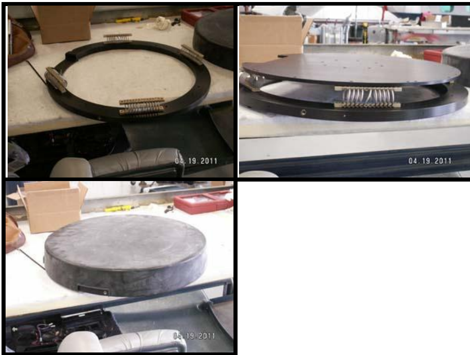
Figure 2–1. Low frequency vibration isolation components mount ring and vibration isolation coils (top left), camera mount plate, isolation coils, and mount ring (top right), and protective cover plate for mount enclosure (bottom) prior to installation on aircraft for Operations House imaging experiments.
