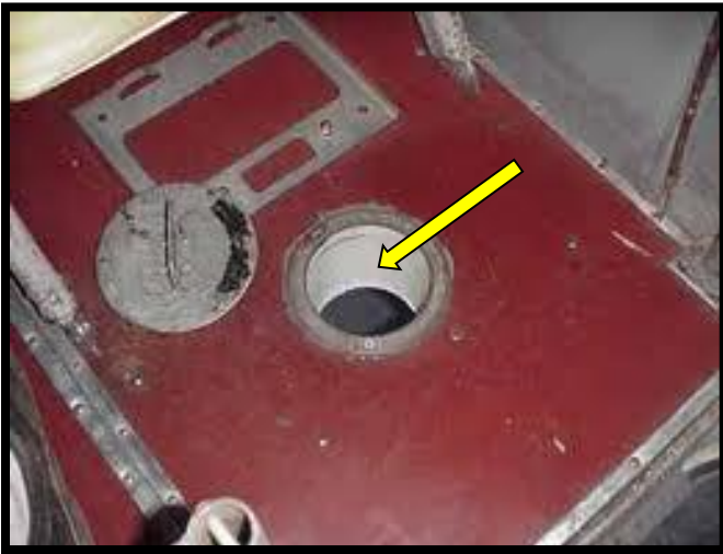
Figure 4–21. Cabin view of a 6-inch diameter tubular type camera port (indicated by the yellow arrow). This type of camera port would not be sufficient for conducting the aerial imaging survey protocols described in this report (see text).
