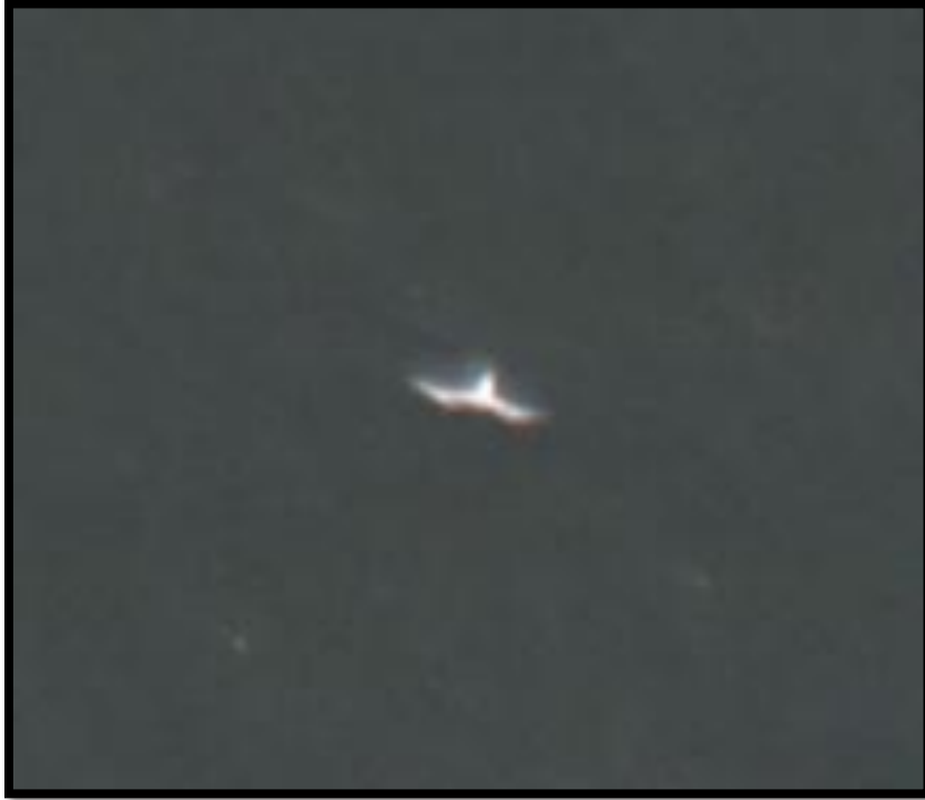
Figure 3–13. Image of a bird from aerial imaging experiments conducted between 10 and 20 May 2011 offshore of Oak Island NC. This image was produced using a gyrostabilized area-scan camera, with imaging parameters otherwise identical to that used in Figure 3–12 above (1,000 m flight altitude and image resolution of 2.5 cm). The increased sharpness of this image compared with Figure 3–12 illustrates the importance of gyroscopic stabilization.
