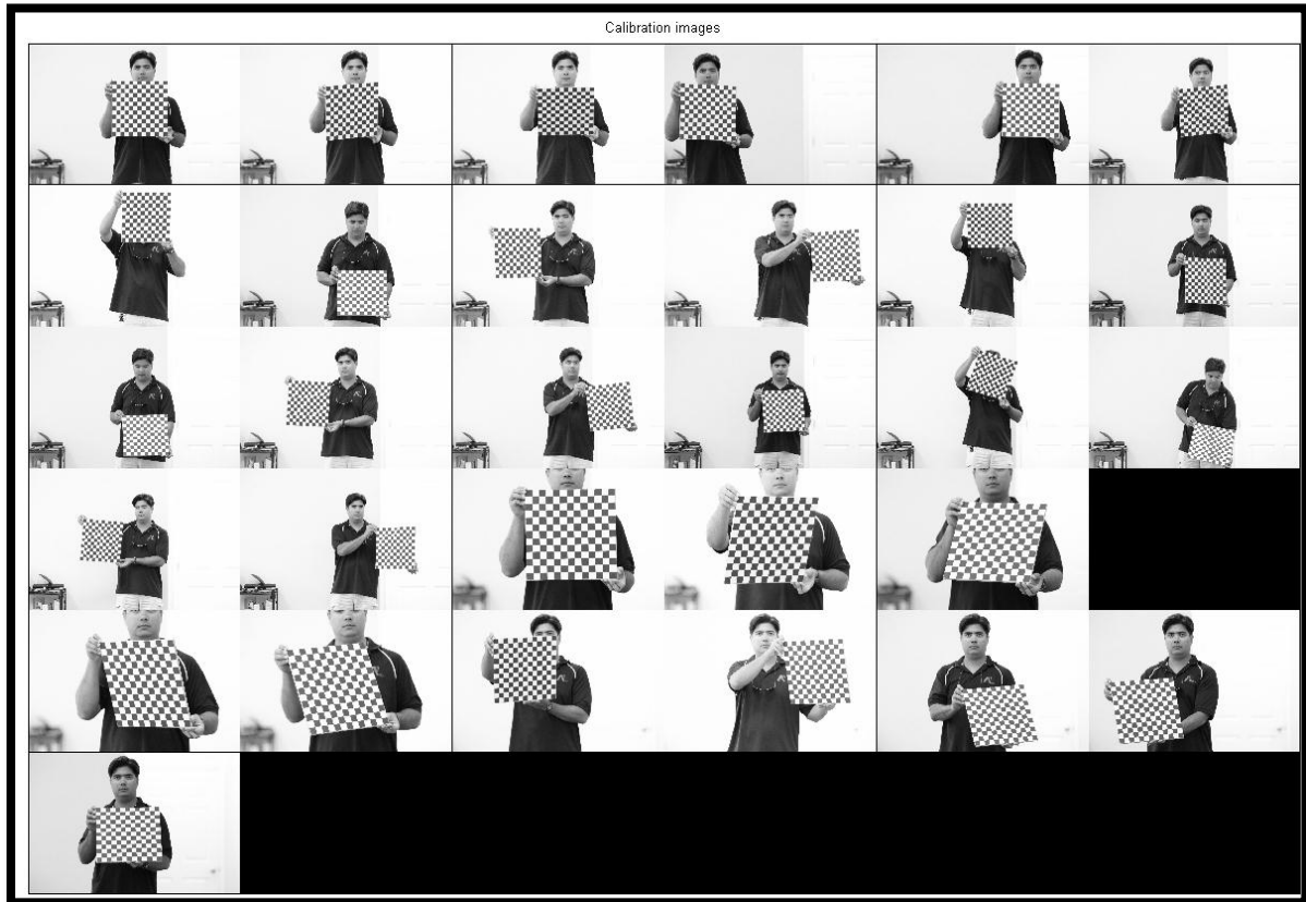
Figure 3–37. Calibration images collected with camera payload for unmanned aircraft system-based imaging system.
