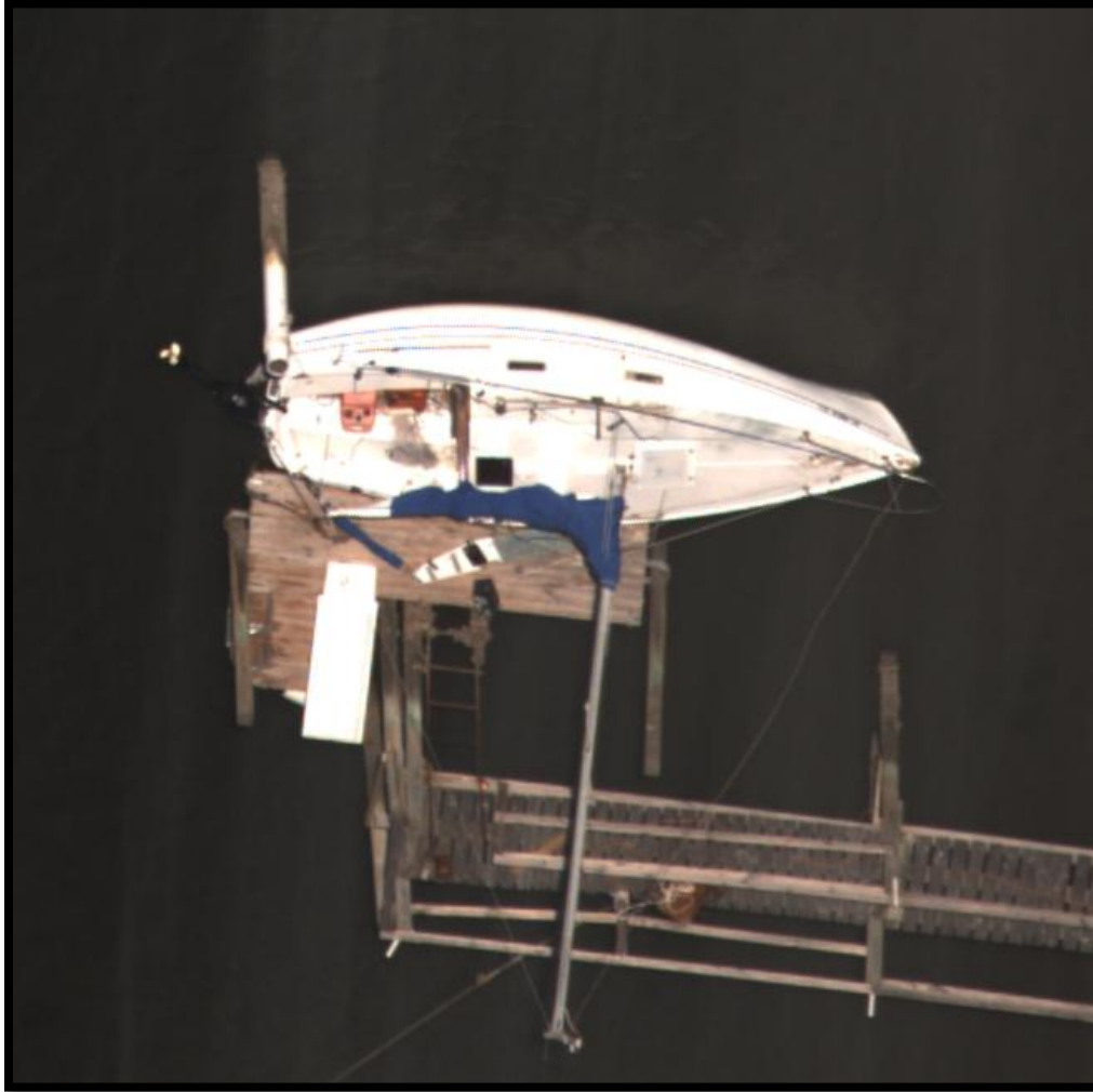
Figure 3–18. Image of the same boat and dock as in Figure 3–17, from aerial imaging experiments conducted between 10 and 20 May 2011 near Oak Island NC. In this image, a shorter (600 mm) focal length lens is used in order to achieve the same image resolution level as in Figure 3–17 (2 cm) at a lower flight altitude (600 m). The increased sharpness of this image relative to Figure 3–17 illustrates the increased image blur that can occur with increased image magnification (see text).
