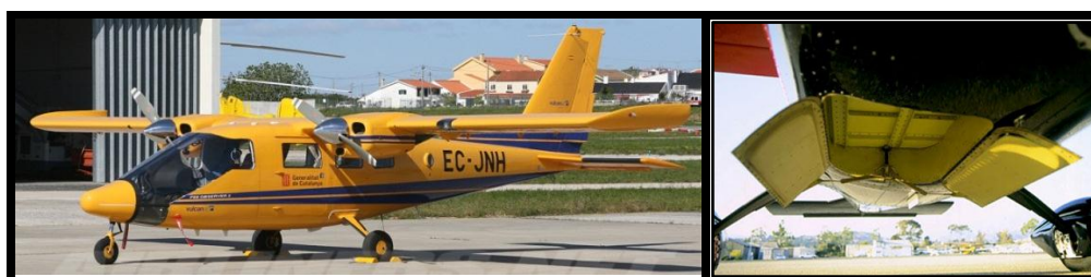
Figure 4–33. Aircraft selected for development of the regional scale protocol for offshore high-resolution aerial wildlife imaging surveys: the Vulcanair P68 Observer 2 (left) and its belly hatch (right).
