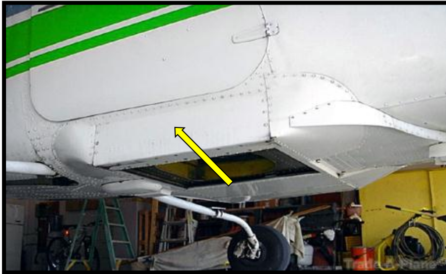
Figure 4–20. Example of a typical camera port in the belly of a small aircraft. The yellow area, internal to the camera hatch, represents the distance between the internal floor of the cabin and the external skin of the aircraft, which can constrain available camera angles (see text).
