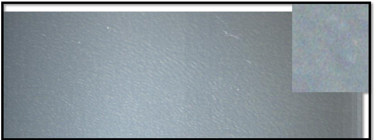
Figure 3–15. Image of water from aerial imaging experiments conducted 10 to 20 May 2011 offshore of Oak Island NC with a digitally magnified portion of the image shown in the inset in the upper right. This image was taken during relatively low light conditions in the early evening. The reduced image quality of this image compared with Figure 3–14 can be seen in the graininess and color distortion visible in the inset (see text).
