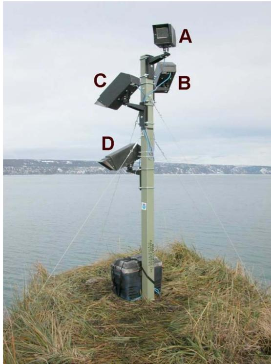
**Figure 2.** Photograph of time-lapse camera systems deployed at Aurora Rock in Kachemak Bay. Four cameras (A – D), with time-lapse controllers, were attached to one support post anchored with guy wires. The cameras were aimed to ensure complete coverage.
