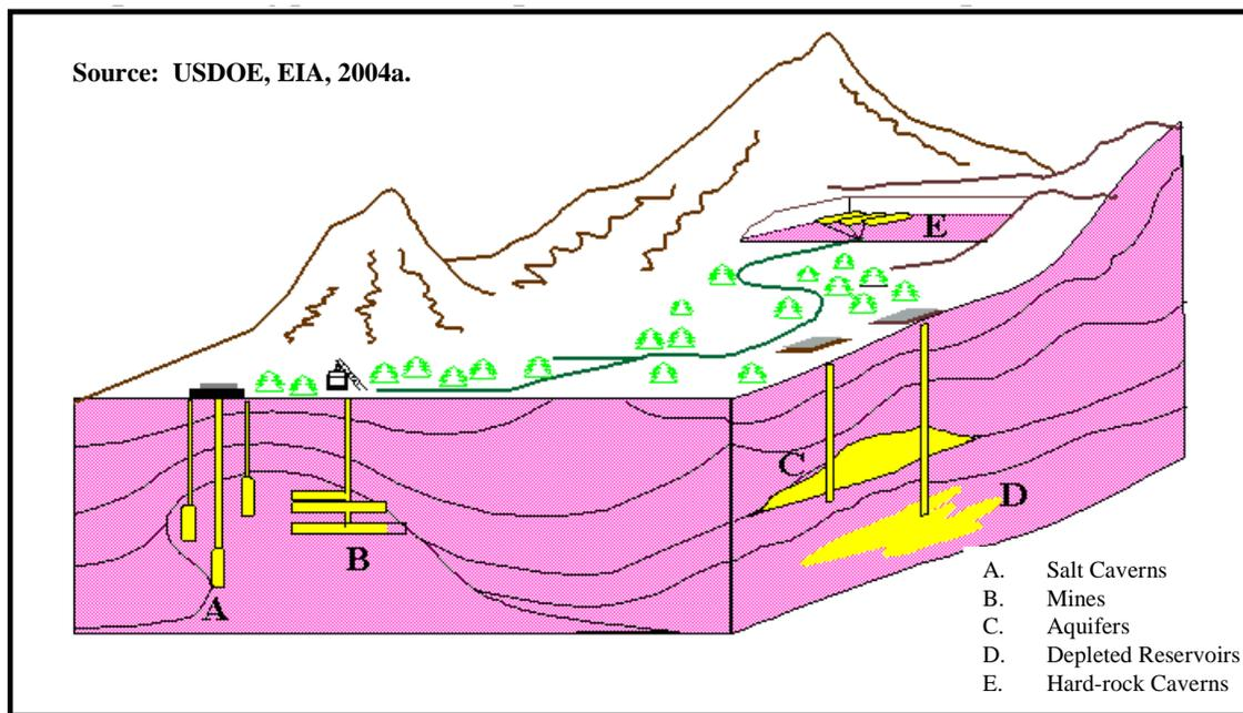
**Figure 90. Types of underground natural gas storage facilities.**
