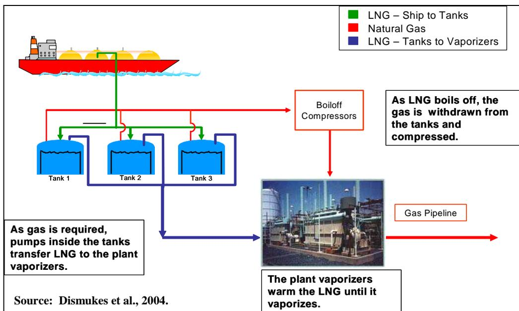
**Figure 69. Receiving terminal – LNG gas flow.**
