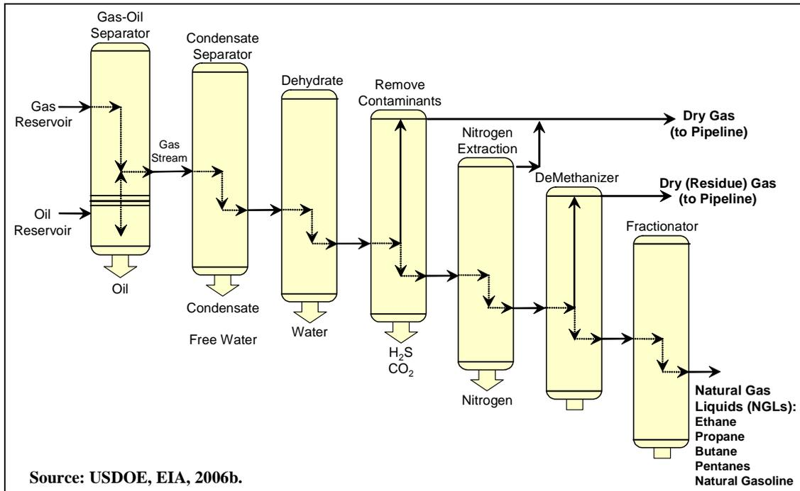
**Figure 84. General natural gas processing schematic.**
