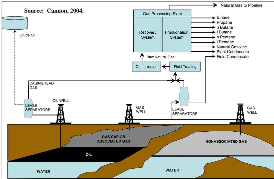
**Figure 83. Natural gas processing.**
