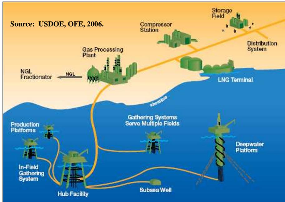
**Figure 73. GOM gas supply schematic.**
