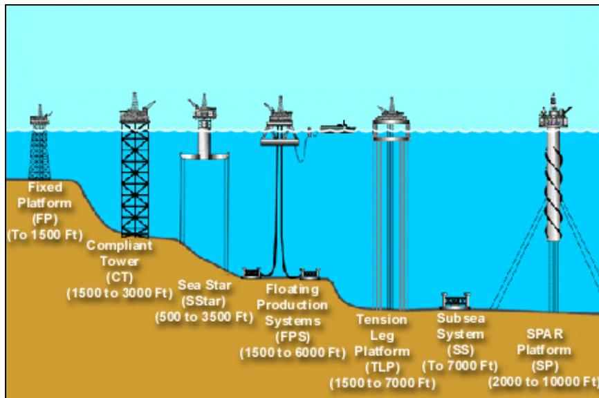
**Figure 4. Offshore drilling platforms.**
