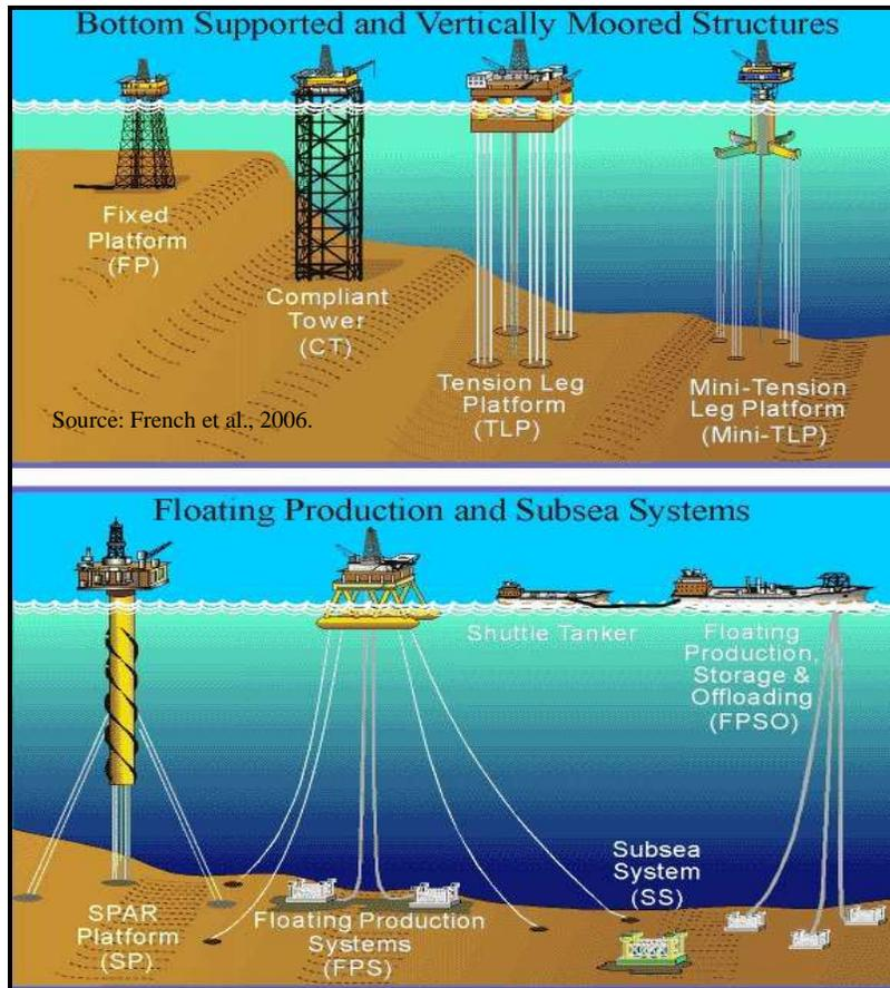
**Figure 9. Permanent production systems on the GOM OCS.**
