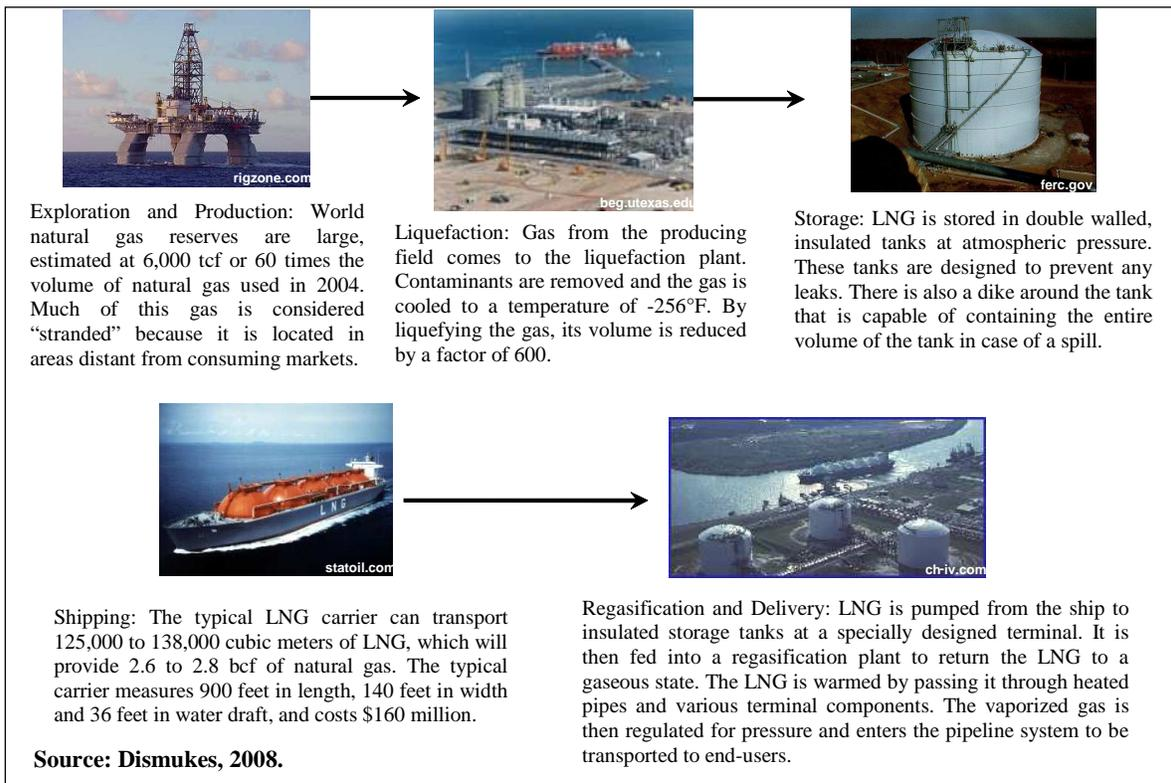
**Figure 68. LNG schematic – production to end-user.**
