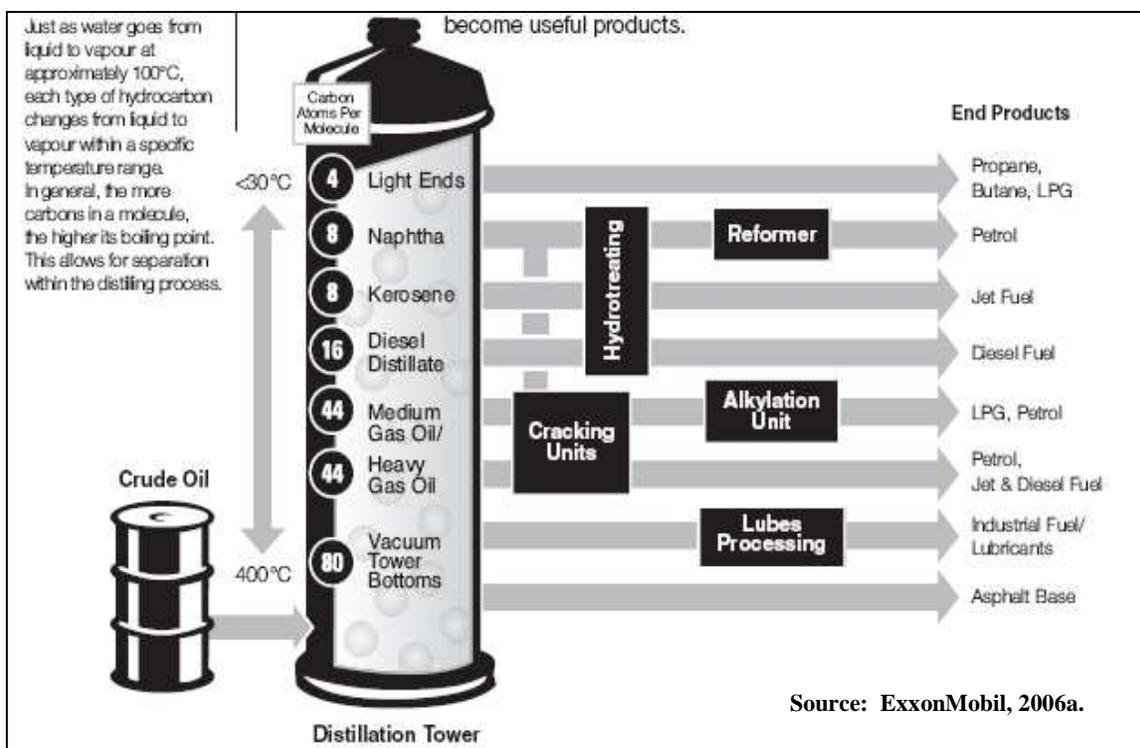
**Figure 98. Distillation process.**
