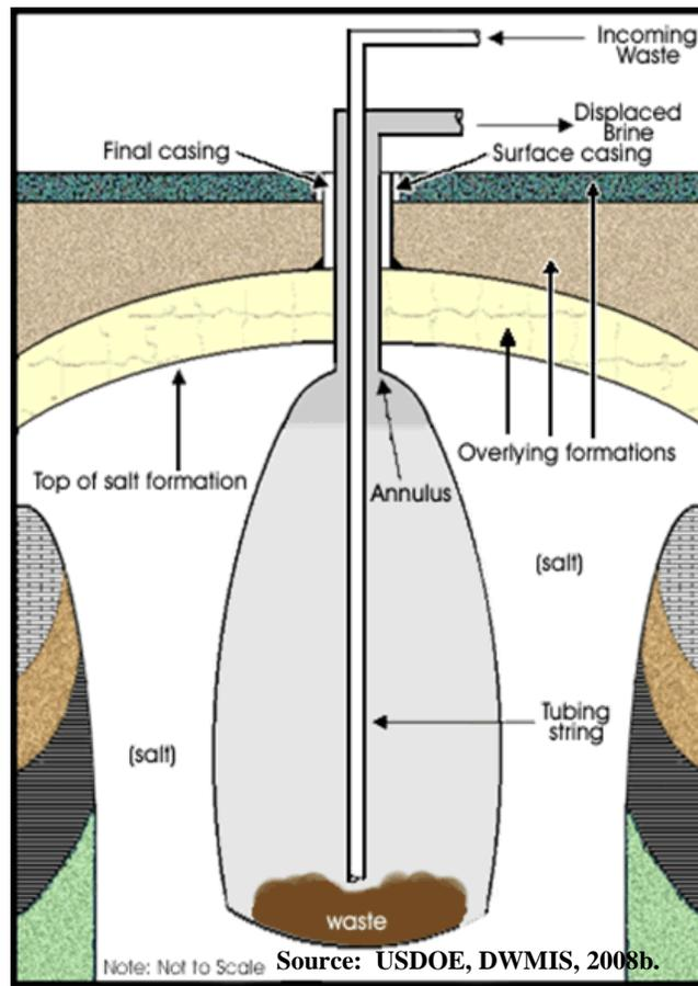
**Figure 38. Schematic of a cavern in domal salt.**
