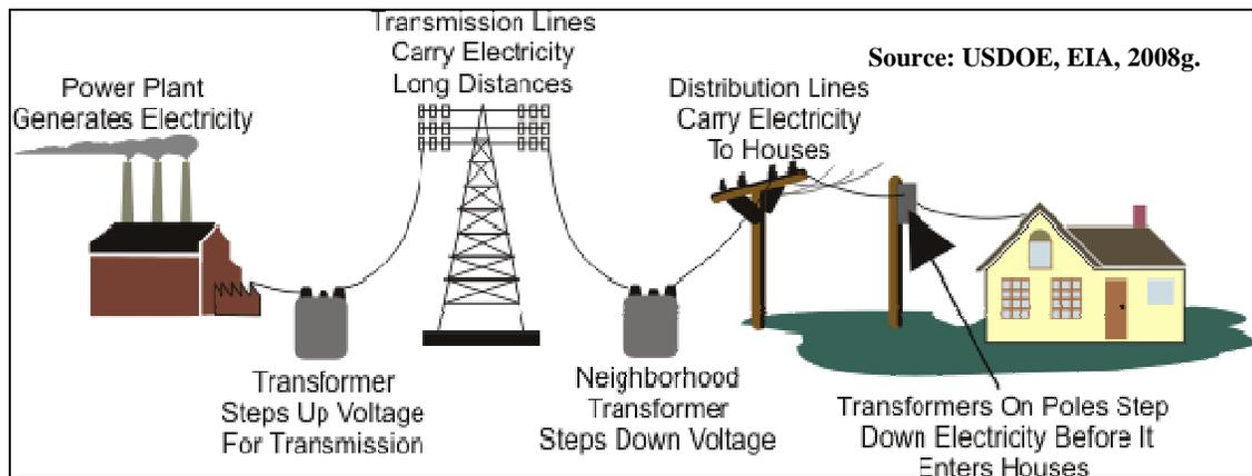
**Figure 126. Power generation, transmission, and distribution.**
