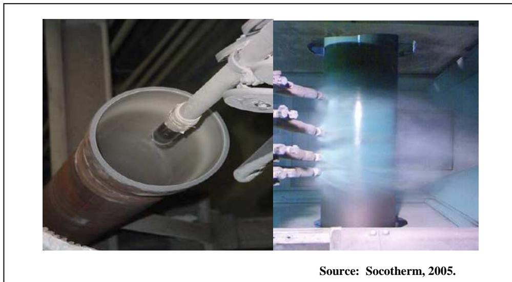
**Figure 60. Internal coating called Tubokote and external coating with fusion bonded epoxy called Powderkote.**
