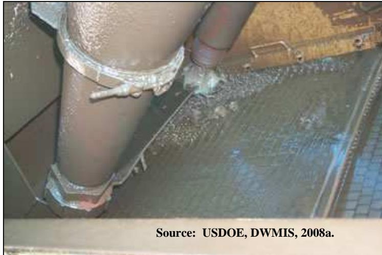
**Figure 37. Shale shaker.**
