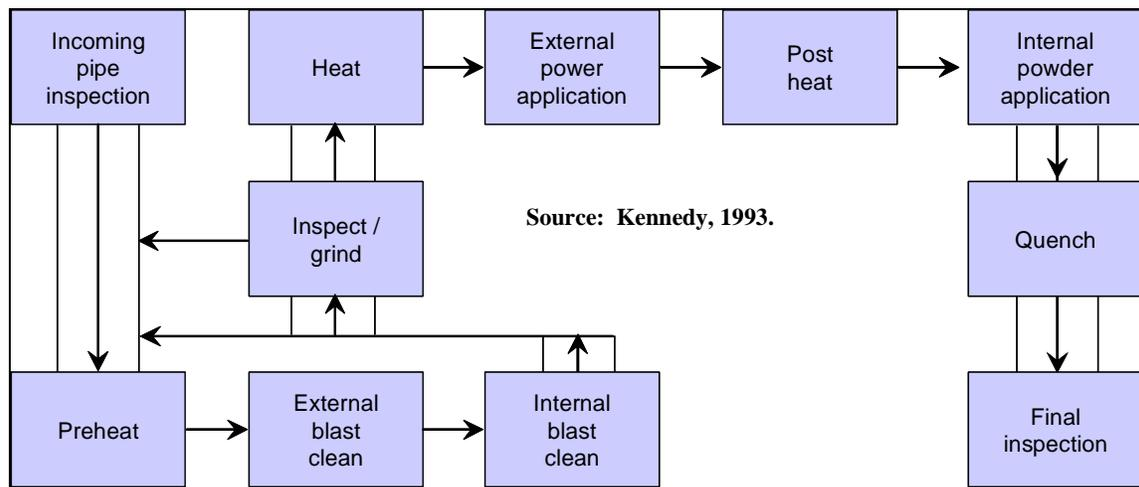
**Figure 61. External/internal fusion bonded epoxy coating plant.**
