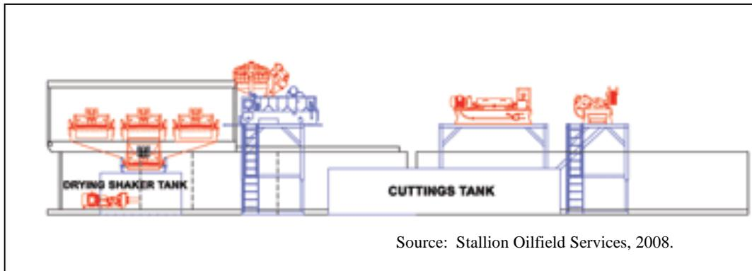
**Figure 41. Stallion’s design of their close loop mud system.**
