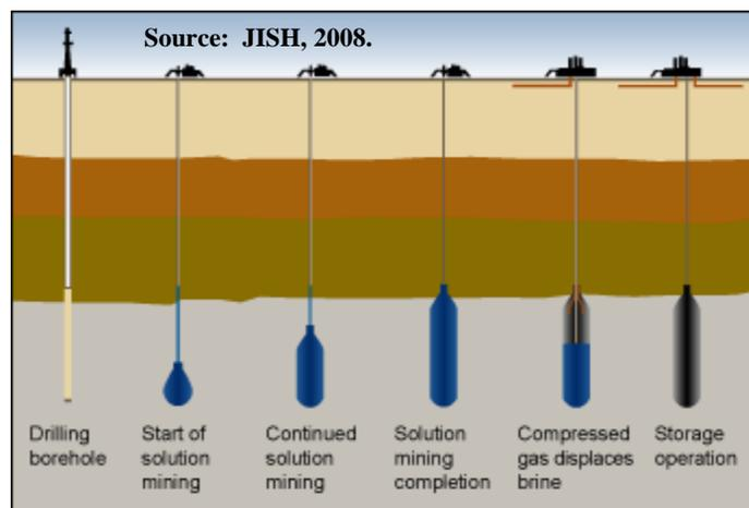
**Figure 92. Solution mining process.**
