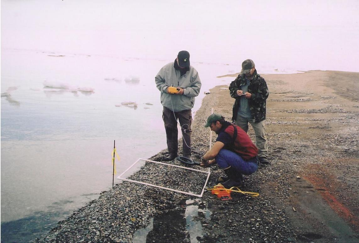
**Plate 6. Scanning the seaward beach for PIT-tagged gravel, adjacent to site 1A marker stake, using a rectangle grid sampling pattern . Note the band of concentrated streak of red fluorescent-dyed sand along the beach stranded at the high-tide mark. The streak was elongated mostly to the west of the stake.**
