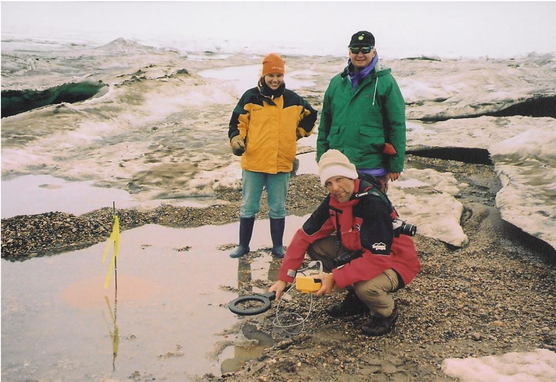
**Plate 5. Scanning with the Reader for and locating PIT-tagged gravels on the seaward beach of Narwhal Island by Bill Streever of British Petroleum Exploration, Inc., and John Kelley and Mindy Krzykowski of the University of Alaska Fairbanks. Note the clump of red dyed-sand submerged in subtidal water and adjacent to the marker stake.**
