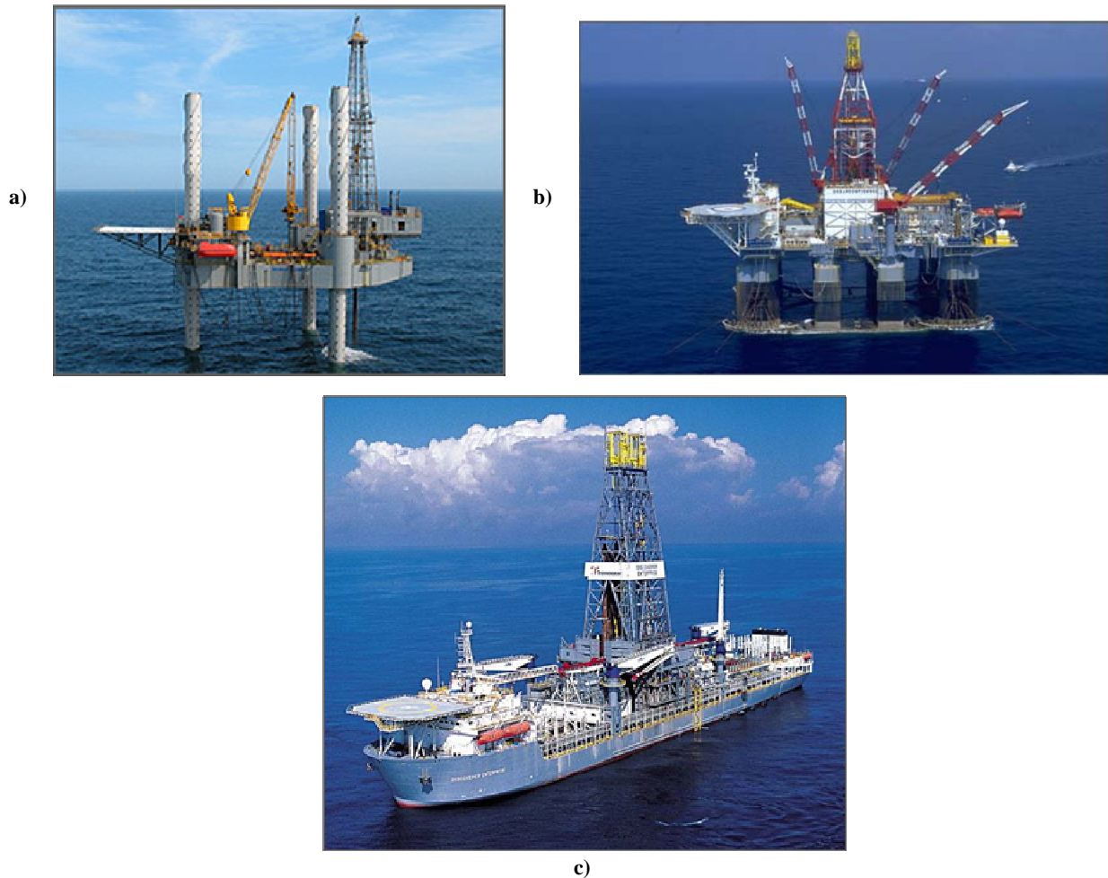
Figure D-1. Examples of mobile offshore drilling units: a) jack-up; b) semi-submersible; and c) drillship. Public domain images from the U.S. Department of Energy (jack-up; courtesy of Blake Offshore LLC; posted at www.apps1.eere.energy.gov ), Baud et al. (2002; semi-submersible; courtesy of Diamond Offshore Drilling, Inc.), and NOAA (drillship; courtesy of Transocean; posted at www.noaa.gov ).
