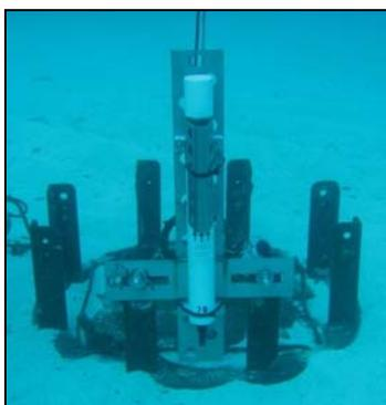
Figure 2.10.4. An image of the Sea-Bird MicroCAT deployed at the EFGB.
