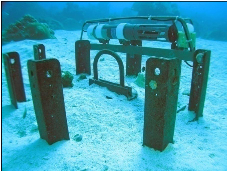
Figure 2.10.2. An image of the YSI datasonde deployed at the FGB. Photograph courtesy of FGBNMS.
