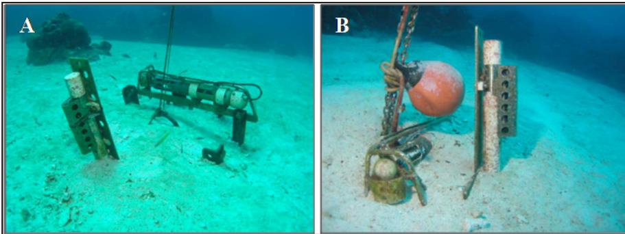
Figure 3.6.4. YSI and Seabird units partially buried in sand at the (A) EFGB and (B) WFGB long-term monitoring sites in October 2008. Photographs from Hickerson (2008b).
