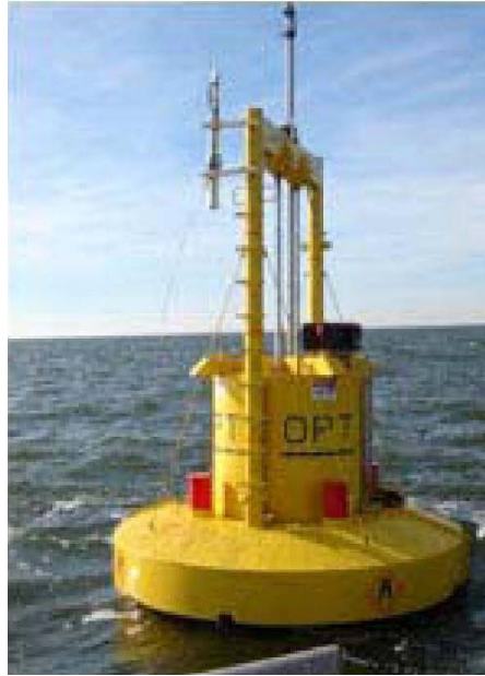
Figure 3-4: An example of a buoy-type wave energy technology.
