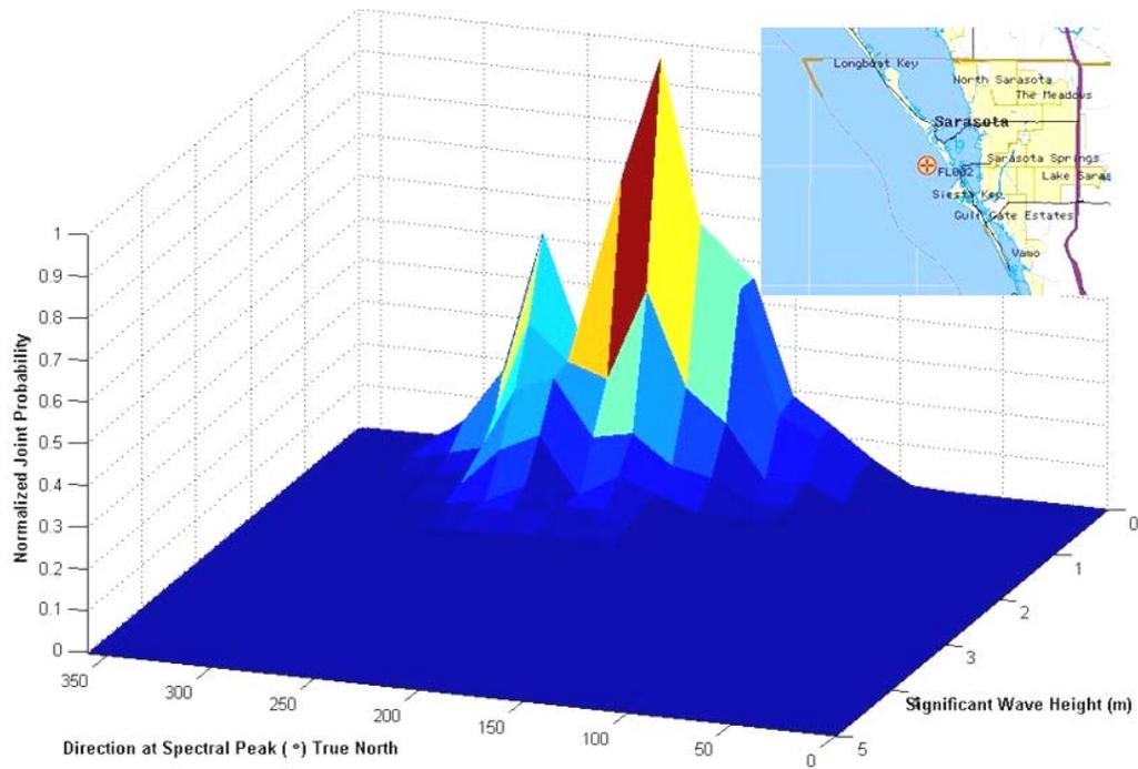
Figure 2-29. Joint probability of significant wave height and peak direction for wave data measured in 7 m of water off Sarasota Beach between 1993 and 1996. Inset shows the approximate location of the directional wave gauge.
