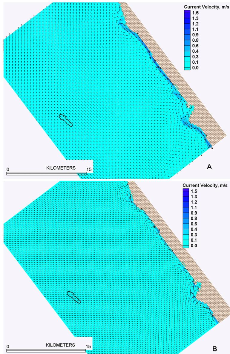
**Figure 4-41. Predicted velocity field generated from the Siesta Shoal model during the February 1998 winter storm (A) and Tropical Storm Harvey in September 1999 (B). Stronger currents in the nearshore zone were produced by breaking waves.**
