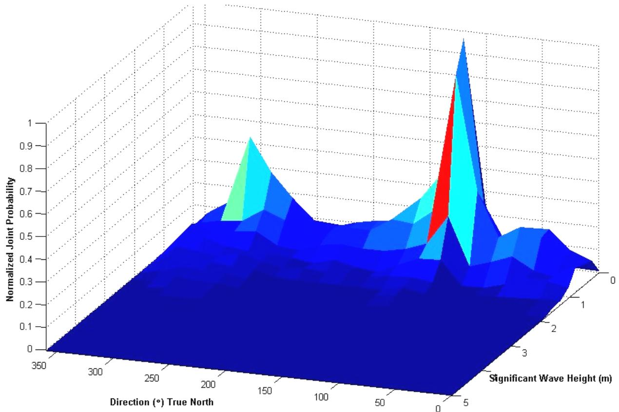
**Figure 2-26. Joint probability between significant wave height and peak direction at WIS Station 290. Hind cast time period is 1995-1999.**
