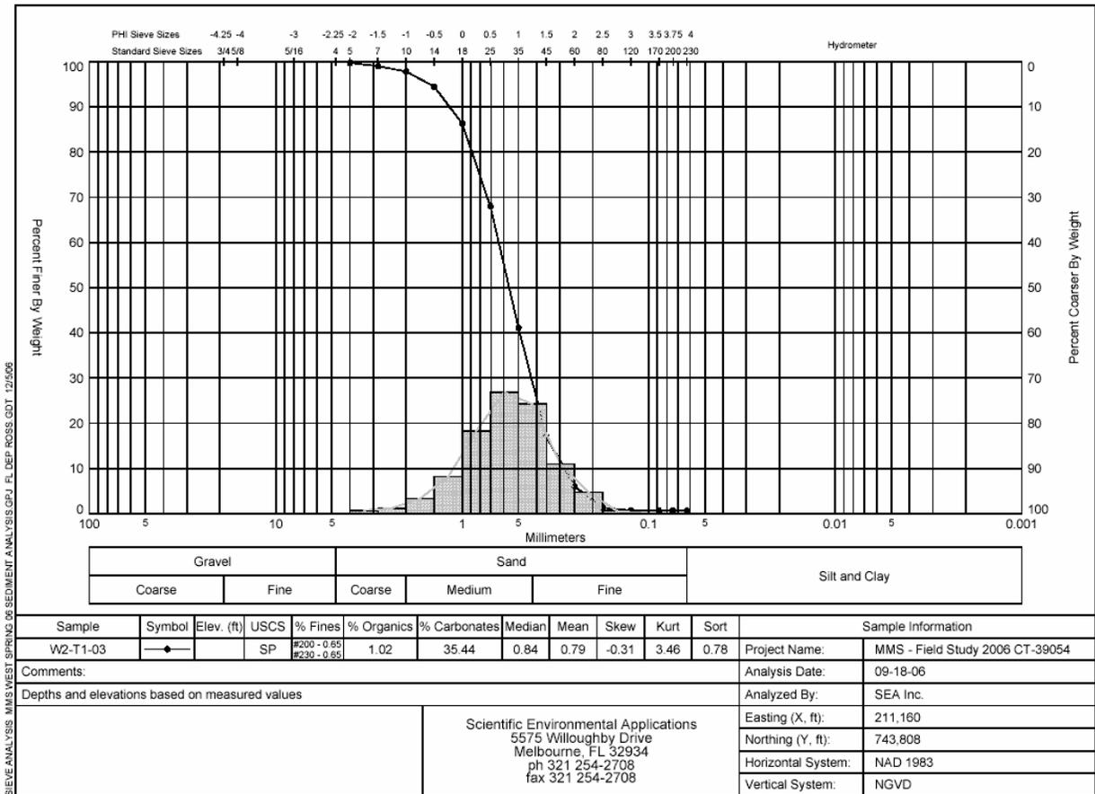
**Figure 3-8. 2006 Sample W2-T1-03 from the crest of the T1 Shoal. Sample texture is predominantly medium sand, some fine sand and a coarse sand fraction of shell fragments.**
