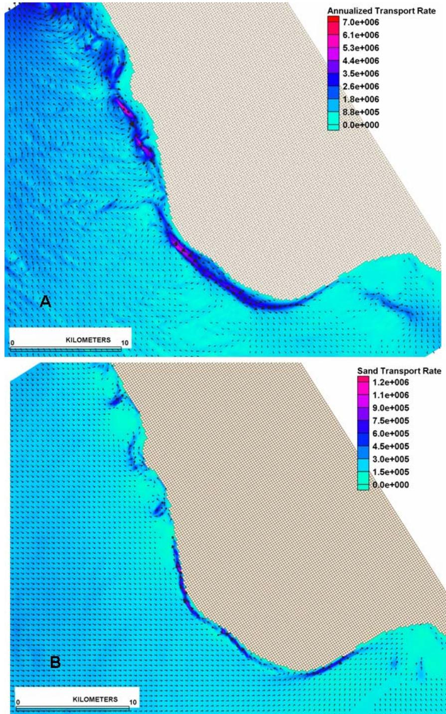
**Figure 4-19. Sand transport rates (annualized) for the T1/T2 model during the 1998 winter storm (A) and during Tropical Storm Harvey in September 1999 (B). Higher transport rates in the littoral zone result from wave driven longshore currents.**
