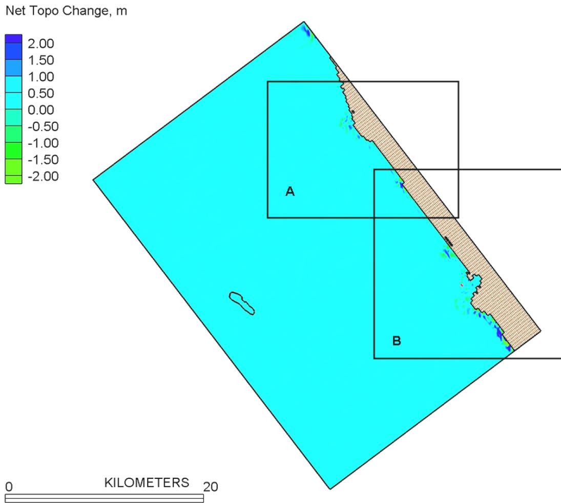
**Figure 4-47. Location of two panels shown in Figure 4-48 (Panels A and B) providing the details of net topographic change after 2-years of simulation under Case 5 for Siesta Shoal (large borrow cut).**
