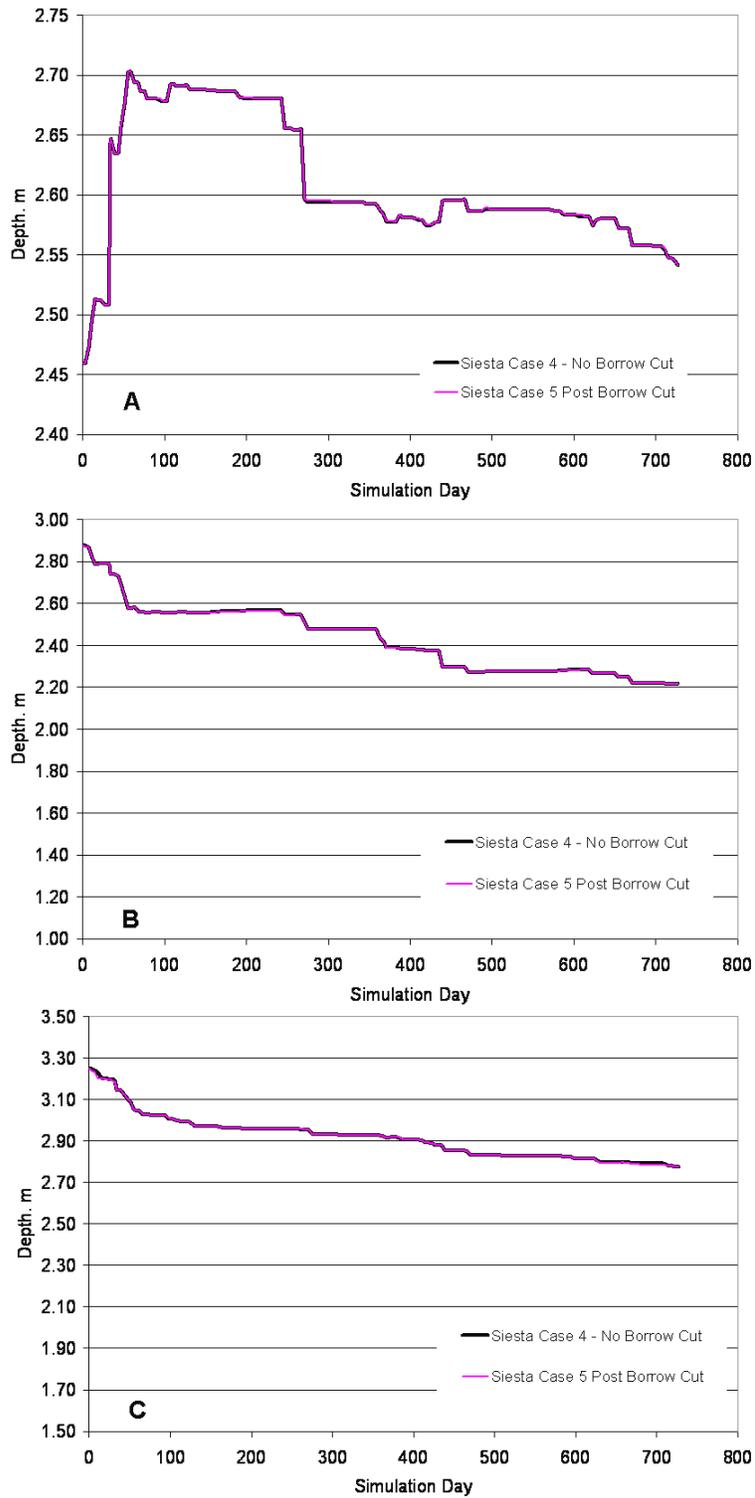
**Figure 4-49. Comparison of predicted topographic evolution over the two-year model simulation on the upper shoreface at Stations 20, 30, and 45. Location of the observation stations is shown in Figure 4-43.**
