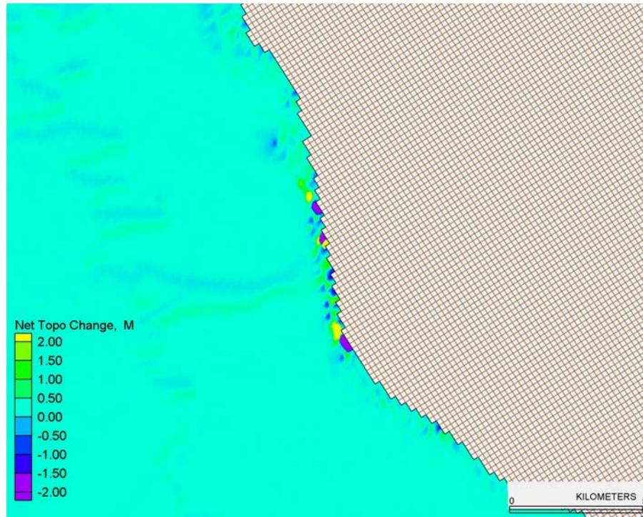
Figure 4-27. Details from Panel B of Figure 4-25 showing the T1/T2 model predicted net change after two years of simulation under Case 1 (No borrow cut).
