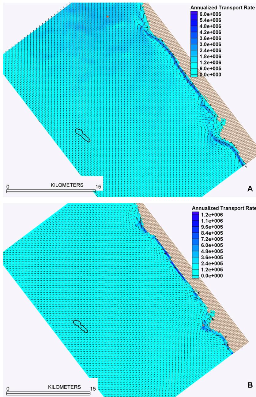
**Figure 4-42. Annualized predicted sand transport rates generated from the Siesta Shoal model during the February 1998 winter storm (A) and during Tropical Storm Harvey in September 1999 (B). Higher transport in the littoral zone results from wave-driven longshore currents. Units are in cubic yards per year.**
