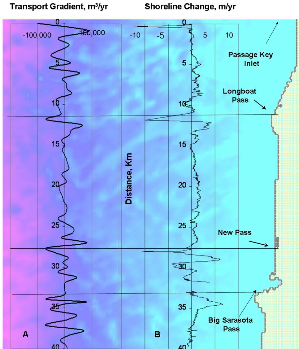
**Figure 4-46. Comparison of Siesta Shoal model predicted gradients of littoral sand transport (A) and measured shoreline change rates between 1976 and 2001 (B) compiled by the USGS.**
