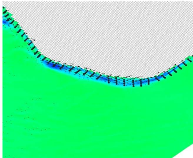
**Figure 4-21. Example of T1/T2 model numerical observation stations (Stations 20 – 50) positioned in the littoral zone of Sanibel Island to capture wave generated longshore currents and sand transport.**
