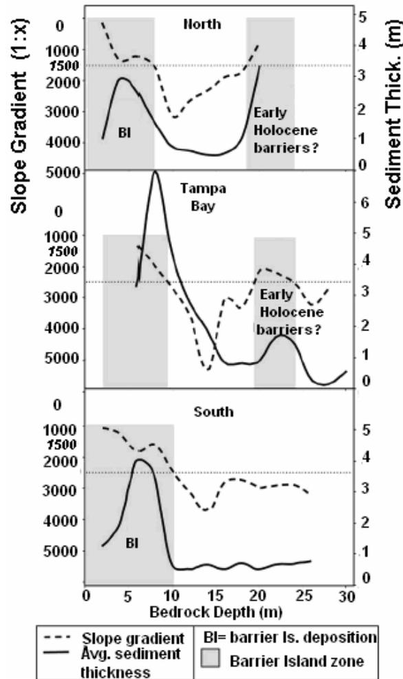
**Figure 2-11. Plots depict relationship of Holocene sediment thickness to slope gradients for the three sections of the west Florida inner continental shelf. Slope gradients greater than 1:1500 correlate to thicker accumulations known, or inferred, to be barrier-island systems (from Locker et al., 2003).**
