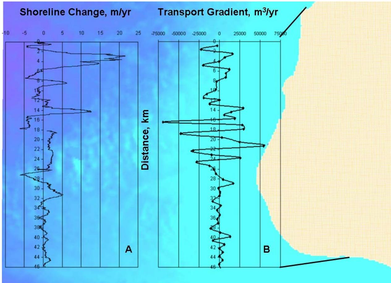
**Figure 4-23. Comparison of measured shoreline change rates from the T1/T2 model between 1976 and 2001 (A) and predicted gradients of net longshore sand transport.**
