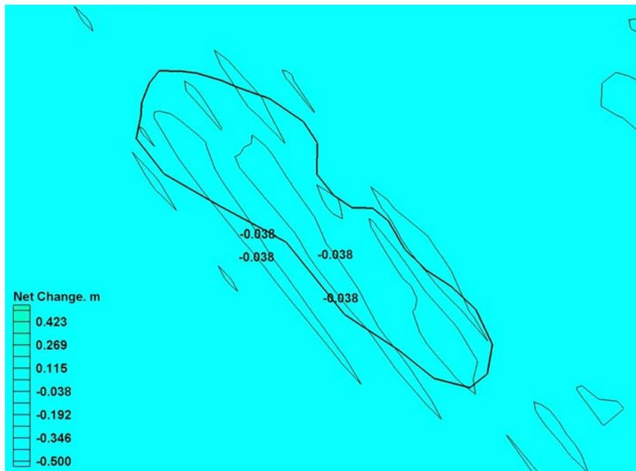
Figure 4-54. Predicted net topographic change over the Siesta Shoal features in the existing topography after two year of model simulation (Case 4, Table 4-1).
