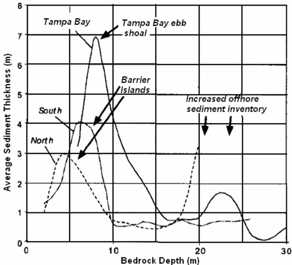
Figure 2-10. Plot of average Holocene sediment thickness versus bedrock depth, which marks the transgressive surface on which Holocene and modern sediments are deposited (from Locker et al., 2003).
