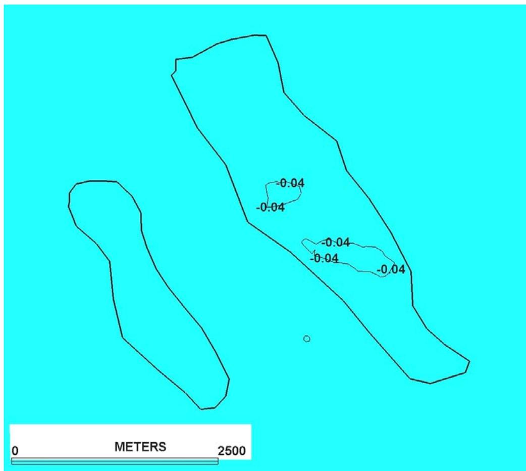
**Figure 4-51. Predicted topographic change over the T1/T2 Shoal features after two years of model simulation under the without a borrow cut (Case 1, Table 4-1).**
