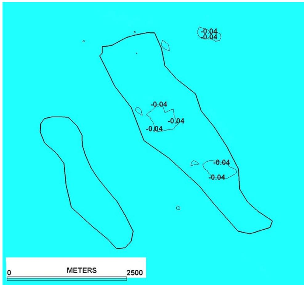
**Figure 4-52. Predicted topographic change over the T1/T2 Shoal features after two years of model simulation with placement of the existing borrow cut at the north end of T1 (Case 2, Table 4-1).**
