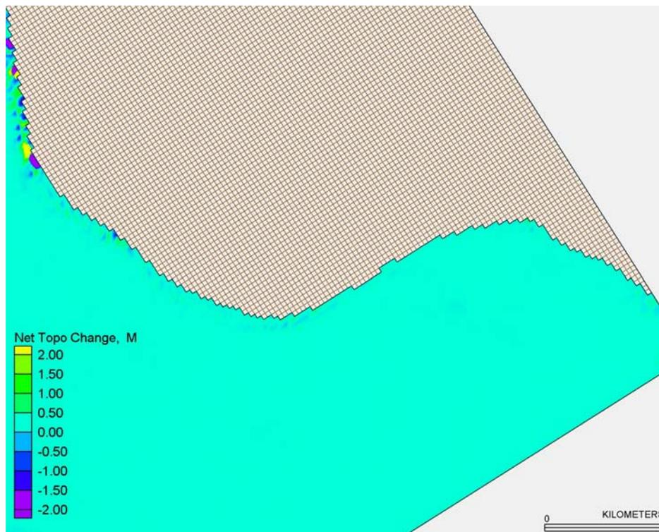
Figure 4-28. Details from Panel C of Figure 4-25 showing the T1/T2 model predicted net change after two years of simulation under Case 3 (Multiple Borrow Cuts).
