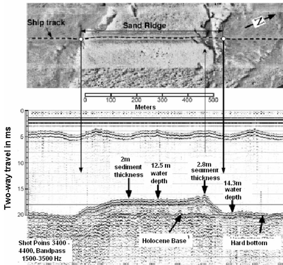
Figure 2-8. Side scan sonar and seismic cross-section records from a sand ridge located about 15 miles offshore of Indian Rocks Beach. Water depth at the crest of the ridge is about 40 ft (12 m) (from Howd et al., 2003).
