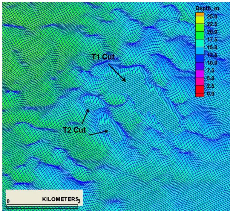
Figure 4-10. Perspective views from the southwest showing the extensive hypothetical borrow cuts in the T1/T2 shoal system that would remove approximately 2.3 million cubic meters of sand.
