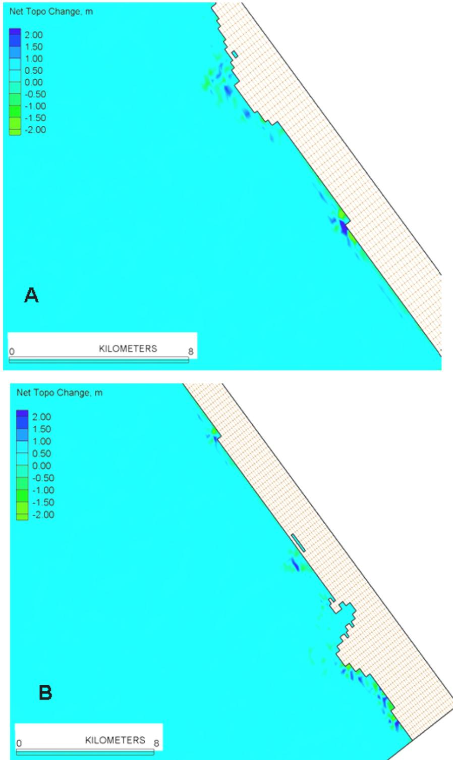
**Figure 4-48. Details from Panels A and B in Figure 4-47 showing the predicted net change after two years of model simulation under Siesta Shoal Case 5.**
