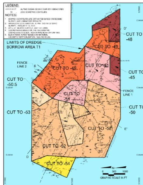
**Figure 4-8. Permit design of the borrow cuts at the north end of the T1 Shoal (from CPE, 2005). (Note position of north arrow).**
