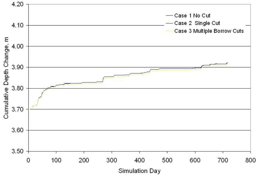
**Figure 4-30. Comparison of predicted topographic change on the upper shoreface at Station 13 over the two-year T1/T2 model simulation. Location of station is shown in Figure 4-26.**
