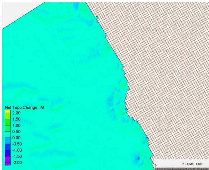
**Figure 4-26.** Details from Panel A of Figure 4-25 showing the T1/T2 model predicted net change after two years of simulation under Case 2 (single borrow cut).
