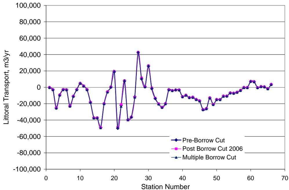
**Figure 4-22. Predicted annual longshore sand transport from the T1/T2 model based on a 2-year model simulation. The results for Case 1 (Pre-Borrow Cut), Case 2 (Post Borrow Cut 2006) and Case 3 (Multiple Borrow Cuts) are shown. Positive values indicate net transport to the north and negative values indicate net transport to the south. Locations of the recording stations in the model are shown in Figure 4-20.**
