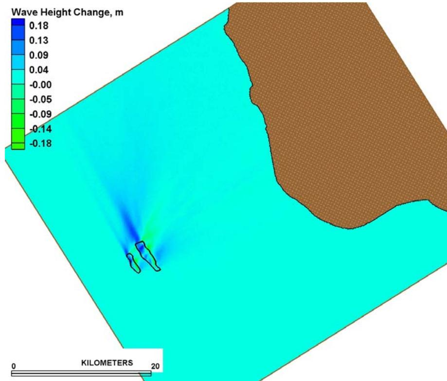
**Figure 4-16. Predicted change in wave height patterns after the T1/T2 topography is modified by multiple borrow cuts. Wave conditions in the simulations are associated with the passage of Tropical Storm Harvey in September of 1999.**
