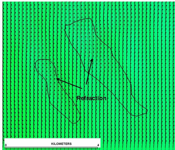
Figure 4-15. Predicted refraction pattern as waves move northward and diagonally across the T1/T2 Shoals during Tropical Storm Harvey in September 1999.
