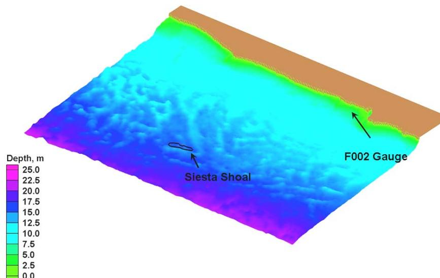
**Figure 4-5. Perspective view from the southwest showing the location of Siesta Shoal and the location of the USACE F002 direction wave gauge used to verify wave model results. Vertical exaggeration is 200x.**
