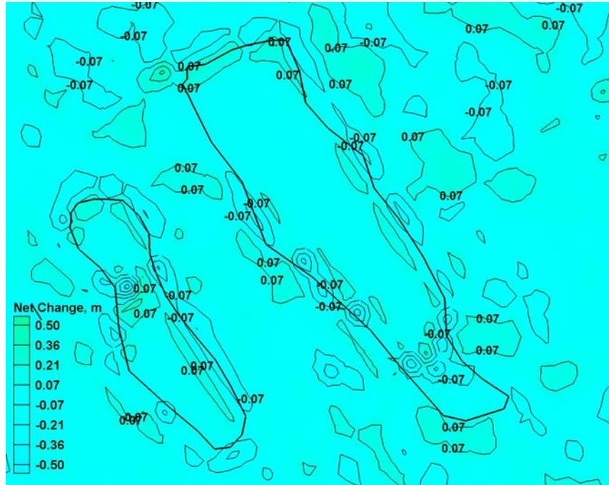
Figure 4-53. Predicted topographic change over the T1/T2 Shoal features after two years of model simulation with placement of the cumulative borrow cut over T1 and T2 (Case 3, Table 4-1).
