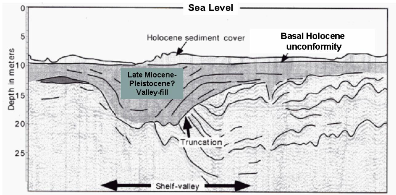
**Figure 2-4.** An interpretation of shelf valley fill sequence from a sub-bottom seismic cross-section. The seismic signature of the overlying thin Holocene sediments is nearly indistinguishable from the Miocene to Pleistocene sections below (from Locker et al., 2003).
