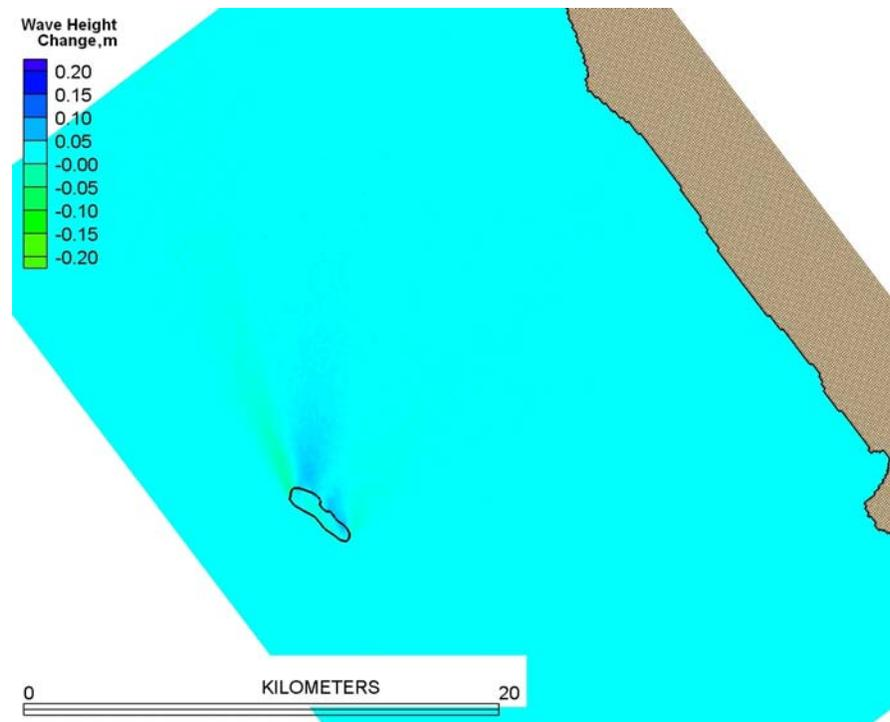
**Figure 4-40. Predicted change in wave height patterns after the Siesta Shoal topography was modified by a large borrow cut (see Figure 4-32). Wave conditions in the simulations are associated with the passage of Tropical Storm Harvey in September of 1999.**
