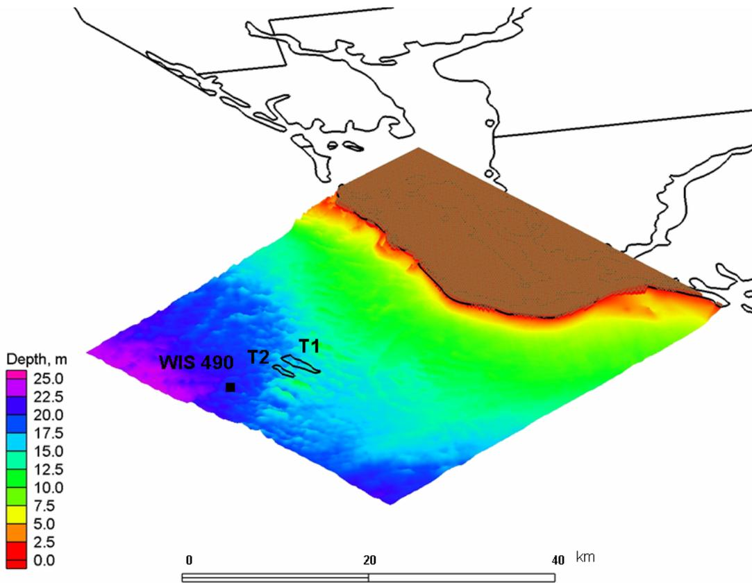
Figure 4-3. Location and bottom topography near the T1/T2 Shoals system. WIS station 490 is shown at the seaward boundary of the model domain.
