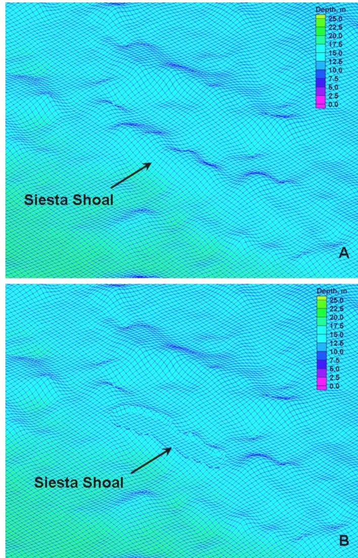
**Figure 4-35. Representation of Siesta Shoal topography in the model grid for Case 4 before borrow cuts (Panel A) and for Case 5 after multiple borrow cuts (Panel B).**
