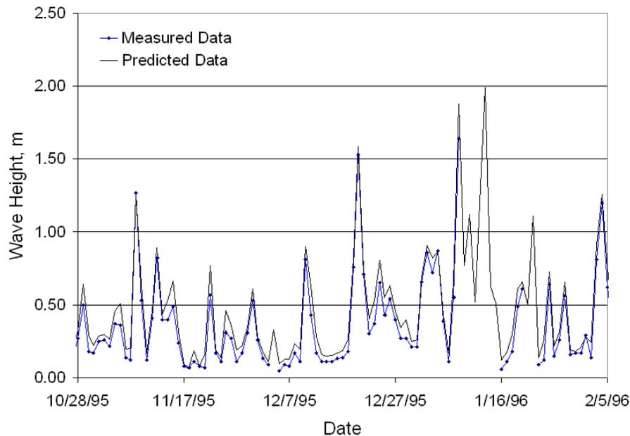
**Figure 4-7. Details of the comparison of predicted and measured wave height data at ERDC Station F002 between October 1995 and February 1996.**
