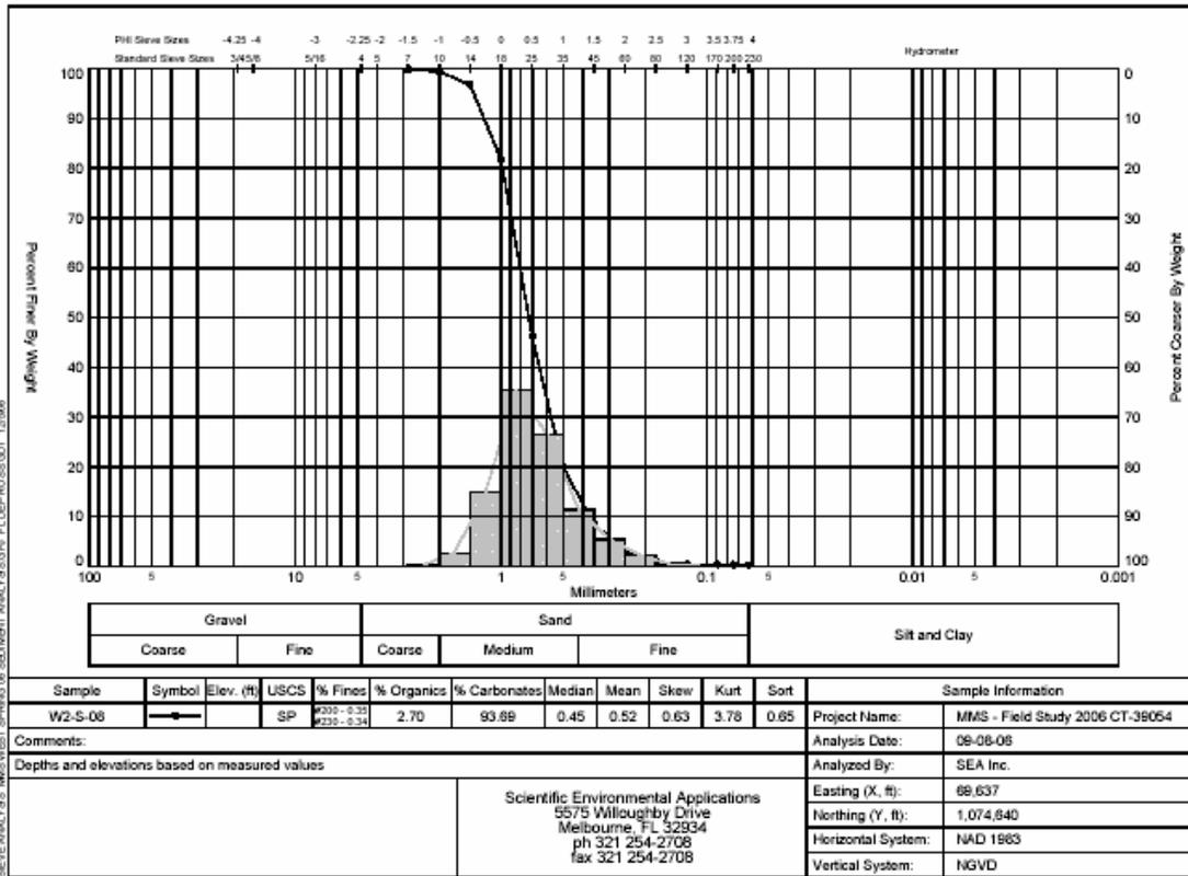
Figure 3-9 Grain size frequency distribution of June 2006 Sample W2-S-08 from the crest of Siesta Shoal. Dominant texture is in the medium sand range compared to the fine sand of samples off the shoal or from the lower flank areas.
