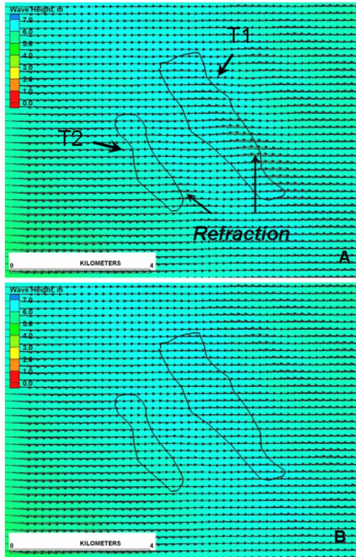
**Figure 4-12. Wave refraction of the T1/T2 Shoals apparent over the pre-borrow cut topography (A) during an extreme wave event. Predicted refraction is minimal during the same event over the post borrow topography (B) that includes large cuts in both shoals (see Figure 4-10).**
