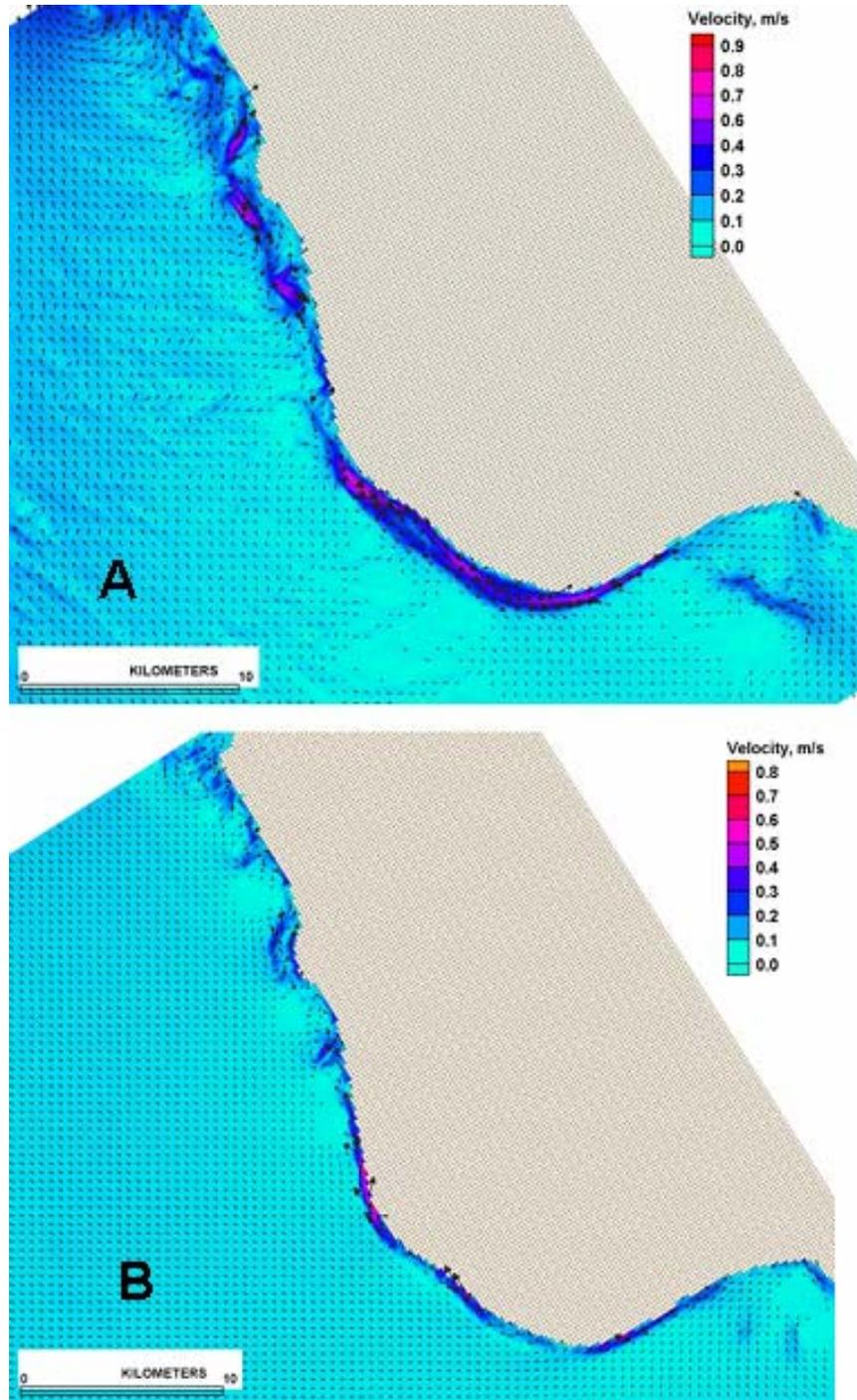
**Figure 4-18. Details of predicted littoral zone longshore currents for the T1/T2 model generated by breaking waves for the Winter Storm of 1998 (A) and Tropical Storm Harvey in September 1999 (B).**
