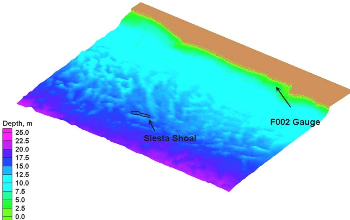
**Figure 4-34. Perspective view from the southwest showing the location of Siesta Shoal on the model domain and the location of the USACE F002 direction wave gauge used to verify wave model results. Vertical exaggeration is 200x.**
