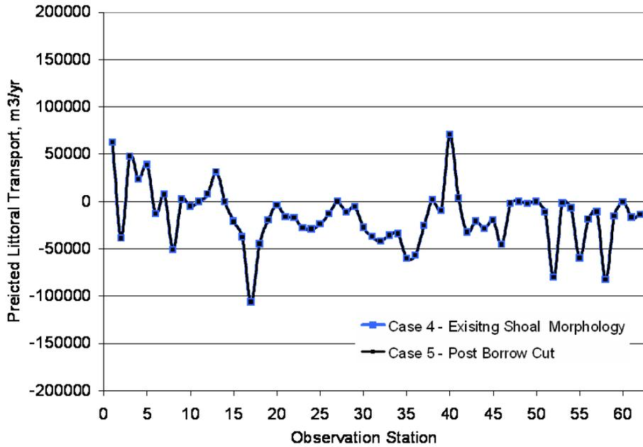
Figure 4-44. Predicted annual littoral sand transport from the Siesta Shoal model based on a 2-year model simulation. The results for Cases 4 and 5 listed in Table 4-1 are shown. Positive values indicate net transport to the north and negative values indicate net transport to the south. Locations of the recording stations in the model are shown in Figure 4-43.
