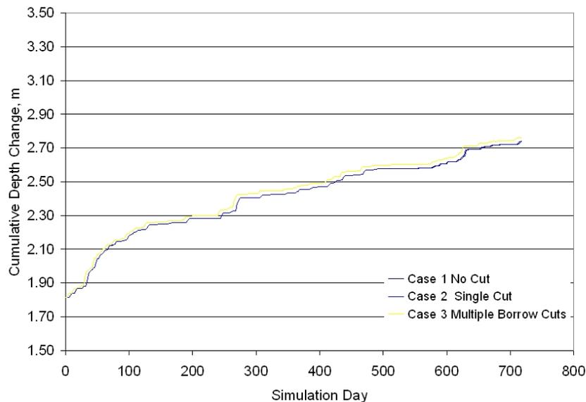
**Figure 4-33. Comparison of predicted topographic change on the upper shoreface at Station 32 over the two-year T1/T2 model simulation. Station location of is shown in Figure 4-26.**
