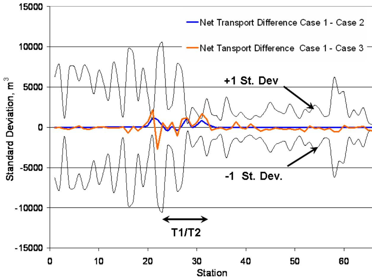
**Figure 4-24. Difference in predicted net littoral sand transport based on the T1/T2 model between Model Case 1 (Pre-Borrow Cut), Case 2 (Post Borrow Cut 2006) and Case 3 (Multiple Borrow Cuts). The differences are shown relative to the standard deviation of transport at each monitoring station.**
