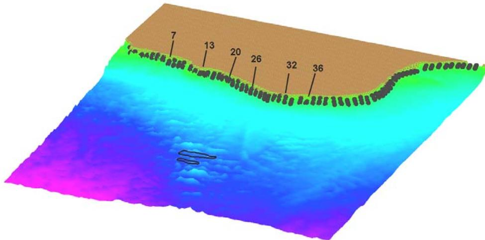
**Figure 4-29. Location of monitoring stations in the T1/T2 model grid from which time series of topographic change were extracted for individual cells in a transect across the littoral zone.**
