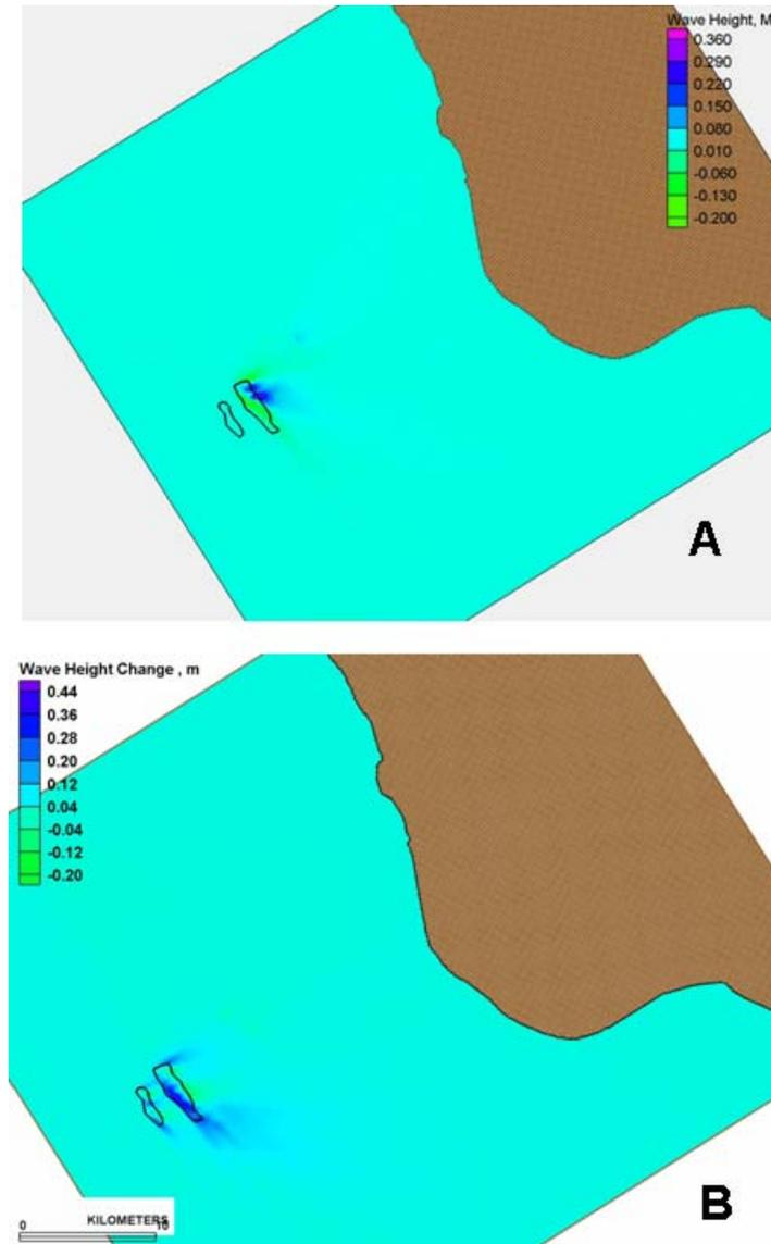
**Figure 4-13. Predicted difference in wave height during the 1998 winter storm after excavation of the 2006 borrow cut in Shoal T1 (Panel A) and after excavation of multiple borrow cuts in T1 and T2 (Panel B).**
