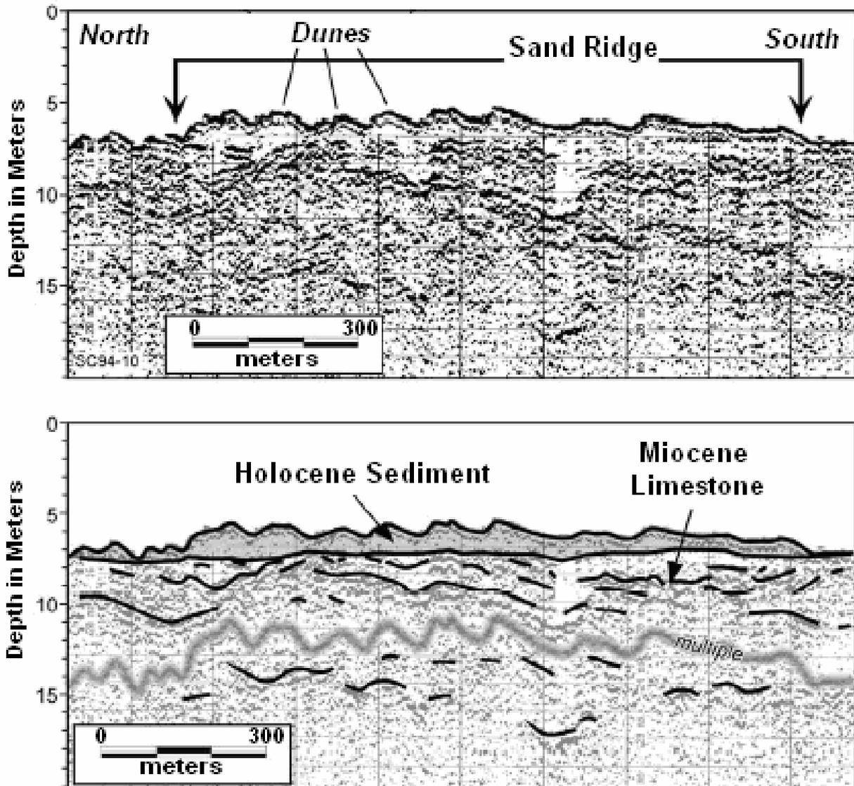
Figure 2-7. Seismic stratigraphy offshore of Indian Rock Beach north of Tampa Bay showing fields of large sand waves combining to form sand ridge topography (from Locker et al., 2003).
