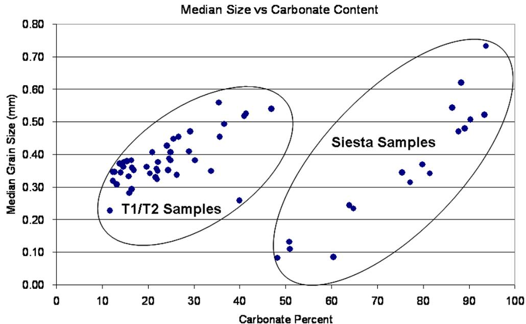
**Figure 3-7. 2006 Comparison of median grain size to percent carbonate fraction.**
