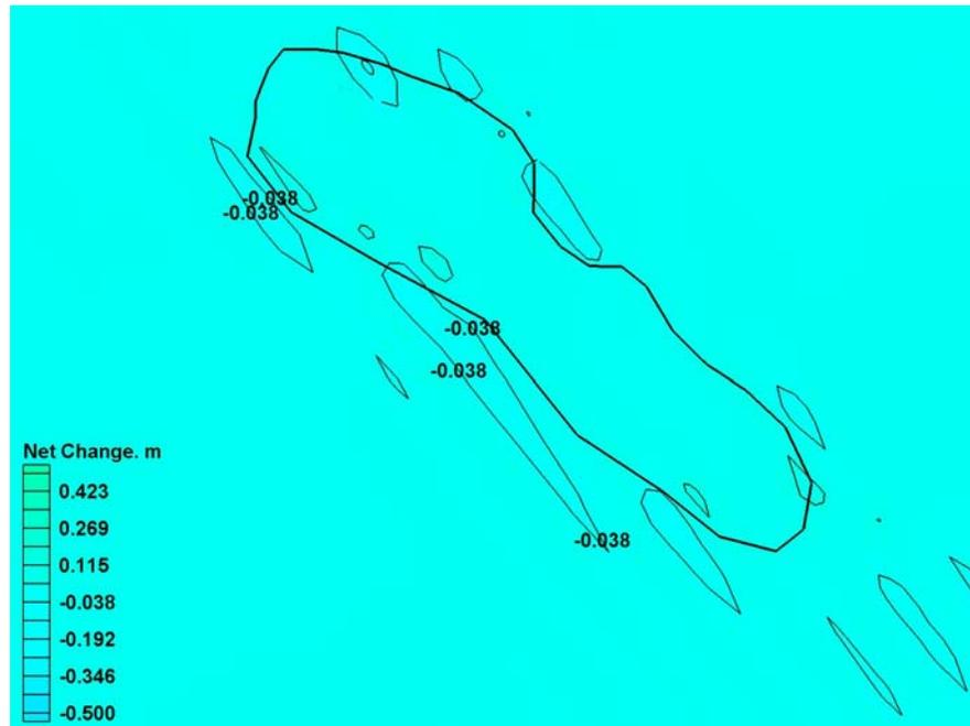
**Figure 4-55. Predicted net topographic change over the Siesta Shoal features after the cumulative borrow cut (Case 5, Table 4-1).**
