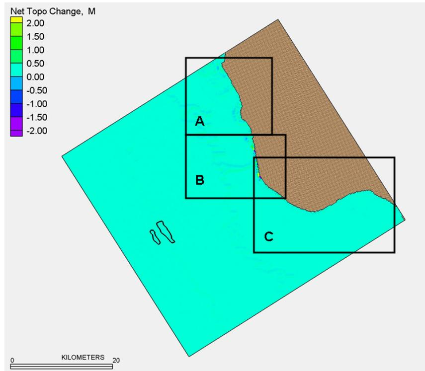
**Figure 4-25.** Location of three panels shown in Figures 4-26 to 4-28 showing predicted net topographic change after 2-years of simulation based on the T1/T2 model.
