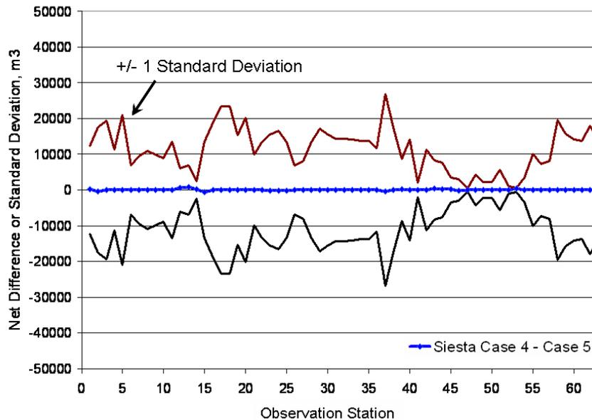
Figure 4-45. Difference in predicted net littoral sand transport based on the Siesta Shoal model between Model Case 4 (no borrow cut), and Case 5 (large borrow cut). The differences are shown relative to the standard deviation of predicted transport at each numerical observation station. The pre-and post- borrow cut morphology is shown in Figure 4-35.
