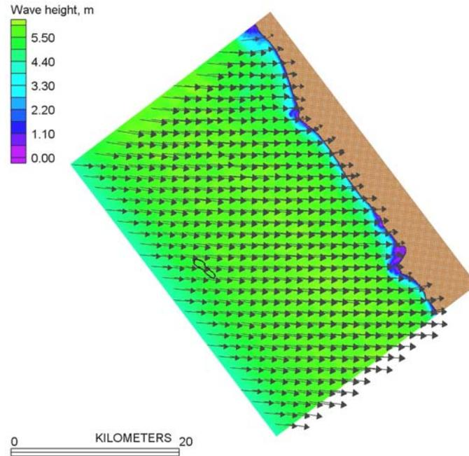
**Figure 4-36.** Wave pattern over the Siesta Shoal model grid for Case 4 during a winter storm producing high wave energy conditions in February of 1998. Significant wave heights are 4m and peak wave period 11s. Reduction of wave heights can be seen (in purple) near the shoreline as wave breaking occurs in shallow water.
