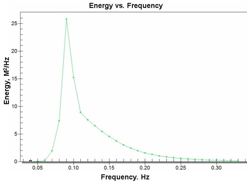
Figure 4-2. Spectral wave energy by direction for storm conditions in early February 1998.
