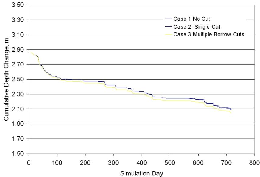
**Figure 4-32. Comparison of predicted topographic change on the upper shoreface at Station 26 over the two-year T1/T2 model simulation. Station location of is shown in Figure 4-26.**
