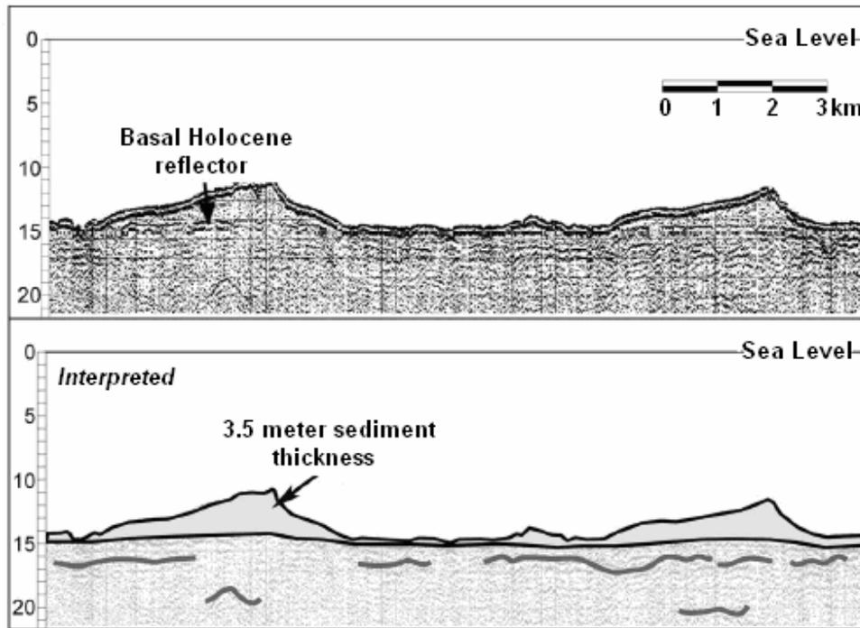
**Figure 2-6. Seismic cross-section through the Siesta Shoal selected for analysis in the current MMS project. The shoal is situated 14 miles offshore of Siesta Key in water depths of approximately 30-40 feet (from Locker et al., 2003).**
