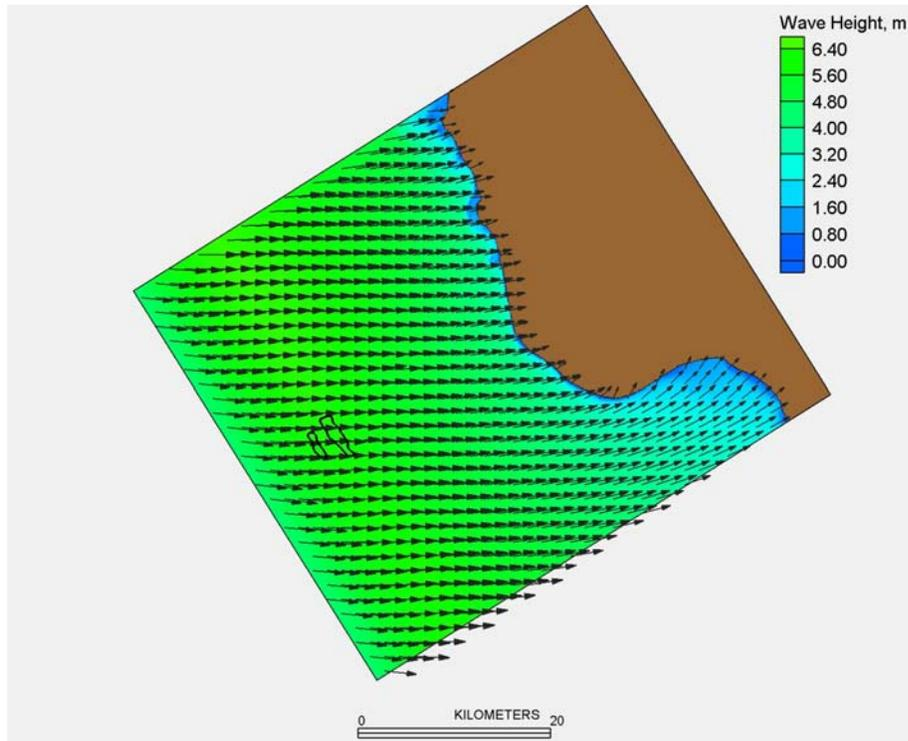
**Figure 4-11. Wave propagation pattern over the T1/T2 wave model grid during storm produced high wave energy conditions in February of 1998.**
