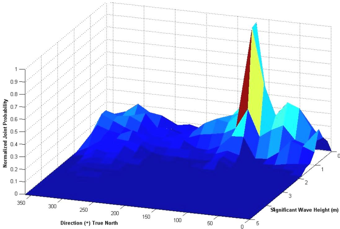
Figure 2-27. Joint probability between significant wave height and peak direction at WIS Station 290 between October and April. The hind cast time period is 1995-1999.
