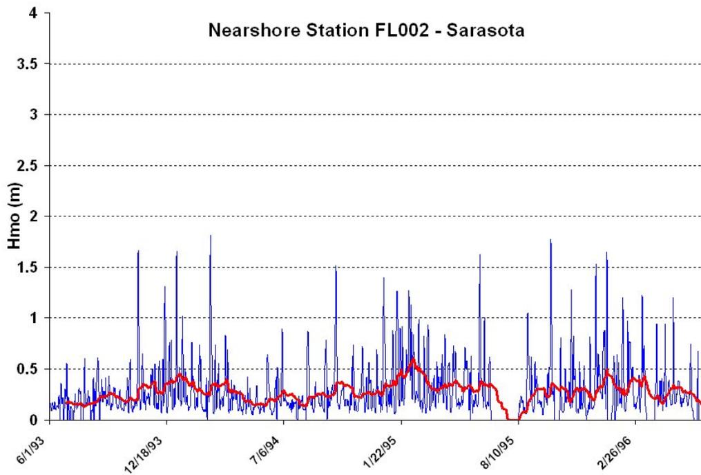
Figure 2-30. Significant wave height record from WES/CHL nearshore directional wave gage FL002 deployed from 1993 to 1996 off Sarasota, FL.
