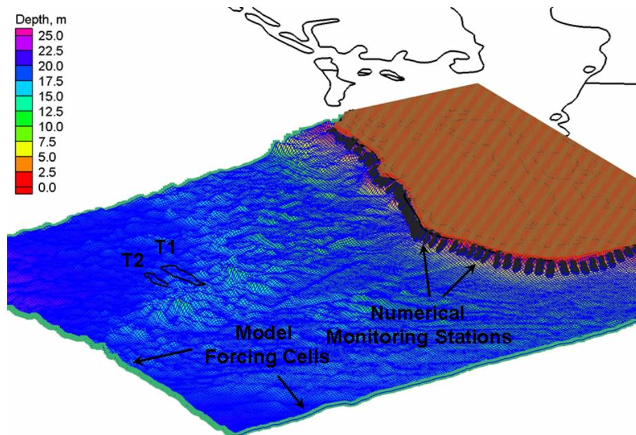
**Figure 4-4. Circulation model grid, model forcing cells, and location of numerical monitoring stations at the shoreline.**
