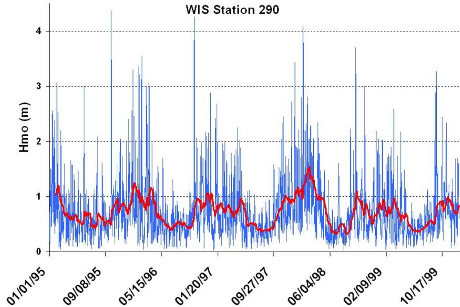
Figure 2-28. Hind cast of significant wave heights at WIS Station 290 from 1995 through 1999. The trend line is a 60-day moving average.
