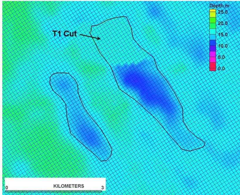
Figure 4-9. Representation of the existing 2006 borrow cut in the T1 Shoal within the wave model grid.
