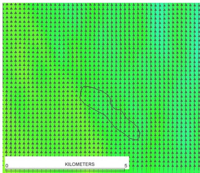
**Figure 4-39. Details of predicted wave energy propagation over Siesta Shoal during Tropical Storm Harvey. Refer to Figure 4-12 for a comparison to the T1/T2 Shoal feature. Model topography is for the existing morphologic situation of Siesta Shoal (Case 5, Table 4-1).**
