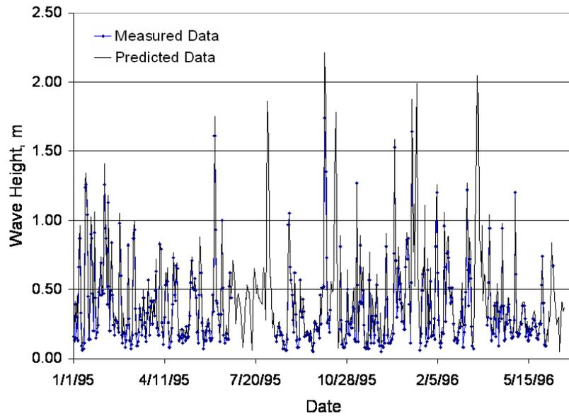
**Figure 4-6. Siesta Shoal: Comparison of predicted and measured wave height data at ERDC Station F002 from January 1995 through May 1996. Statistical comparison included a RMS error of 0.06 m and ME of 0.05 m. Refer to Figure 4-5 for the location.**
