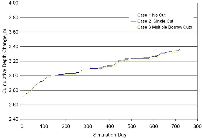
**Figure 4-31. Comparison of predicted topographic change on the upper shoreface at Station 20 over the two-year T1/T2 model simulation. Location of station is shown in Figure 4-26.**
