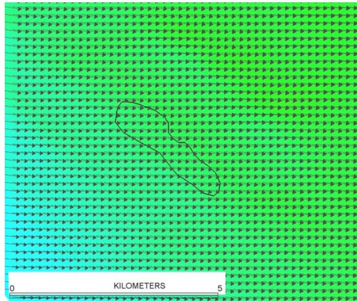
**Figure 4-37.** Details of predicted wave movement over Siesta Shoal during the 1998 winter storm. Maximum wave heights over the shoal are 4 m, whereas the wave period is 11s. Refraction or bending of wave rays tracing the movement of wave energy is not apparent.
