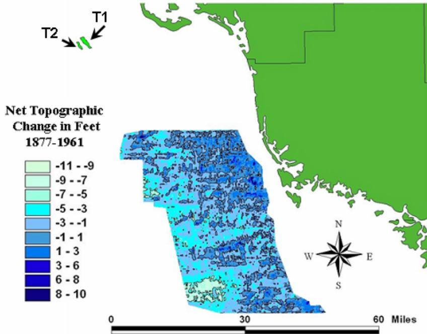
Figure 2-16. Net differences between interpolated topographic surfaces calculated from the overlap areas of the 1877-88 survey data and the 1955-61 survey data sets.
