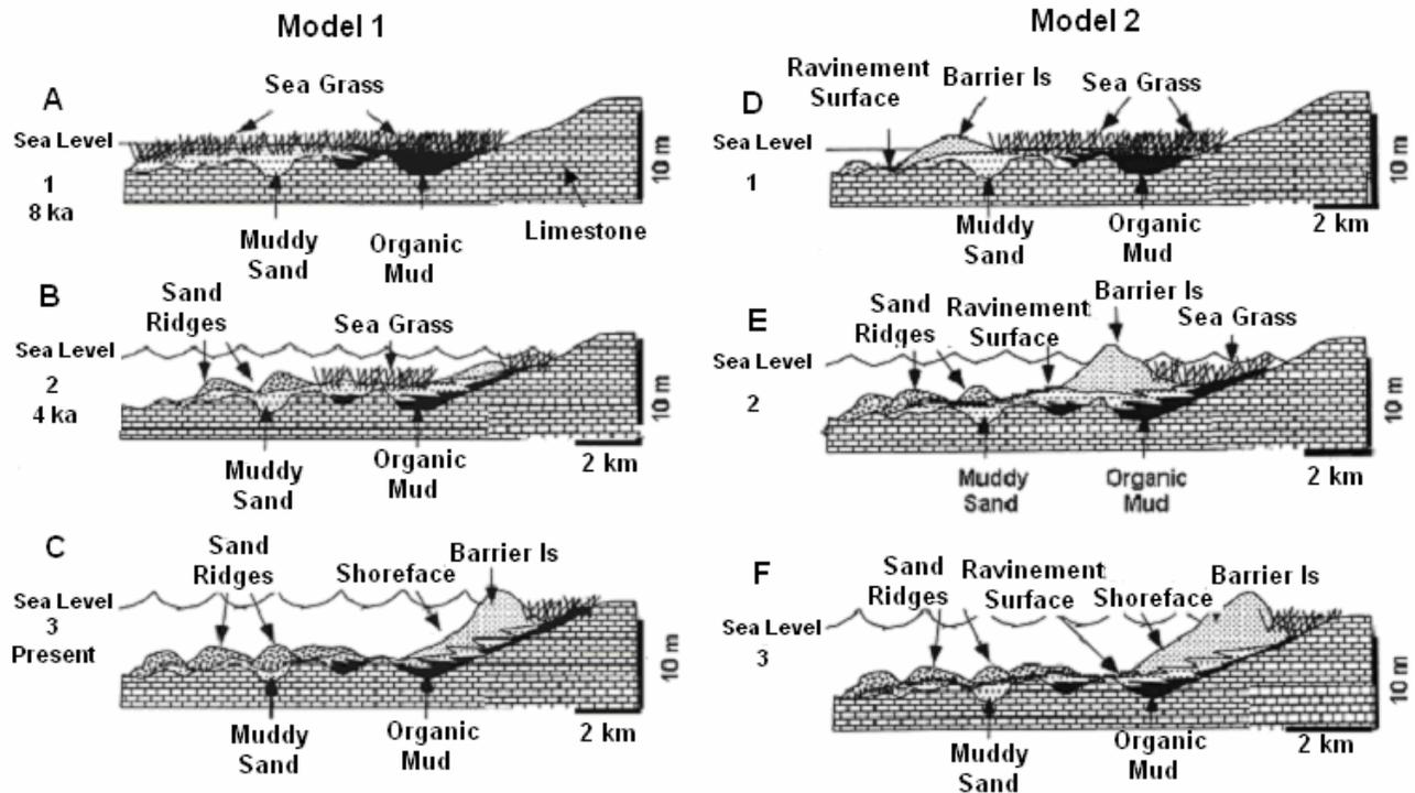
**Figure 2-14. Conceptual models of sand ridge and barrier island development on a shallow, low gradient shelf originally dominated by seagrass beds (from Edwards et al., 2003).**
