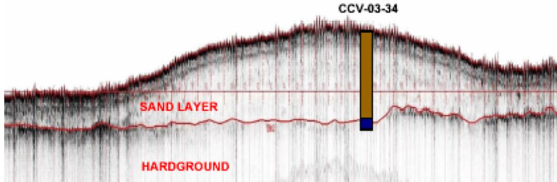
**Figure 2-13. A seismic cross-section through the T1 sand ridge. Maximum relief is approximately 20 feet. Location is shown in Figure 2-12 (from Finkl et al., 2004).**
