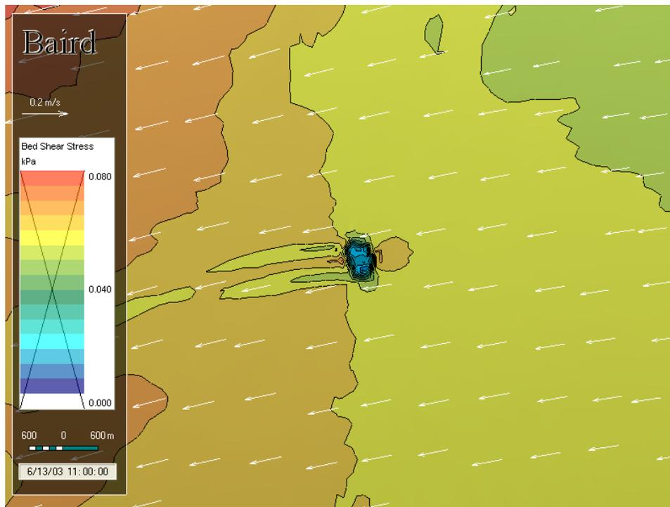
**Figure 3.48a Near Bed Flow Vectors Overlaid on the Bed Shears Stress Map for the Full Model Domain and the Higher Flow Condition**
