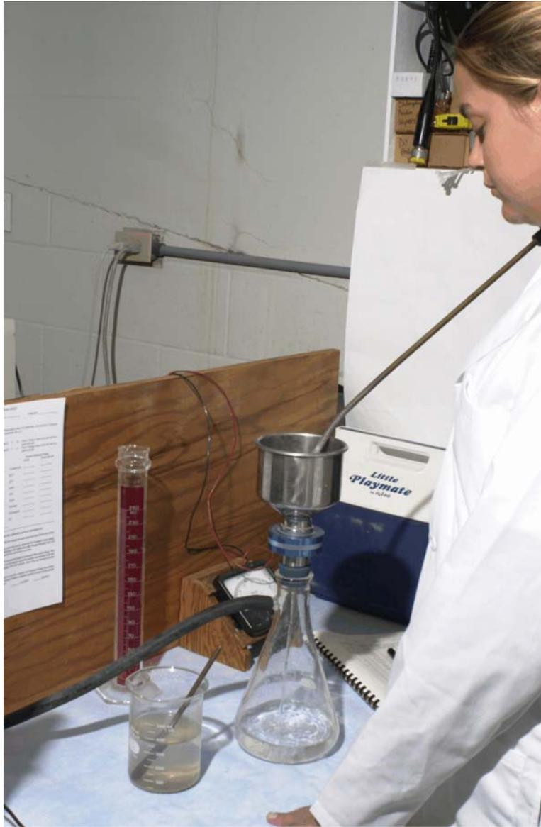
Figure A4 Wet sieving sediment using a vacuum pump and a Millipore Hydrosol SST filter holder
