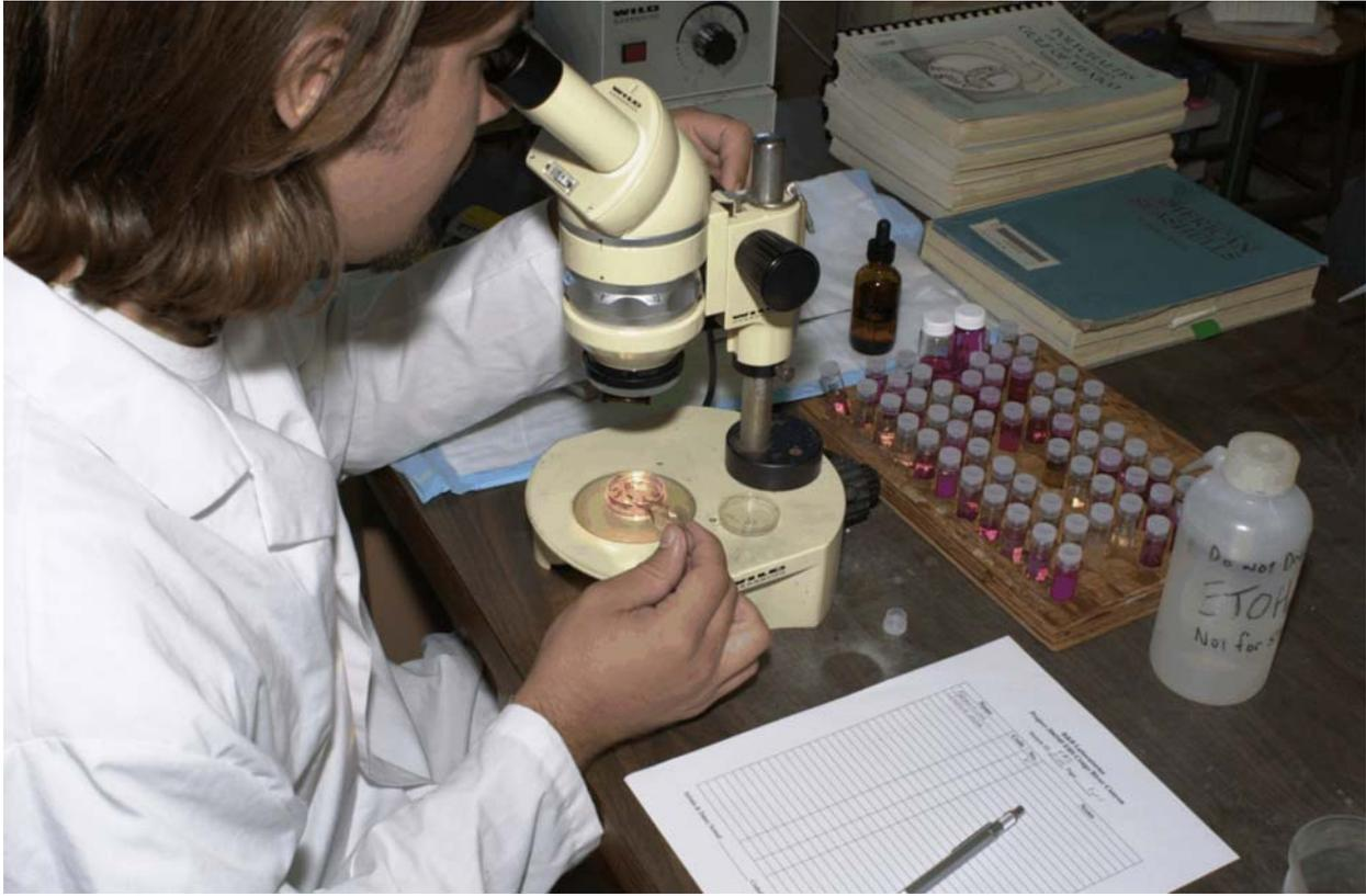
Figure A2 Identifying and enumerating macrofauna under a dissecting microscope
