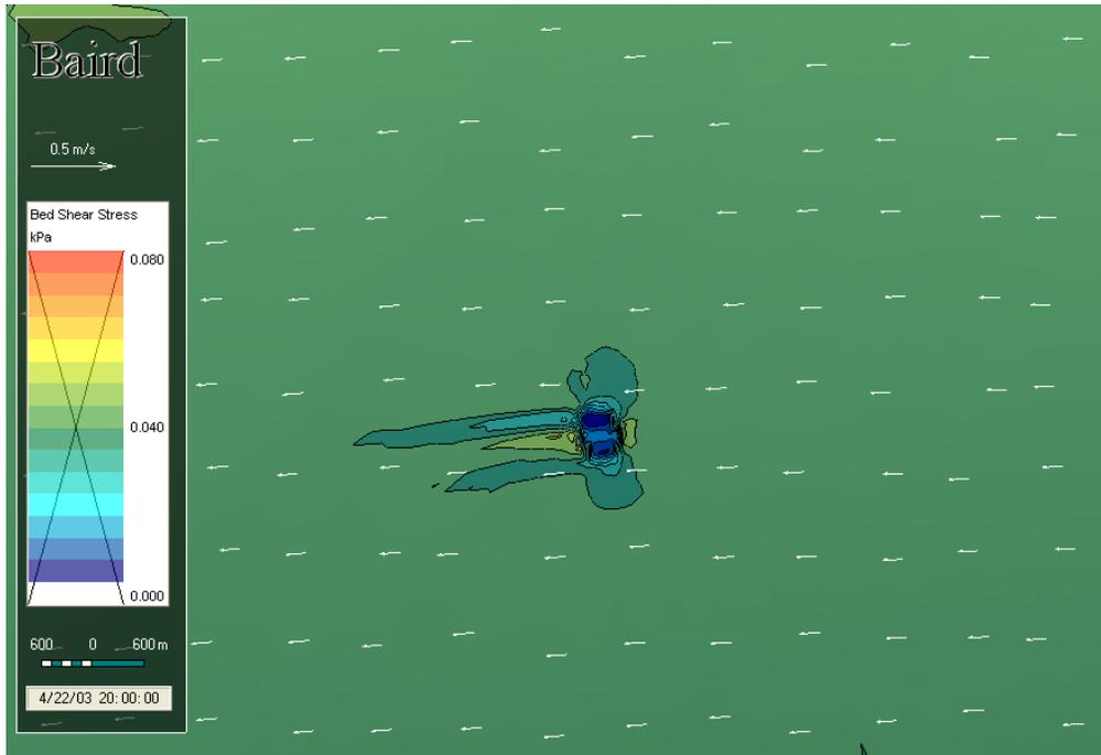
**Figure 3.47a Near Bed Flow Vectors Overlaid on the Bed Shears Stress Map for the Full Model Domain and the Lower Flow Condition**
