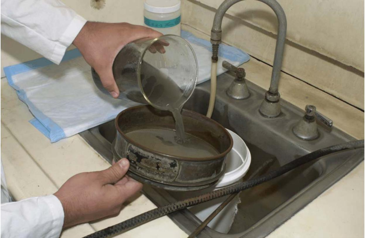
Figure A1 Sieving sediment on a 0.5 mm sieve
