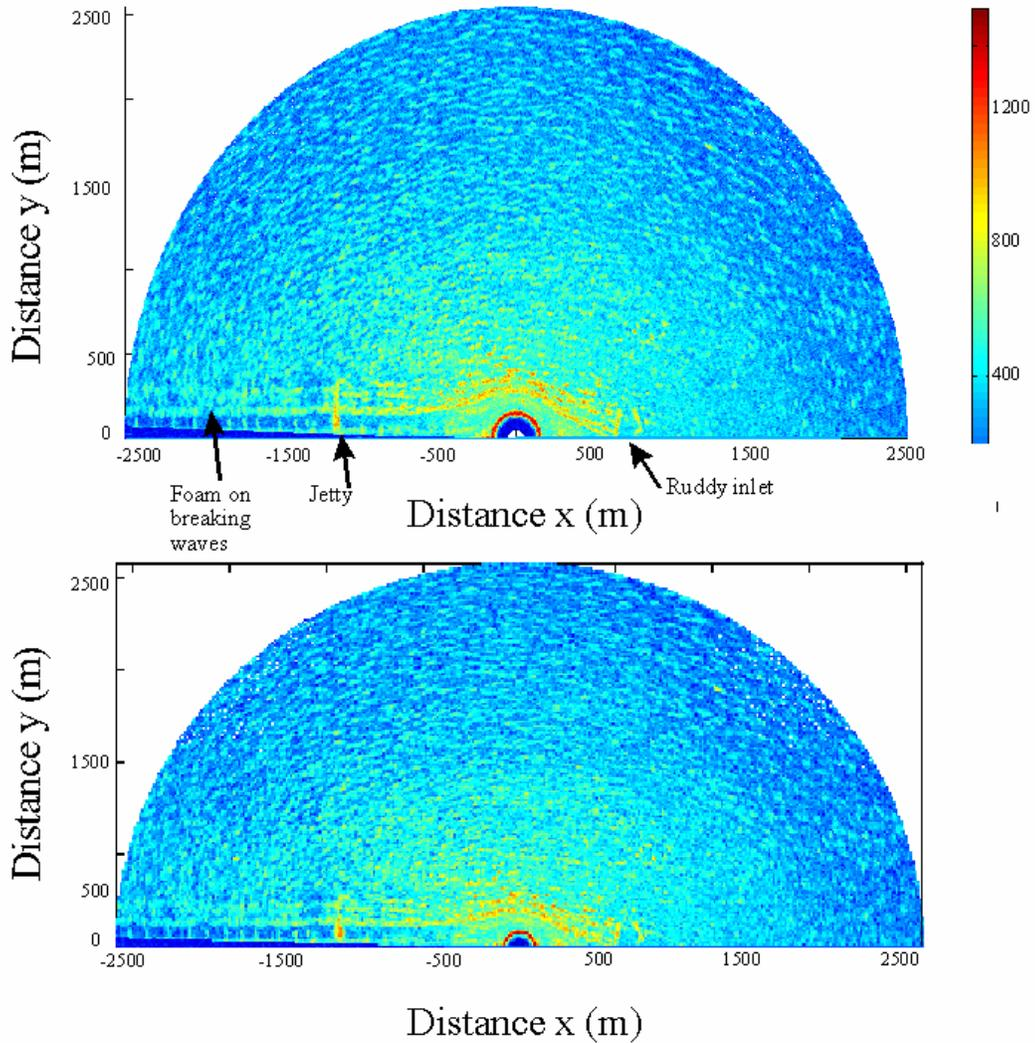
Fig. 3-6. An example of the radar images obtained at the Virginia Beach on 18:00, Feb. 17, 2004. (a) All the radar burst lines (1750) are used (b) only 437 burst lines are used for the image.
