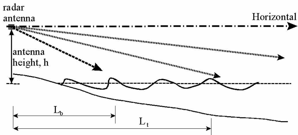
Fig. 3-7. Sketch to show the image distortion caused by side (or side lobe) effect when there is a strong echo at near field ( $< 500$  m from radar). Echoes from breaking wave foams at a distance  $L_b$  from the radar exceeds the echo strength at the true distance  $L_t$  which is calculated by the EM wave travel speed and the time duration after trig.
