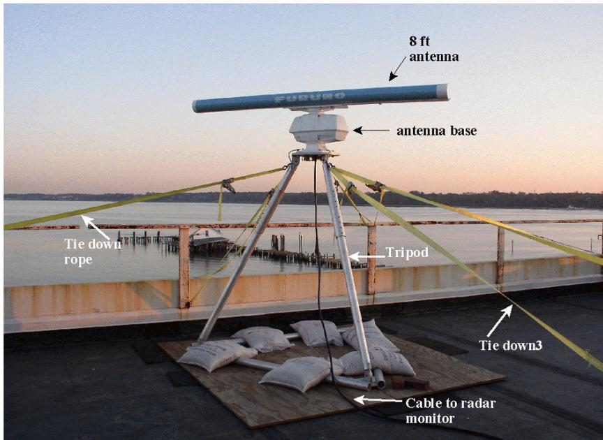
Fig. 2-1. Setup of an X-band radar at a building roof.
