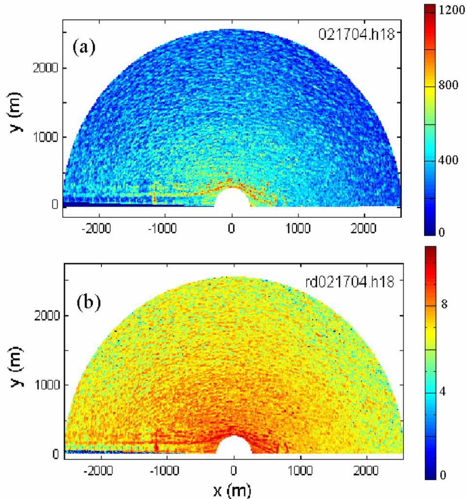
Fig. 5-1. A radar image with a relatively severe sea ( $S_a = 410$ ) obtained at Virginia Beach at 18:00, Feb. 17, 2004. (a) Image from raw data, (b) image after a processing to reduce the distance effect.
