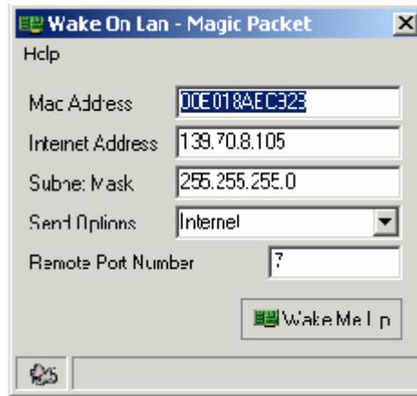
Fig. 7-1. The window generated when running the program WaveOnLanGui for WOL.
