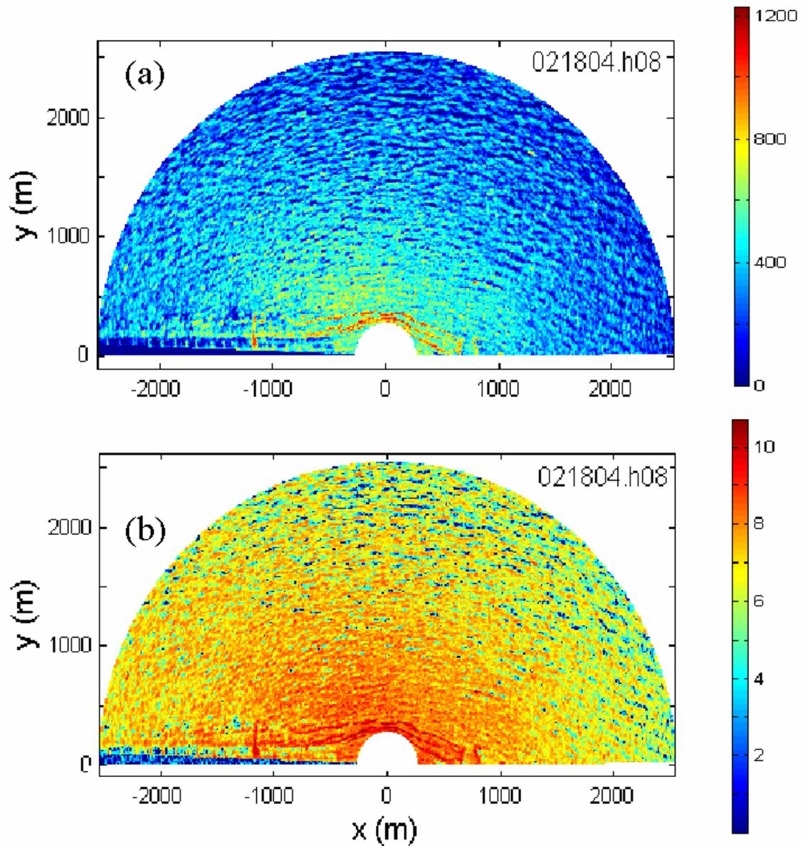
Fig. 5-2. A radar image with a relatively severe sea ( $S_a = 404$ ) obtained at Virginia Beach on 08:00, Feb. 18, 2004. (a) Image from raw data, (b) image after processing to reduce the distance effect.
