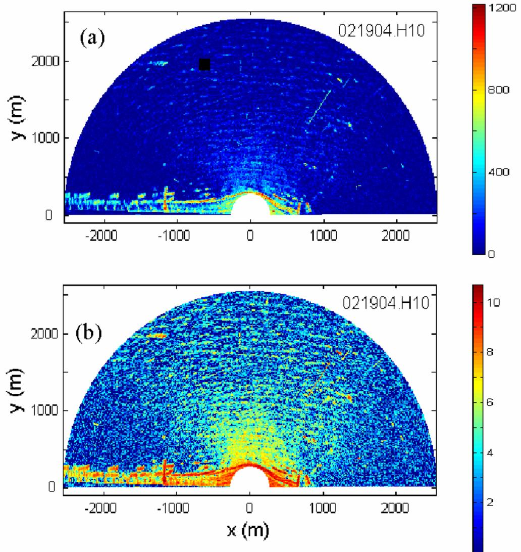
Fig. 5-3. A radar image with a relatively calm sea ( $S_a = 120$ ) obtained at Virginia Beach at 10:00, Feb. 19, 2004. (a) Image from raw data, (b) image after a process to reduce distance effect.
