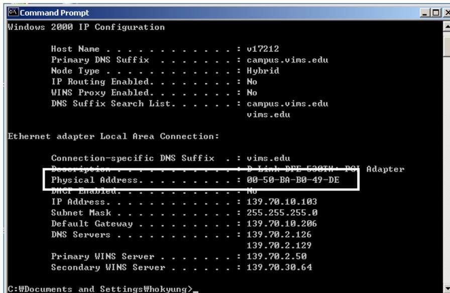
Fig. 7-2. An example of the window for the command prompt showing the MAC address which is the same as the 12-digit physical address. Each individual NIC has its own MAC different from other NICs.
