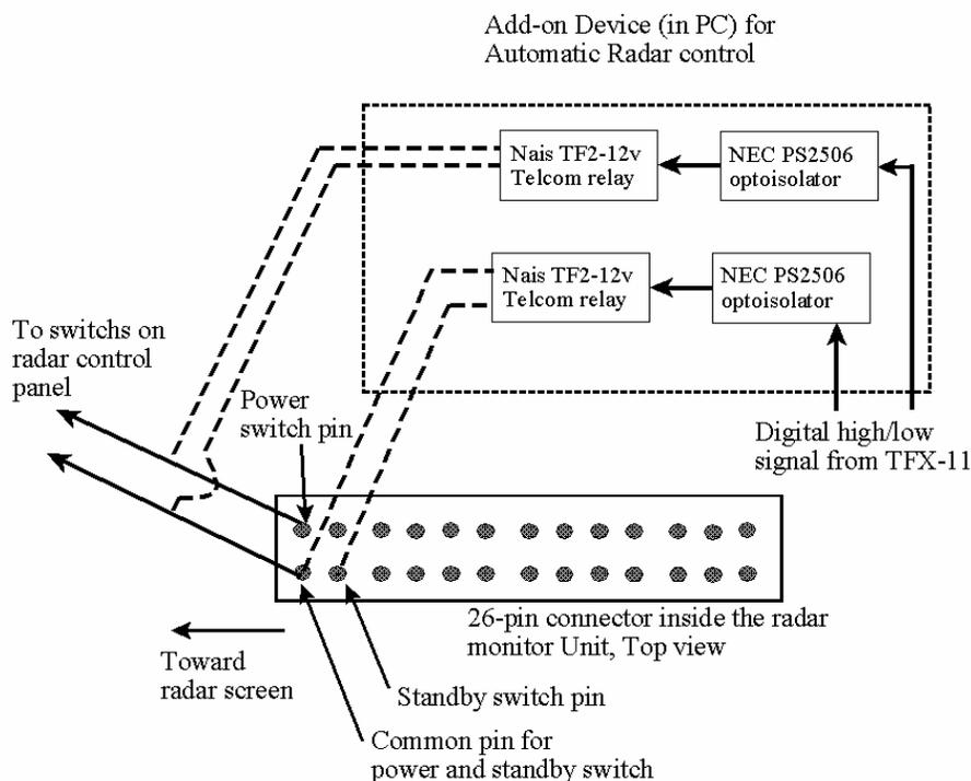
Fig. 3.2. Wiring diagram for turning a FURUNO 8251 radar on and off.
