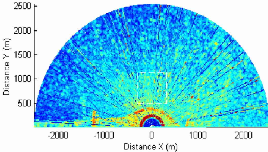
Fig. 8-1. A raw radar image showing the incorrect setting of the radar measurement range and the occasional missing line image.
