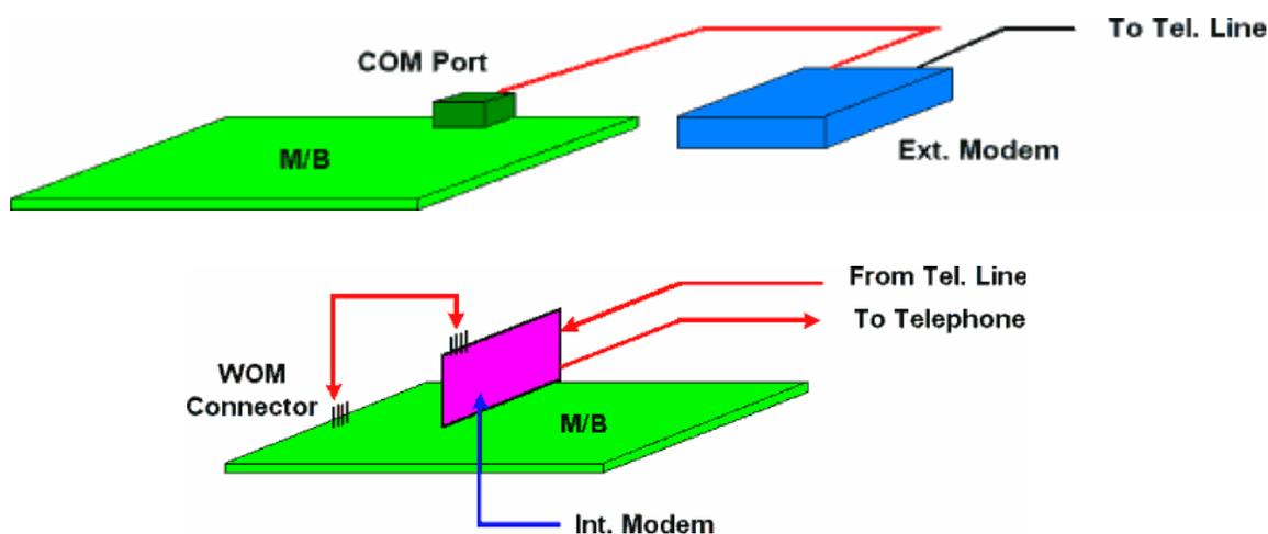
Fig. 7-3. The device connection diagram for WOM using either external or internal modems.
