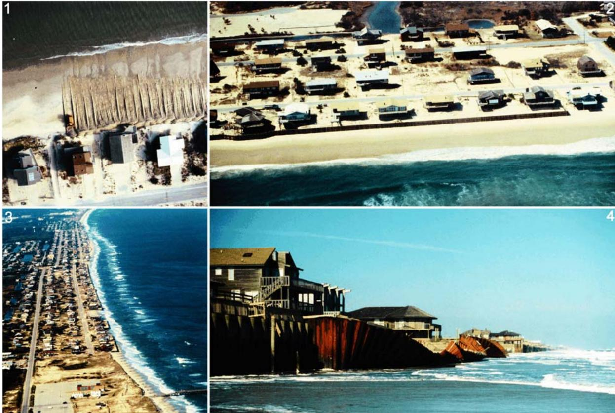
Figure 2: Photographs depicting the chronic shoreline erosion and the effort of the local residents to mitigate loss of property. Descriptions from top left: 1) bulldozing to elevate foredune and dune (1985), 2) seawall construction along south central Sandbridge (1986), 3) oblique aerial photograph looking north from Little Island Park (1990), and 4) seawall failure (1994).
