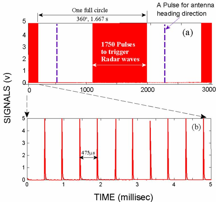
Fig. 2-4. For a FURUNO FR8251 radar, the radar scanning domain can be specified. (a) Within this domain, pulses are generated from the radar control unit at a rate of 2,100 pulse/s to trigger the burst of radar waves. (b) Detail of the pulses pattern within the scanning domain. These pulses also were used to trigger the ADC conversion.
