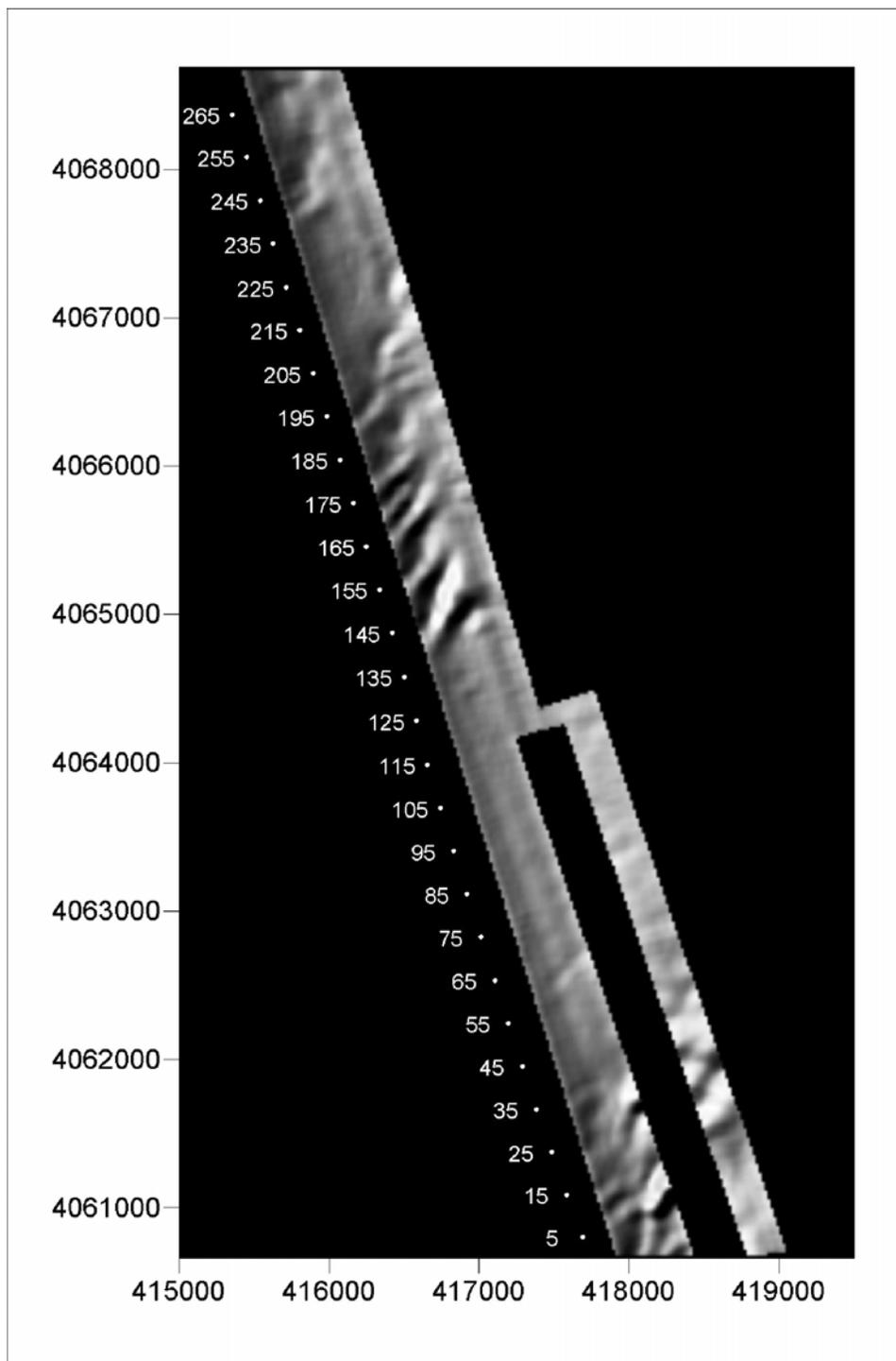
Figure 35: A 2002 interferometric swath bathymetry survey documented complex nearshore morphology along the southern end of Sandbridge Beach. This reach was characterized by a series of shore-oblique sand bars and gravel patches. Every other WSE beach profile location is provided for reference; profiles ending in 0 are profile lines that actually extended offshore (not shown). Coordinates in UTM NAD 1983 (m).
