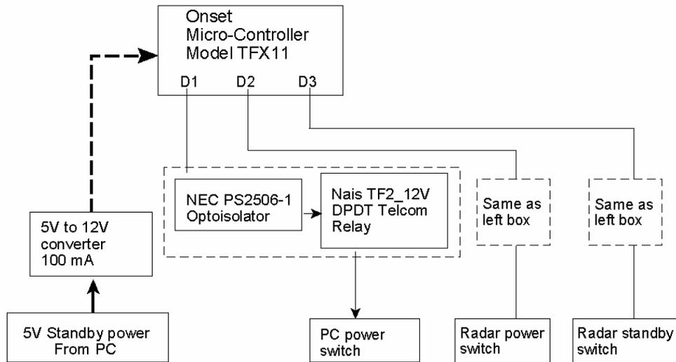
Fig. 2-5. Schematic diagram of the PC and radar auto-control.
