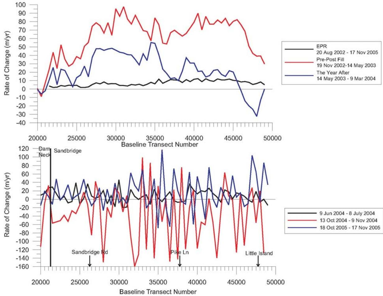
Figure 27: Selected rates of shoreline change as calculated from MHW generated by data collected with the ATV RTK-GPS system.
