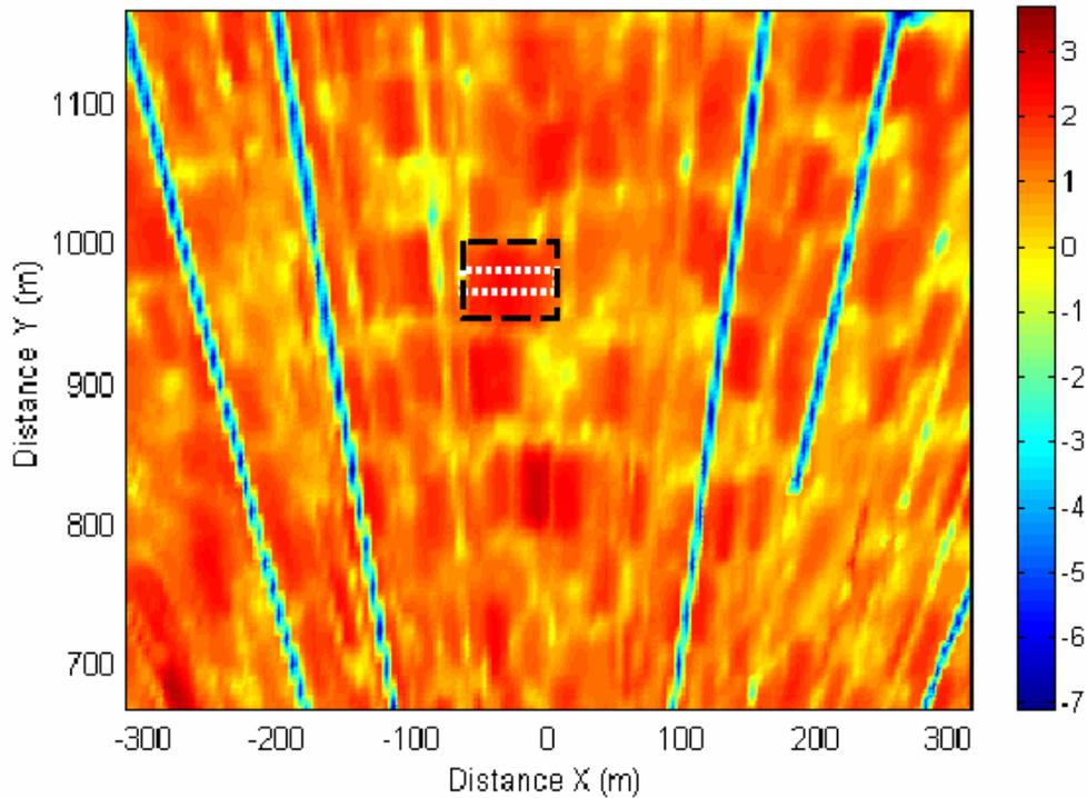
Fig. 8-2. The Incorrect setting on radar measurement range changes the image size from that in the thin white dotted box to that in a much thicker black dashed box. The occasional missing line images (the blue lines) produce a strong signal after FFT and with the result that waves always travel in a direction parallel to the x axis.
