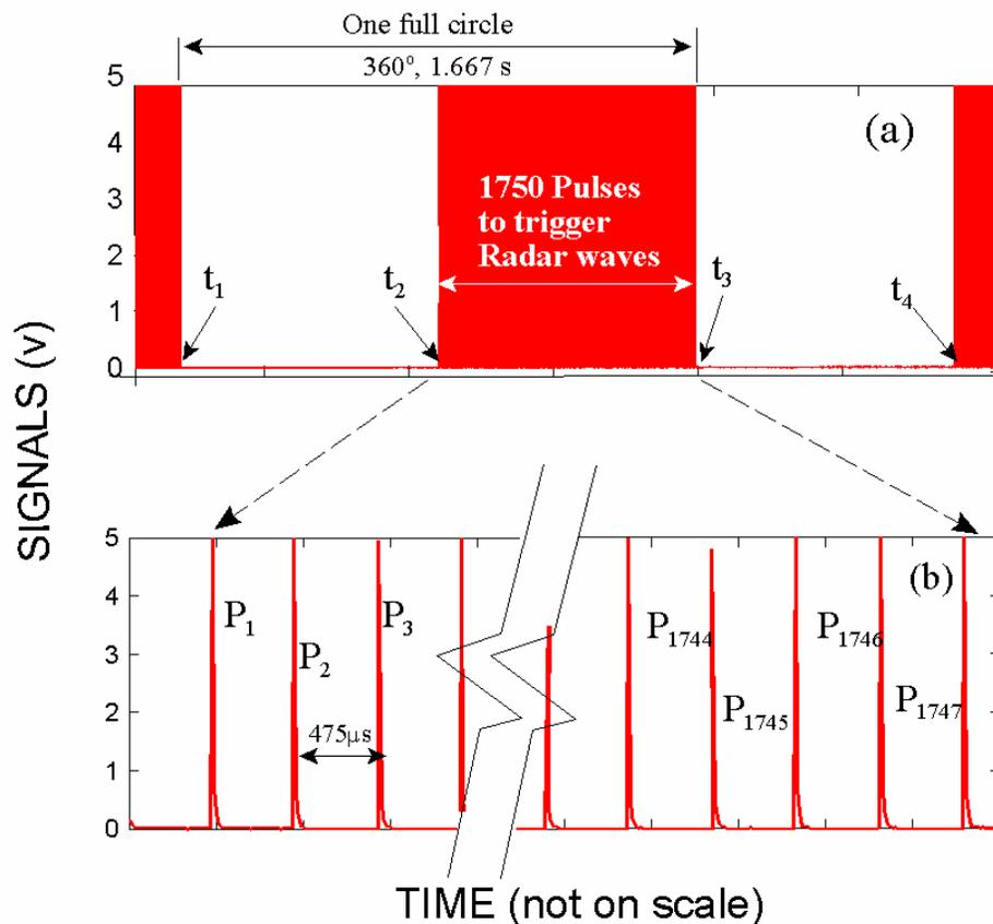
Fig. 3-4. A sketch showing the algorithm for finding the first trigger pulse,  $P_1$ , when the data acquisition software starts. This algorithm requires a radar has the capability of setting a angular sector for observation. Between time  $t_1$  and  $t_2$ , there is no trigger signal.
