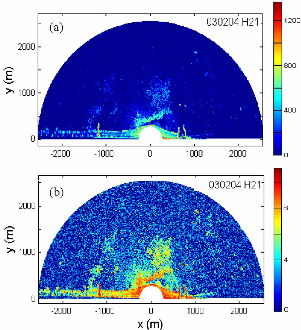
Fig. 5-4. A radar image with a relatively calm sea ( $S_a = 105$ ) obtained at Virginia Beach at 21:00, Mar. 2, 2004. (a) Image from raw data, (b) image after a process to reduce distance effect.
