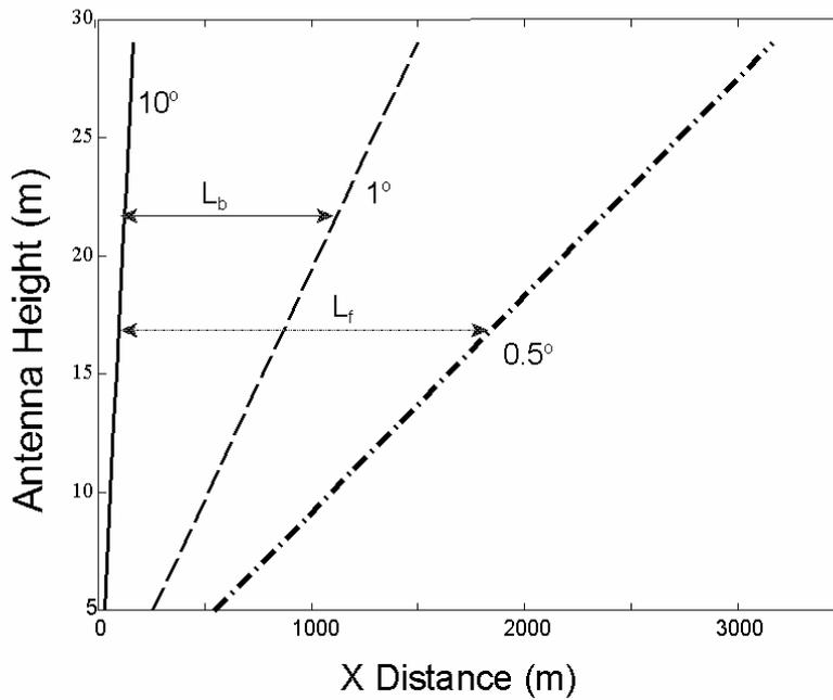
Fig. 2-3. Relationship between radar antenna height and the better working area.  $L_b$  is for an impinging angle of  $1^\circ$  and  $L_f$  is for a possible extension of the better working area by decreasing the impinging angle to  $0.5^\circ$ .
