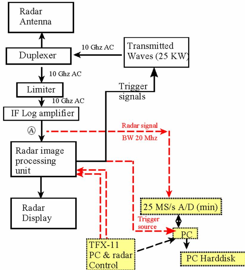
Fig. 3-1. System diagram for the radar wave observation system. The dotted boxes indicate hardware added to the system, and the dashed lines mark the flow of control signals and radar image. All solid boxes are from a radar manufacturer.
