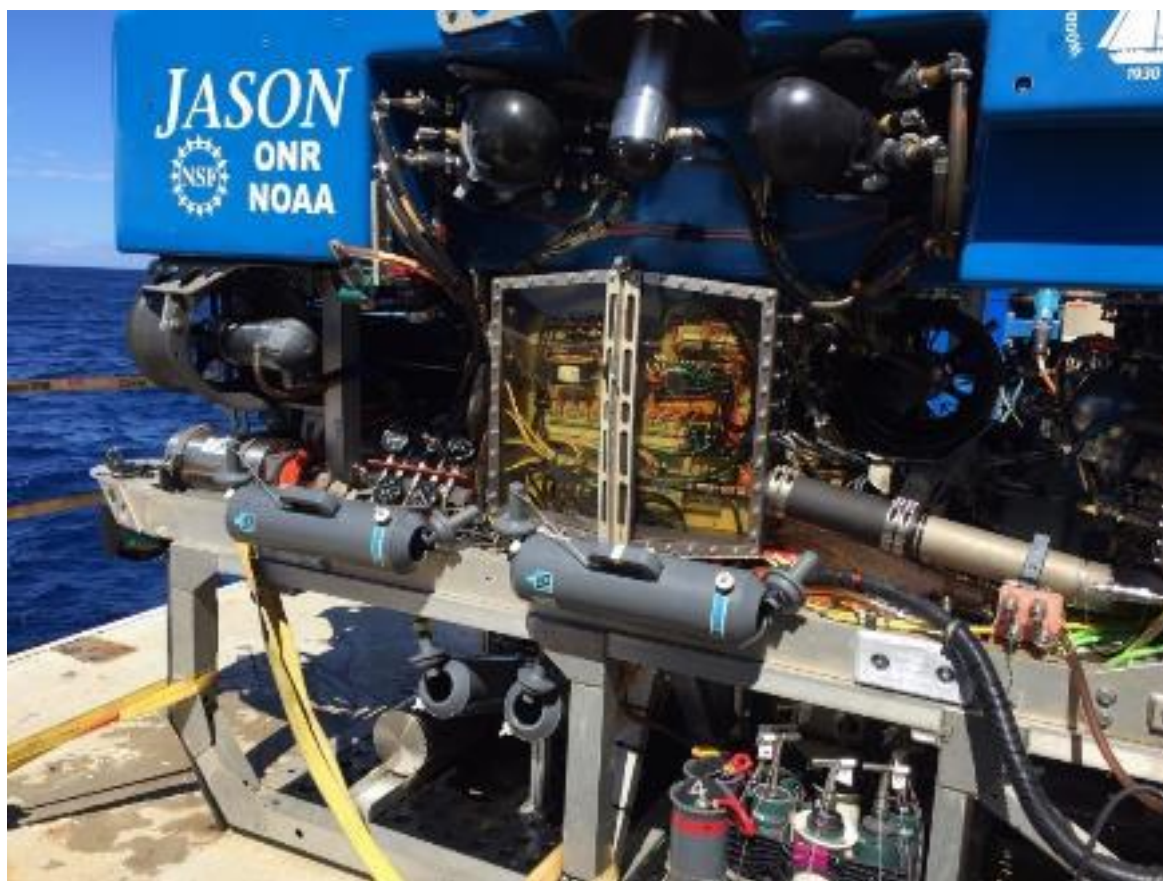
Figure 4-107. Mounting and orientation of the Niskin bottles on Jason for collections Collection of deep-sea bottom water. Niskin bottles on the side of the ROV were not used for eDNA collection, and openings of the two eDNA bottles are visible on the bottom center left. Photo: C. Kellogg.
