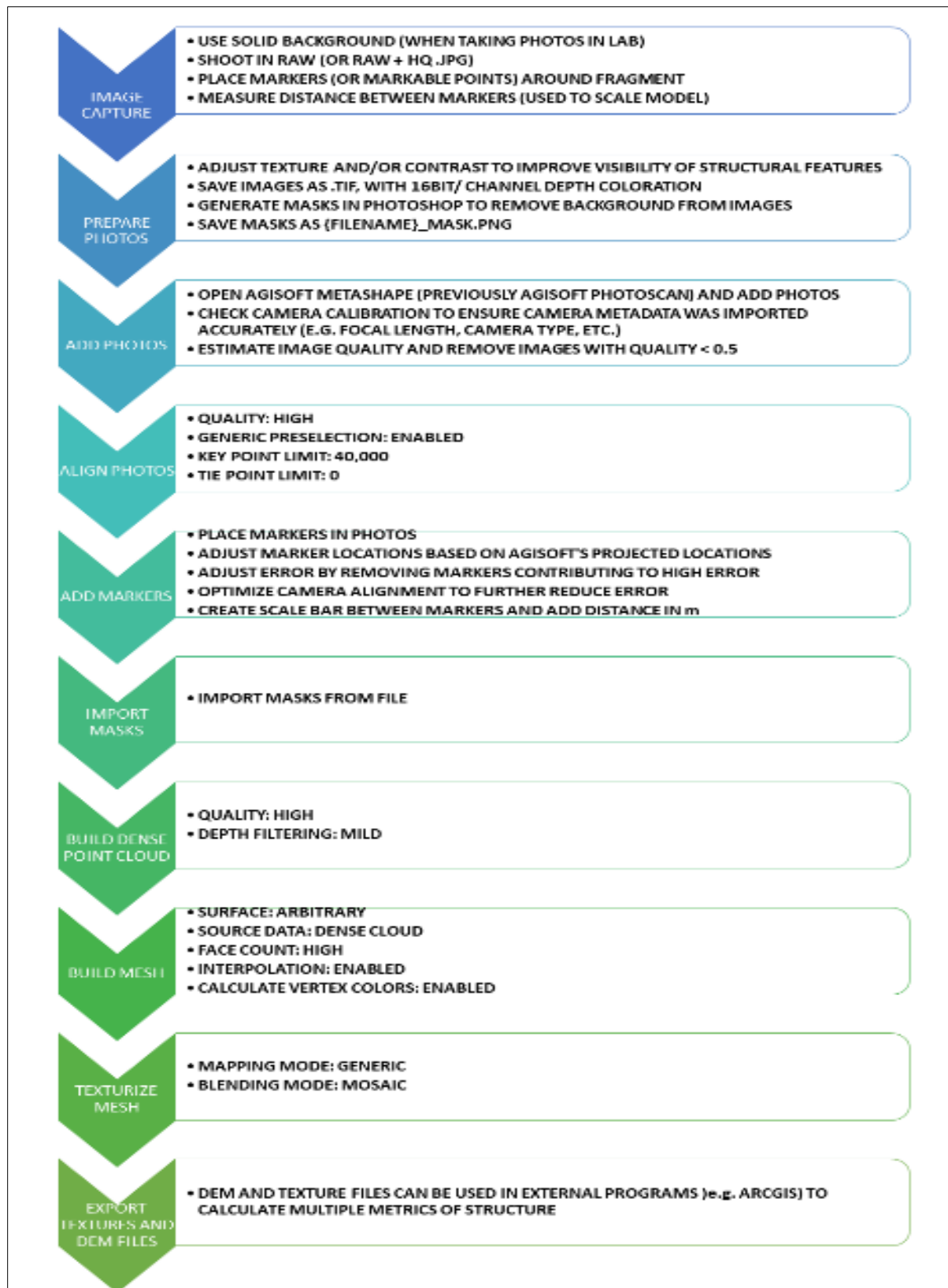
Figure 5-10. Schematic of workflow for creating models of coral fragments
