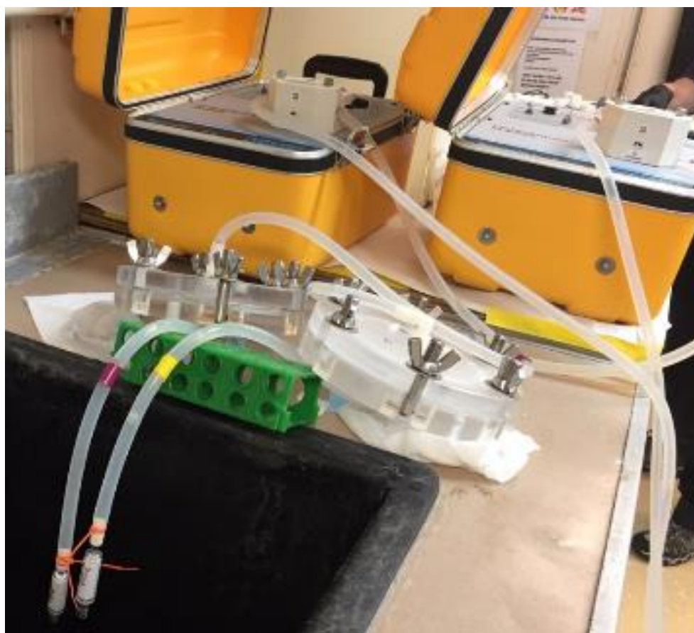
Figure 4-108. Laboratory setup for water filtration of 10 L seawater from Niskin bottles
