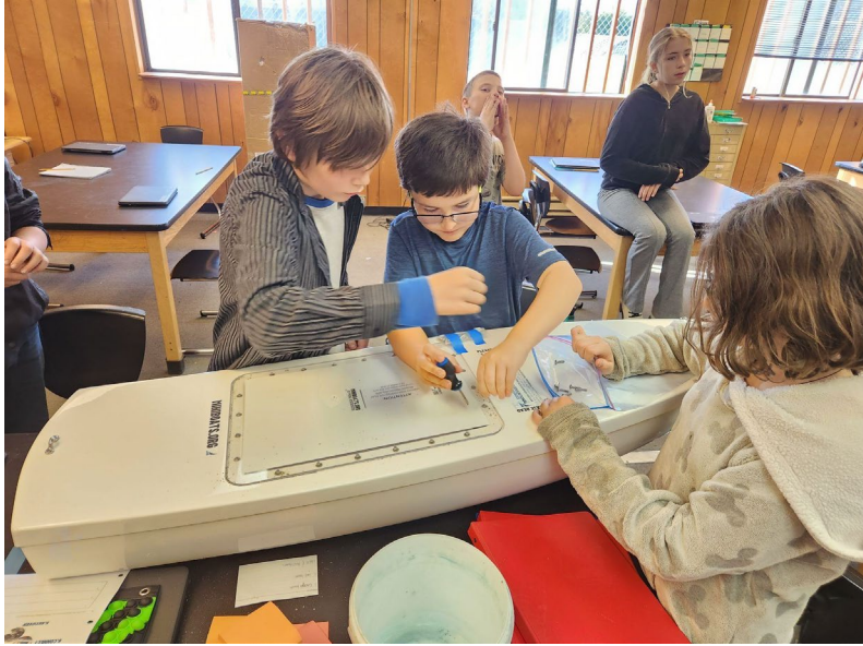
Figure 7. Members of the Cargo team during construction The team members dry-fit the cargo hatch to determine the instrument and solar panel locations.
