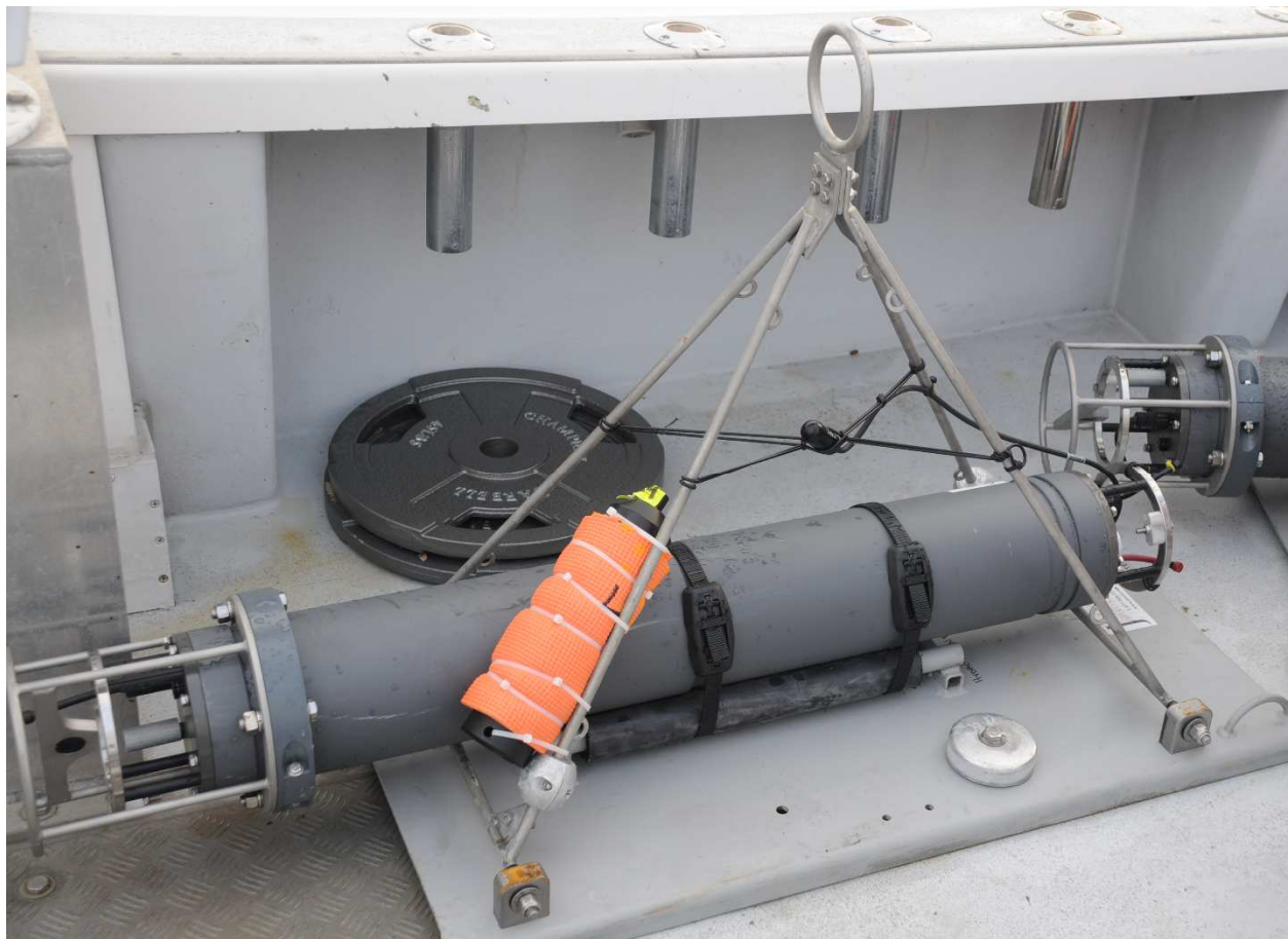
Figure 3.1.1b. Autonomous Multichannel Acoustic Recorder (AMAR) External view of the Autonomous Multichannel Acoustic Recorder (AMAR).
