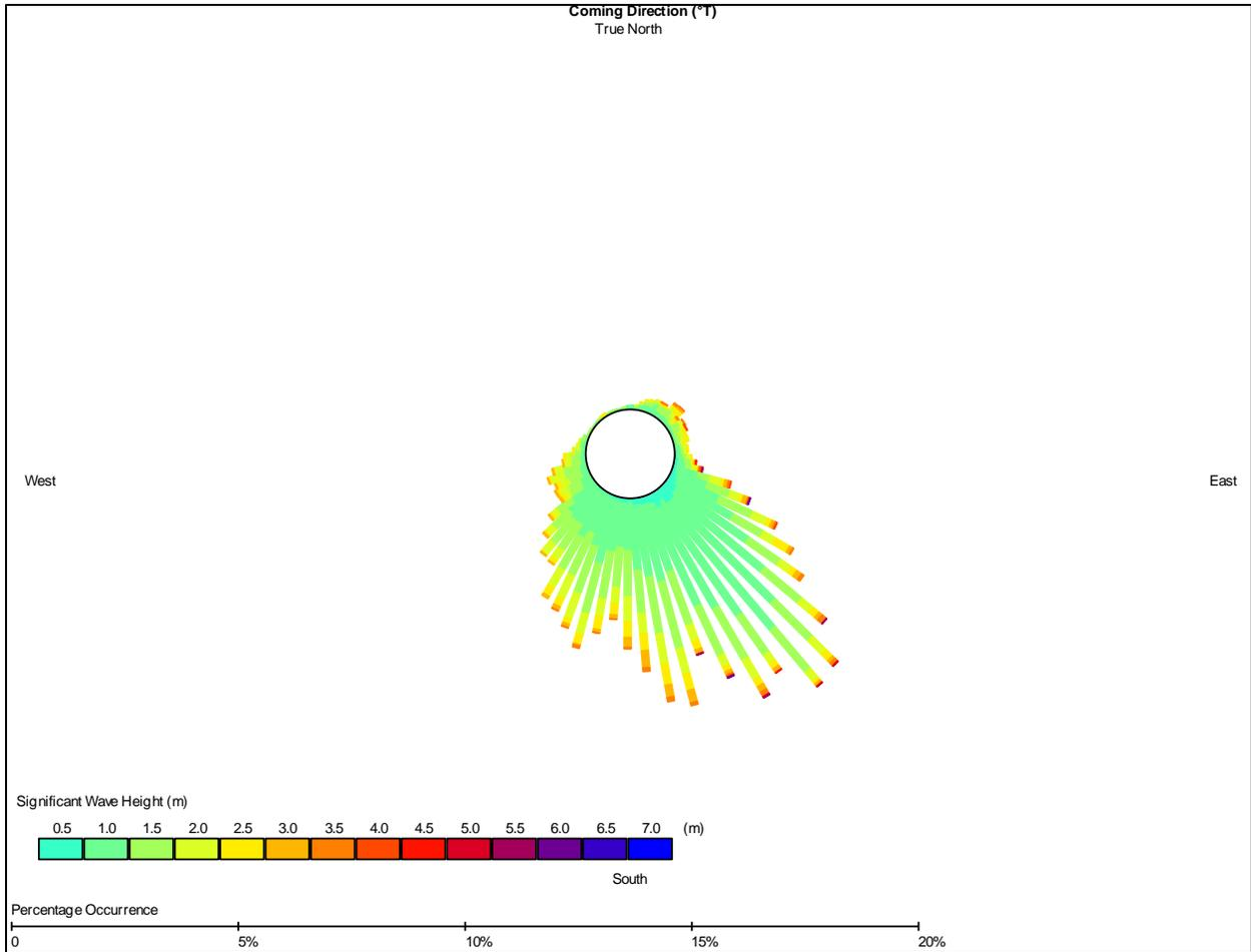
Figure 5. All Wave Data – Significant Wave Height Versus Coming Direction Hodogram (rose plot)
