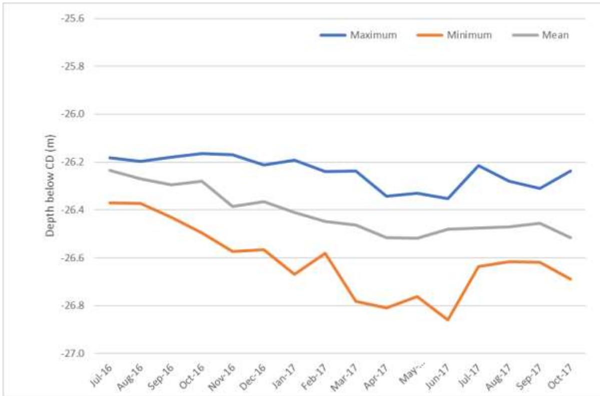
Figure 13. NE Beam 3 Scour Depth
