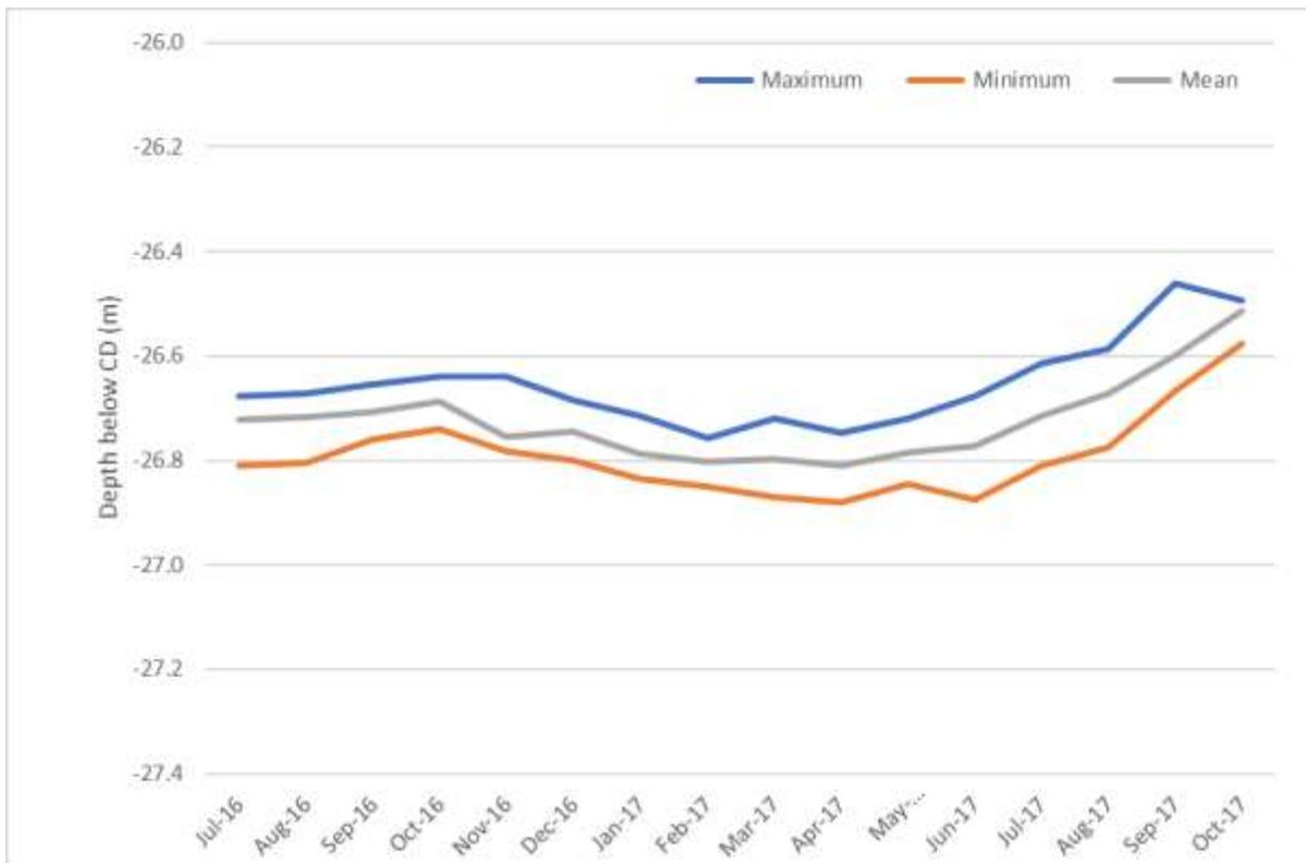
Figure 10. SE Beam 4 Scour Depth
