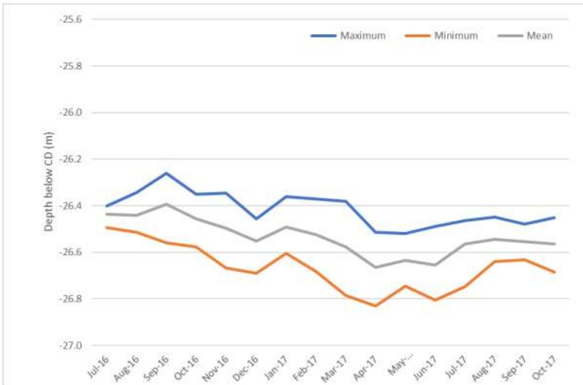
Figure 12. NE Beam 2 Scour Depth
