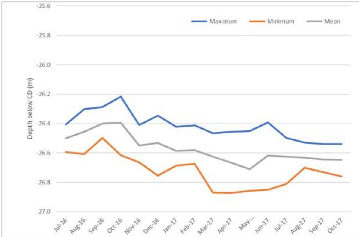
Figure 11. NE Beam 1 Scour Depth
