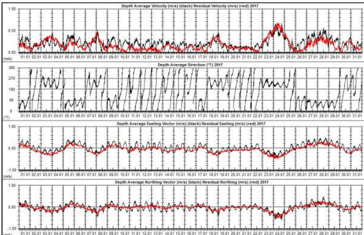
Figure 3. January 2017 Current Data – Observed and Non-tidal Components
