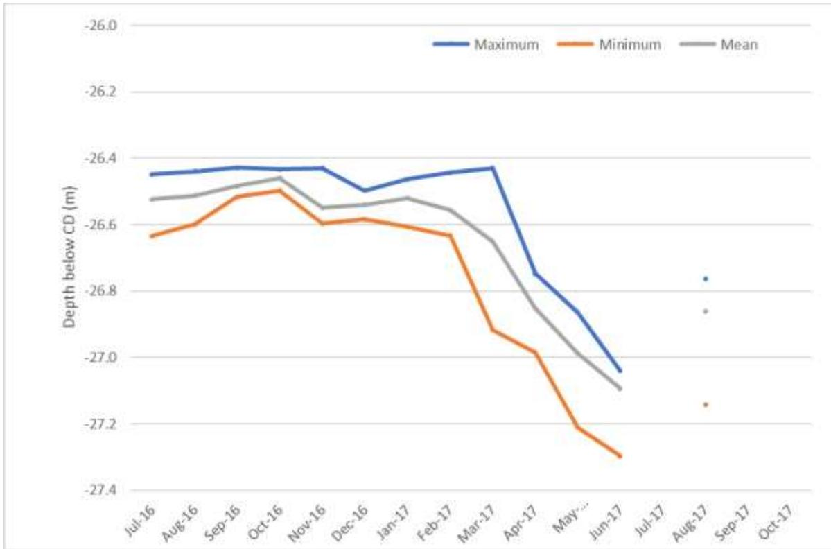
Figure 7. SE Beam 1 Scour Depth
