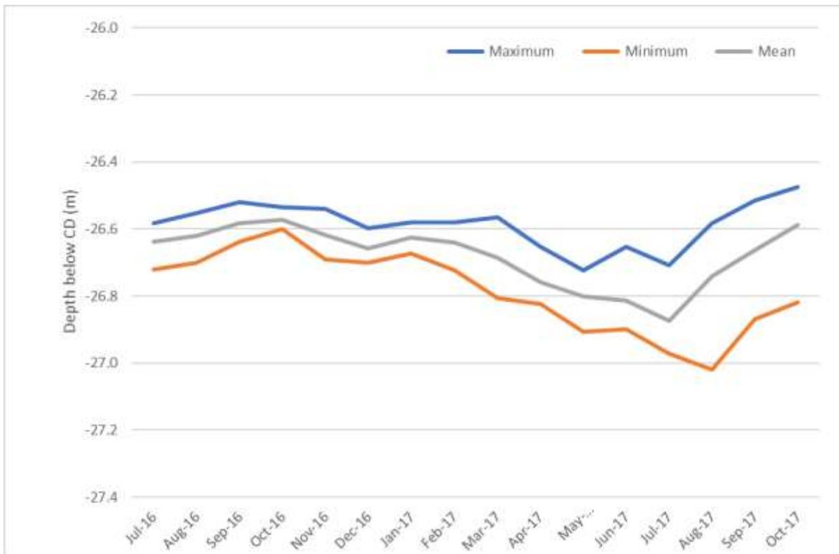
Figure 8. Figure 4.1: SE Beam 2 Scour Depth
