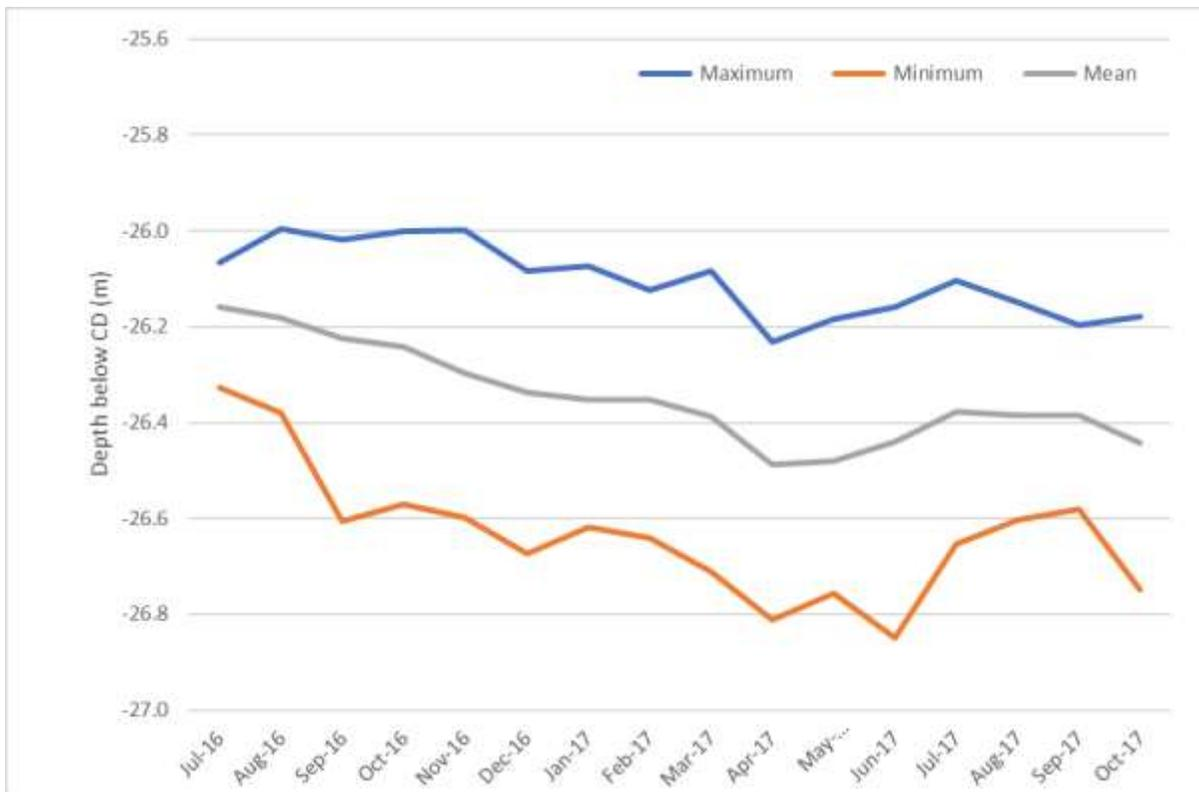
Figure 14. NE Beam 4 Scour Depth
