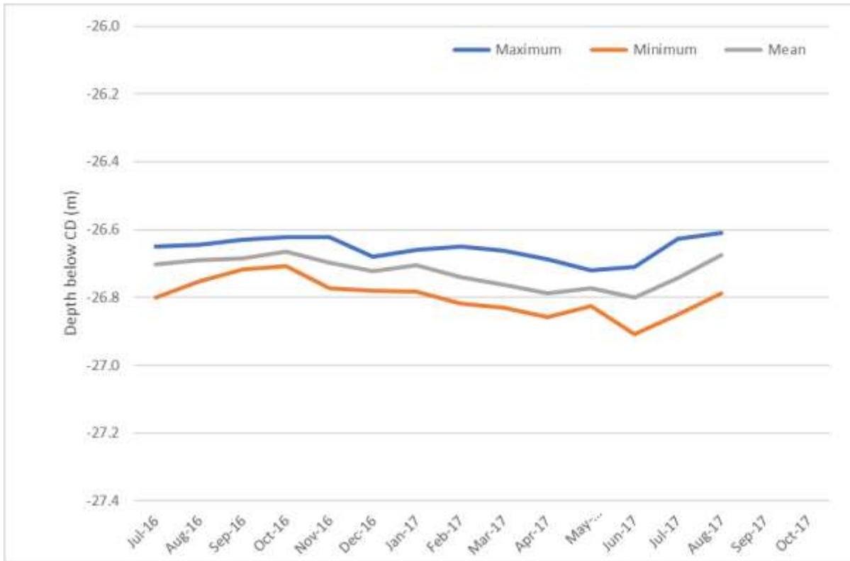
Figure 9. SE Beam 3 Scour Depth
