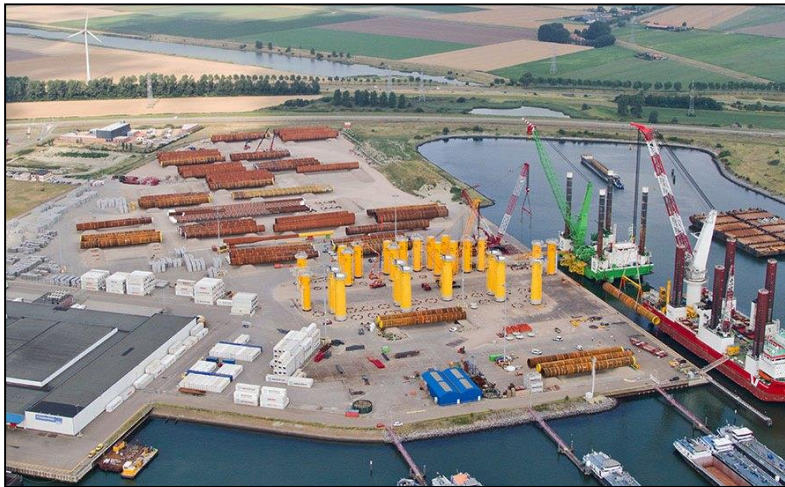
Figure 4-1. BOW Terminal handling foundations (BOW Terminal 2014, Renewables 2014)
