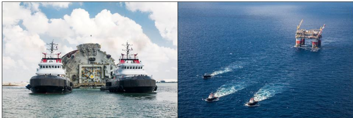
Figure 3-8. Spar (left panel) and Semi-Sub (right panel) towed by two Crowley Ocean Tugs (150-ton bollard pull each), with a support tug as auxiliary (Crowley 2013)
