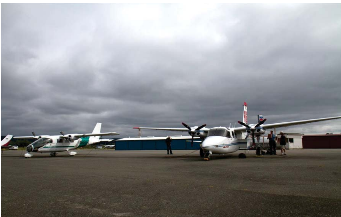
Figure 2. Survey aircraft used during the PaCSEA program. Partenavia P-68 Observer (left; Aspen Helicopters, Oxnard, CA) and Commander AC-500 (right; GoldAero, Arlington, WA). Photo by J. Felis, USGS.
