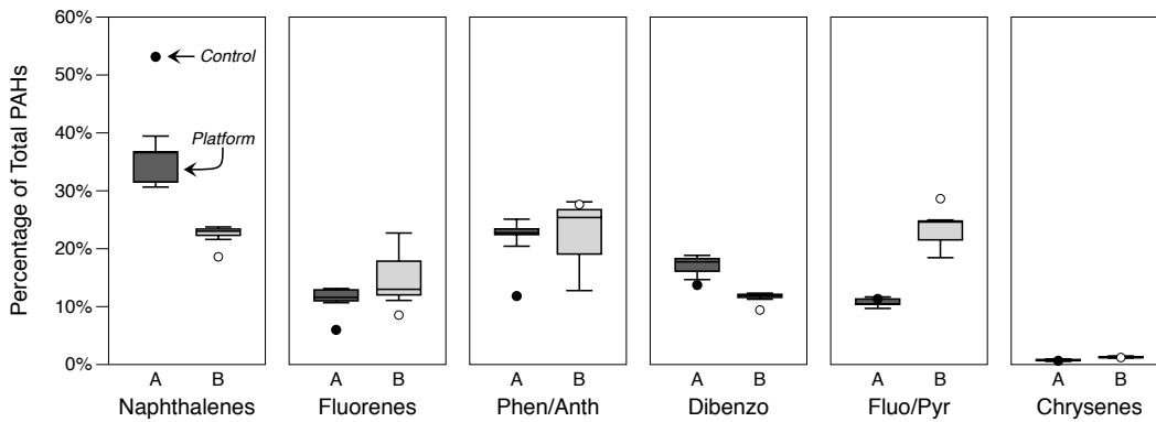
Figure 3.3. Percentage contributions of PAH compound groups to total PAHs at Platforms A and B sites. Each box plot shows the spread in the data with the range (lines above and below boxes), median (lines through boxes) and the 25% and 75% quartiles (the lower and upper boundaries of the boxes) of these data. Associated controls are shown as points.
