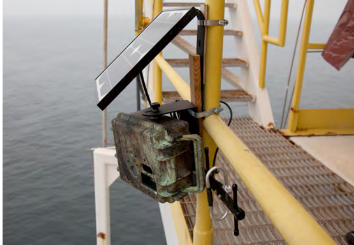
Figures A-3: Close-up image of BirdCam showing the camera unit in green camouflage box, solar panel and antenna. Note simple attachment to vertical handrail support with hose-clamps and wooden shim.]
