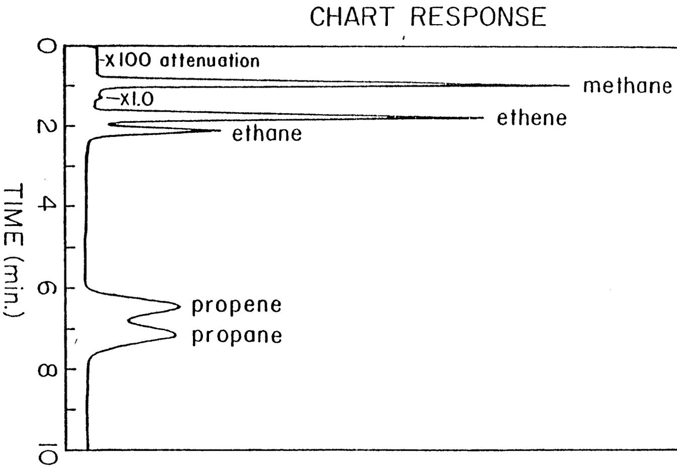
Figure 3.3 Chromatogram of Sediment Light Hydrocarbons.
